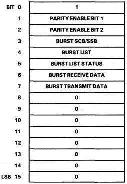
FIGURE 4-31. INITIALIZATION OPTIONS BIT ASSIGNMENTS
