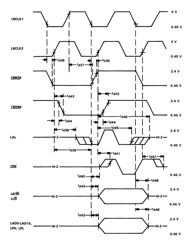
NOTE 10: The timing reference points for LBCLK1 and LBCLK2 are 3 V and 0.8 V. The timing reference points for the other waveforms are 2 V and 0.8 V.
