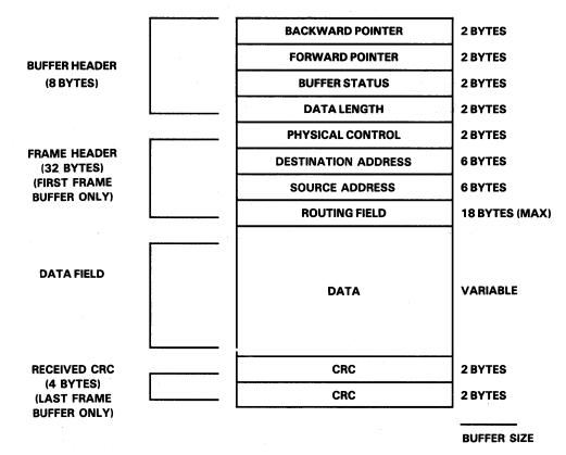
FIGURE 4-43. ADAPTER INTERNAL BUFFER FORMAT
