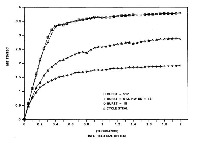
FIGURE 2-10. TRANSMIT THROUGHPUT – PC AT ADAPTER: DMA MODE COMPARISON – 512 BYTE BUFFERS
