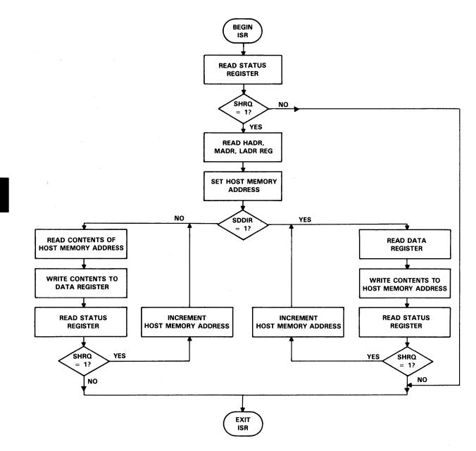
FIGURE 2-2. INTERRUPT SERVICE ROUTINE FLOWCHART - I/O MAPPED EXAMPLE
