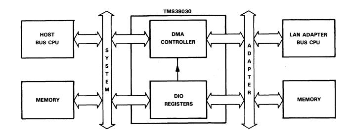
FIGURE 1. TMS38030 DMA CONTROL-CONCEPTUAL REPRESENTATION
