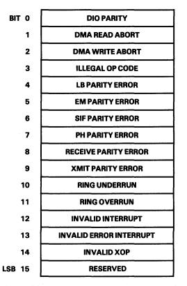
FIGURE 4-38. ADAPTER CHECK STATUS FORMAT
