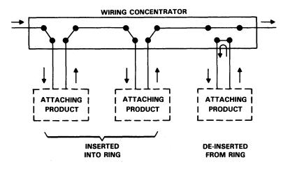
FIGURE 1-5. TOKEN RING WIRING CONCENTRATOR
