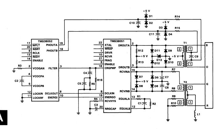
FIGURE 1. TOKEN RING INTERFACE CIRCUIT
