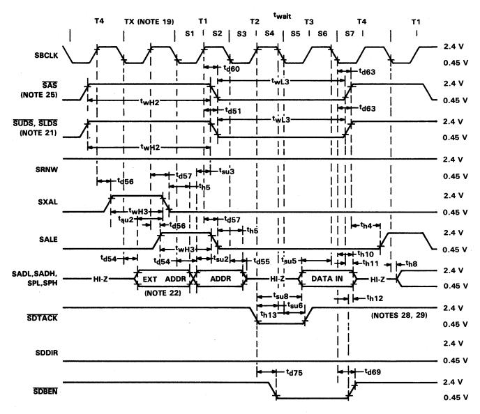
NOTES: 19. In cycle-steal mode, state TX is present on every system bus transfer. In burst mode, state TX is present on the first bus transfer, and whenever the increment of the address carries beyond the least-significant 8 bits.
