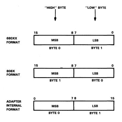
FIGURE 4-13. BIT- AND BYTE-NUMBERING CONVENTIONS
