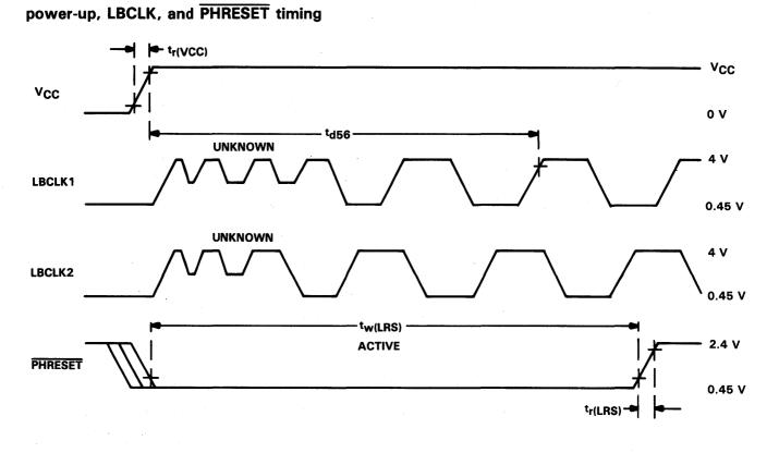
NOTE 11: The timing reference points for V<sub>CC</sub> are 4.5 V and 1.2 V. The timing reference points for LBCLK1 and LBCLK2 are 3 V and 0.8 V. The timing reference points for PHRESET are 2 V and 0.8 V.
