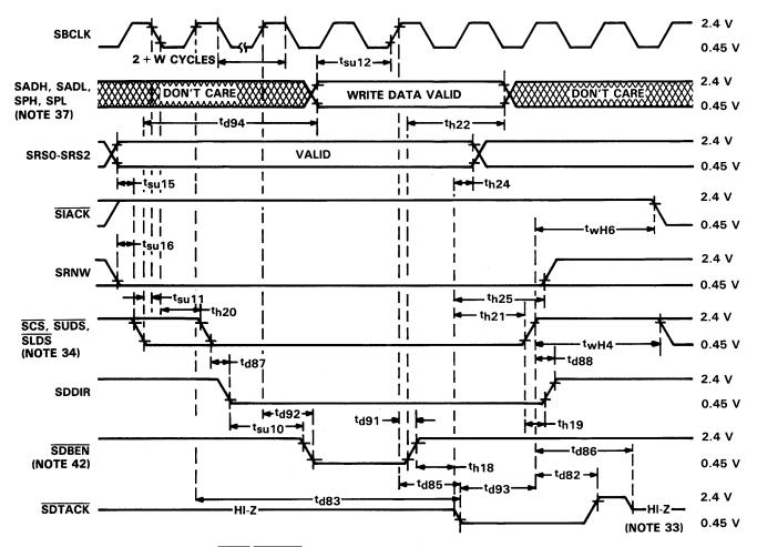
NOTES: 33. Internal logic will drive SRDY/SDTACK high and verify that it has reached a valid high level before tristating the signal.
