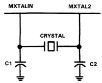
NOTE 7: C1 and C2 represent the total capacitance on these pins including strays and parasitics, but not the input capacitance of the device pins.
