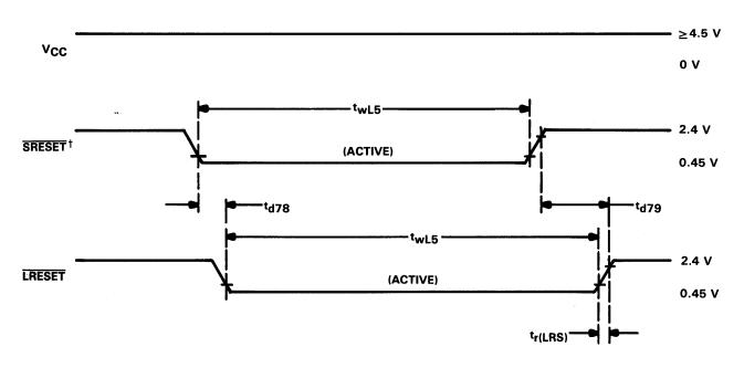
NOTE 18: The timing reference points for SRESET and LRESET are 2 V and 0.8 V. <sup>†</sup>Following a low-to-high transition of SRESET, SRESET must remain high for a minimum of 20 milliseconds before again driven low.
