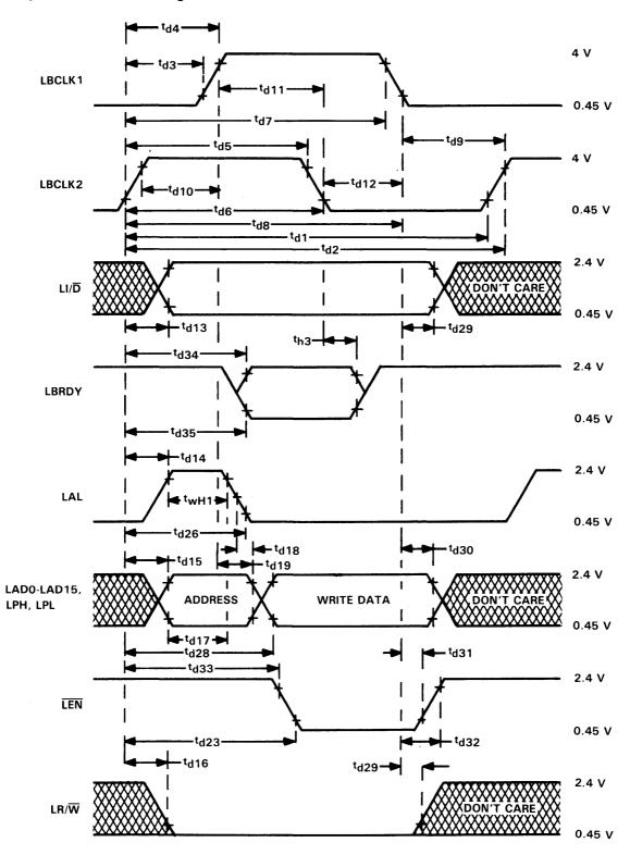
NOTE 9: The timing reference points for LBCLK1 and LBCLK2 are 3 V and 0.8 V. The timing reference points for the other waveforms are 2 V and 0.8 V. The intermediate reference point for LAL is 1.3 V.
