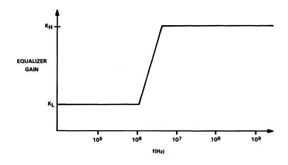
FIGURE 4-71. EQUALIZER TRANSFER FUNCTION
