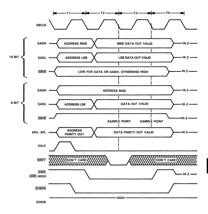
FIGURE 4-21. 808X DMA WRITE CYCLE TIMING
