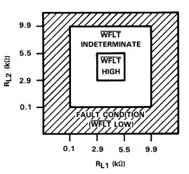
FIGURE 4. WIRE-FAULT PIN TEST
