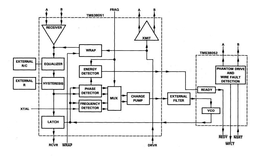
FIGURE 4-68. RING INTERFACE FUNCTIONAL BLOCK DIAGRAM
