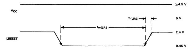
NOTE 16: The timing reference points are 2 V and 0.8 V.
