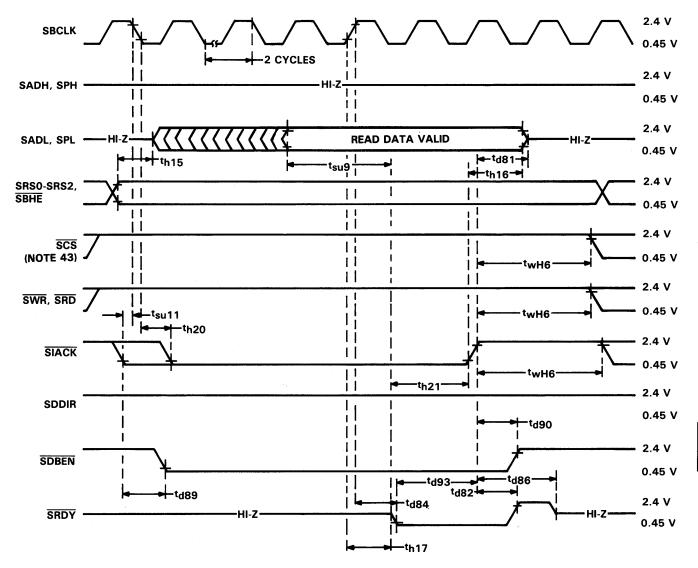
NOTE 43: The "inactive" chip select is SIACK in DIO read and DIO write cycles, and SCS in interrupt acknowledge cycles.
