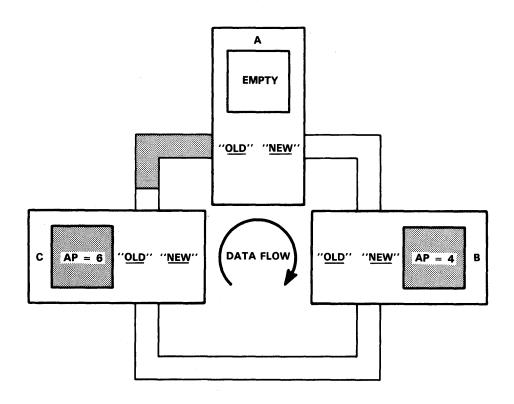
FIGURE 3-25. STATION A STRIPS FRAME FROM THE RING
