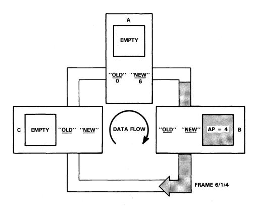
FIGURE 3-29. FRAME CIRCULATES WITH NO MODIFICATION
