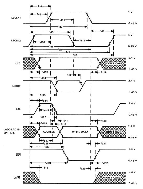
NOTE 8: The timing reference points for LBCLK1 and LBCLK2 are 3 V and 0.8 V. The timing reference points for the other waveforms are 2 V and 0.8 V. The intermediate reference point for LAL is 1.3 V.
