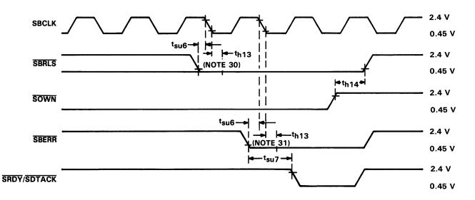
NOTES: 30. The TMS38030 ignores the assertion of SBRLS if it does not own the system bus. If it does own the system bus, then when it detects the assertion of SBRLS it will complete any internally started DMA cycle and relinquish control of the bus. If no DMA transfer has internally started, then the TMS38030 will release the bus before starting another.
