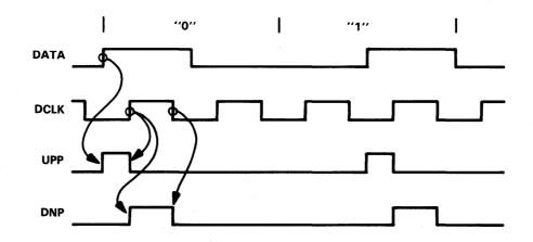
FIGURE 4-74. PHASE DETECTOR TIMING CHARACTERISTICS
