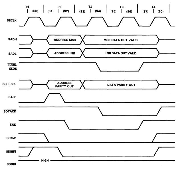
FIGURE 4-25. 680XX MODE DMA WRITE TIMING
