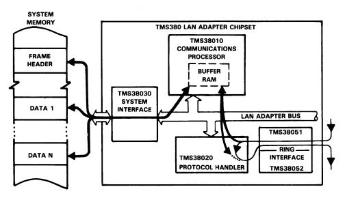
FIGURE 1-11. ADAPTER DATA FLOW
