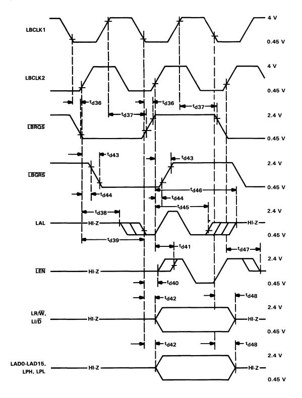
NOTE 9: The timing reference points for LBCLK1 and LBCLK2 are 3 V and 0.8 V. The timing reference points for the other waveforms are 2 V and 0.8 V.
