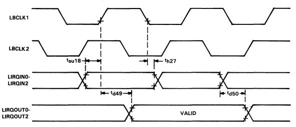
NOTE 10: LIRQOUTs may not follow LIRQINs because the TMS38030 prioritizes LIRQOUT0-LIRQOUT2 outputs between internal TMS38030 interrupts and LIRQIN0-LIRQIN2.
