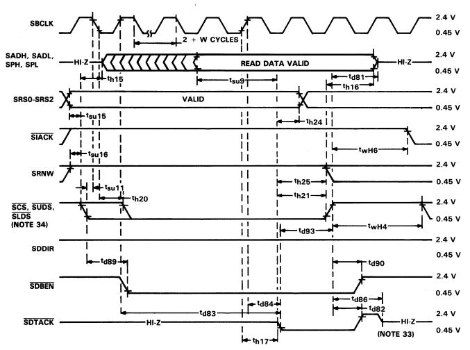
NOTES: 33. Internal logic will drive SRDY/SDTACK high and verify that it has reached a valid high level before tristating the signal.
