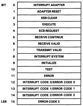
NOTE: Bits 12 through 15 are used to report bring-up diagnostic and initialization errors.
