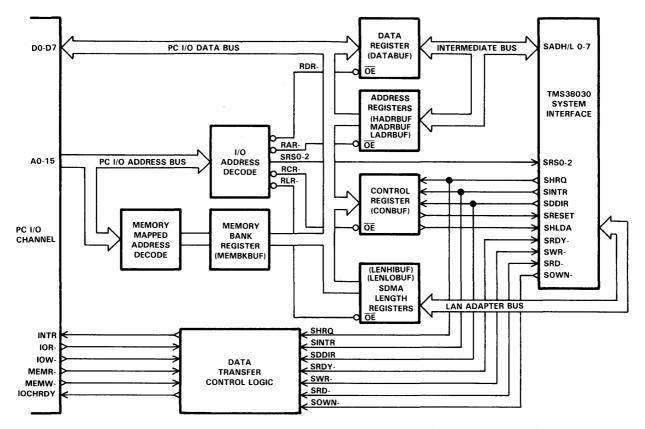
FIGURE 2-3. MEMORY MAPPED DESIGN BLOCK DIAGRAM
