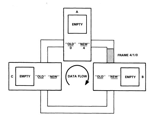
FIGURE 3-34. STATION B STRIPS ITS FRAME FROM THE RING
