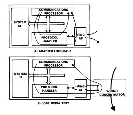
FIGURE 1-10. ADAPTER SELF-TEST
