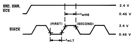
808X mode interrupt acknowledge timing-second SIACK pulse
