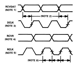
NOTES: 1. Output of the receiver (internal signal derived from RCVIN pins) 2. PLL Static timing offset plus 62.5 ns
