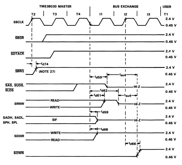
NOTE 27: In 808X Mode, the TMS38030 deasserts SHRQ on the rising edge of SBCLK following the T4 state of the last system bus transfer it controls. In 680XX Mode, the TMS38030 deasserts SBRQ on the rising edge of SBCLK in state T2 of the first system bus transfer it controls.
