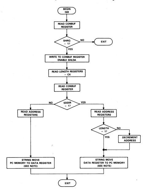
NOTE: The string move instruction automatically increments the source and destination addresses for each byte until the CX register is decremented to zero.
