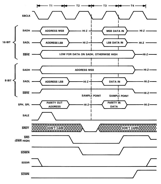
FIGURE 4-20. 808X DMA READ CYCLE TIMING
