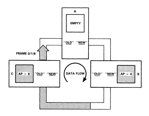
FIGURE 3-24. STATION C REPEATS FRAME AND CHANGES PR TO 6.
