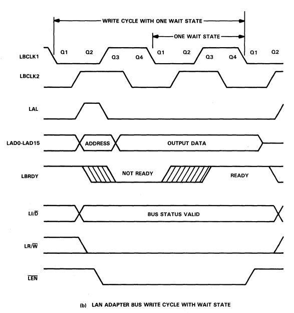
FIGURE 4-7. LAN ADAPTER BUS TRANSFERS WITH ONE WAIT STATE (concluded)
