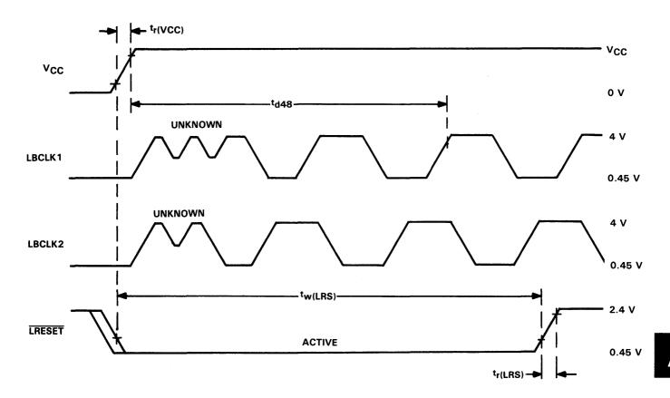
NOTE 17: The timing reference points for V<sub>CC</sub> are 4.5 V and 1.2 V. The timing reference points for LBCLK1 and LBCLK2 are 3 V and 0.8 V. The timing reference points for LRESET are 2 V and 0.8 V.
