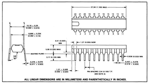
NOTE A: Each pin centerline is located within 0,25(0.010) of its true longitudinal position.
