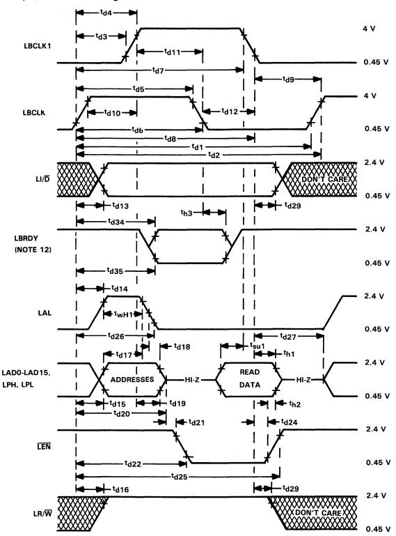
NOTES: 11. The timing reference points for LBCLK1 and LBCLK2 are 3 V and 0.8 V. The timing reference points for the other waveforms are 2 V and 0.8 V. The intermediate reference point for LAL is 1.3 V.
