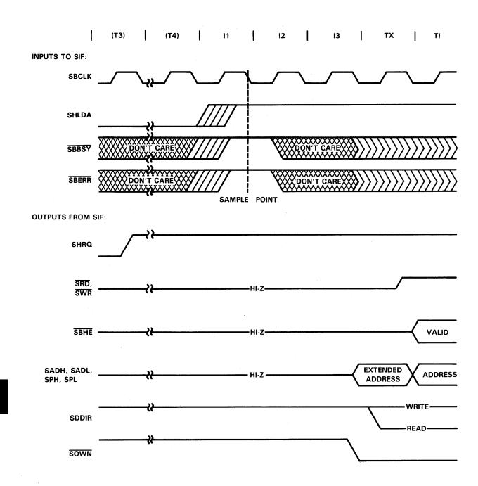
FIGURE 4-18. ADAPTER ACQUIRES SYSTEM BUS - 808X MODE
