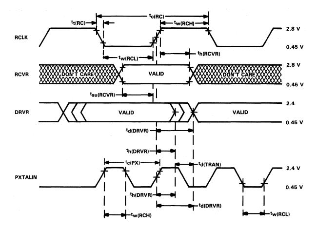
NOTE 19: The timing reference points for RCVR and RCLK are 2.6 V and 0.6 V. The timing reference points for PXTALIN are 2 V and 0.8 V. The intermediate reference point for RCLK and DRVR is 1.5 V.
