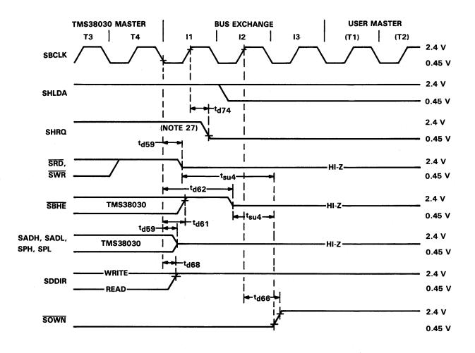
NOTE 27: In 808X Mode, the TMS38030 deasserts SHRQ on the rising edge of SBCLK following the T4 state of the last system bus transfer it controls. In 680XX Mode, the TMS38030 deasserts SBRQ on the rising edge of SBCLK in state T2 of the first system bus transfer it controls.
