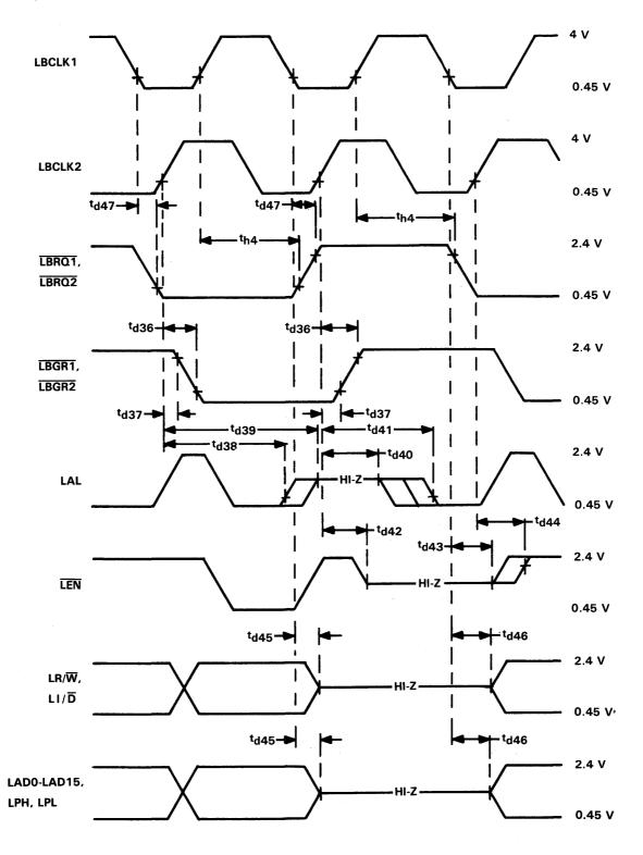
NOTE 13: The timing reference points for LBCLK1 and LBCLK2 are 3 V and 0.8 V. The timing reference points for the other waveforms are 2 V and 0.8 V.
