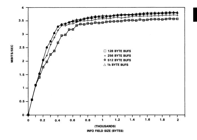
FIGURE 2-7. TRANSMIT THROUGHPUT — PC AT ADAPTER: INTERNAL BUFFER SIZE COMPARISON
