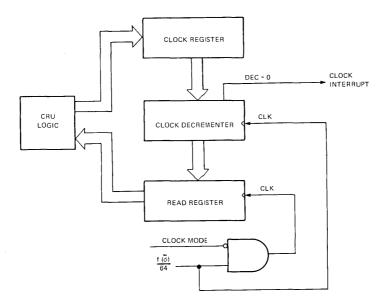
FIGURE 6-TMS 9901 INTERVAL TIMER SECTION
