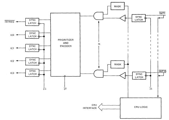
FIGURE 3- TMS 9901 PSI INTERRUPT CONTROL SECTION BLOCK DIAGRAM
