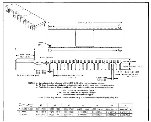
ceramic packages with side-brazed leads and metal or epoxy or glass lid seal
