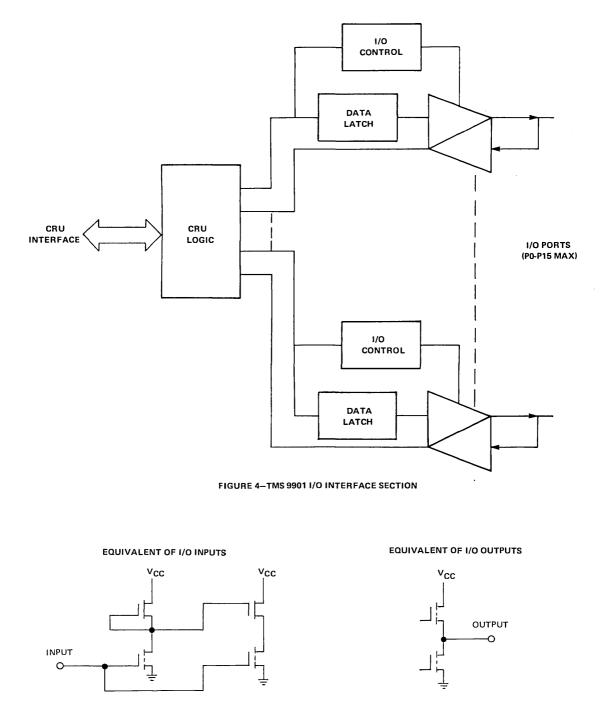
FIGURE 5 - INPUT AND OUTPUT EQUIVALENTS
