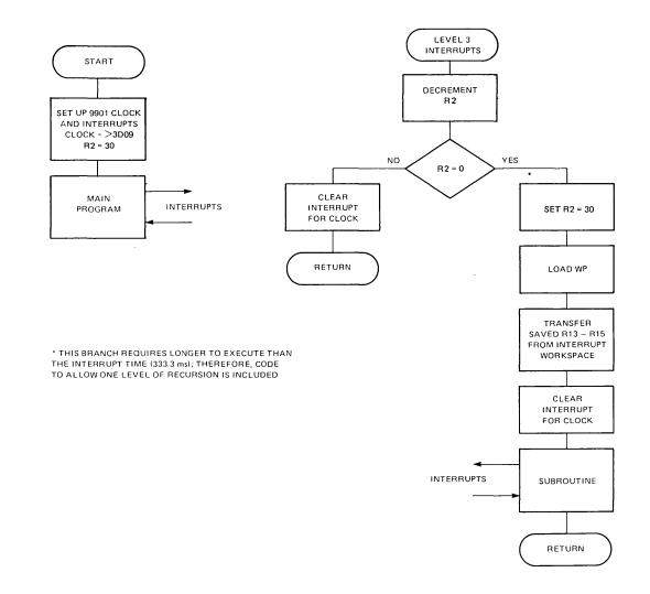
FIGURE 10-TMS 9901 INTERVAL TIMER APPLICATION FLOWCHART
