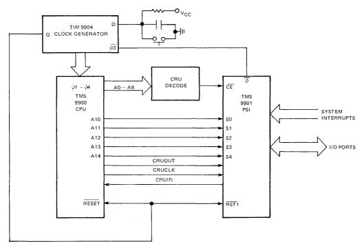
FIGURE 7-TMS 9900/TMS 9901 INTERFACE
