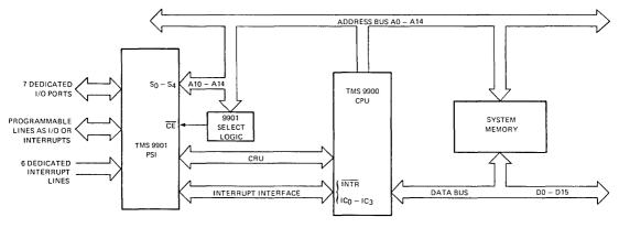
FIGURE 1- TYPICAL TMS 9901 PROGRAMMABLE SYSTEM INTERFACE (PSI) APPLICATION
