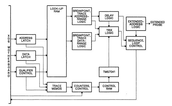
Figure 11-12. Breakpoint/Trace/Timing Card Block Diagram
