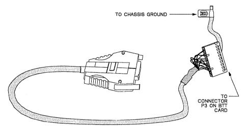
Figure 11-15. Extended-Address Cable
