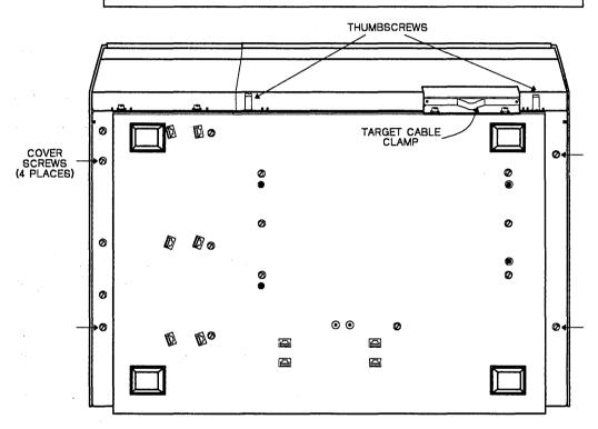
Figure 11-21. Top Cover Removal
