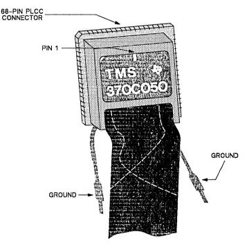
Figure 11-18. TMS370C050 Target Cable Assembly
