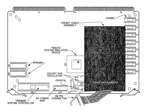
Figure 11-8. TMS370 Emulator Board with Target Cable Attached
