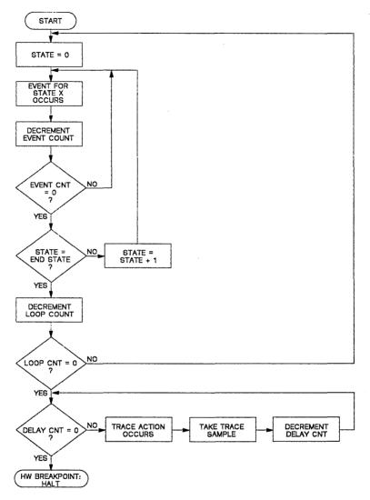
Figure 8-2. Flow of BTT Operation
