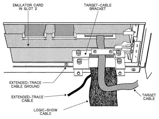
Figure 11-10. XDS/22 with Breakpoint/Trace and Emulator Cards Installed
