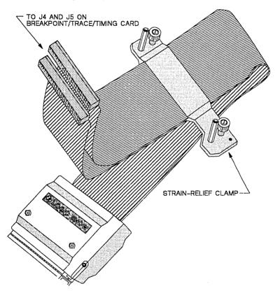
Figure 11-13. Texas Instruments LOGIC-SHOW Cable
