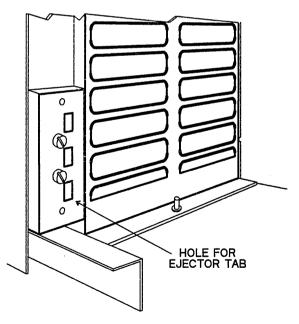
Figure 11-17. XDS/22 Card Cage Ejector Tab Holes
