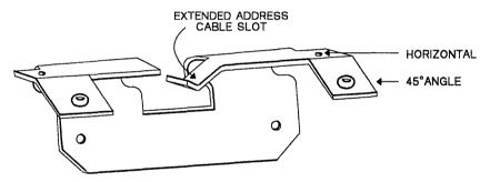
Figure 11-5. Chassis Cable Mounting
