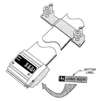
Figure 11-14. LOGIC-SHOW Cable Showing Pinout Label
