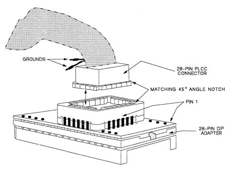
Figure 11-19. TMS370C010 Target Cable Assembly
