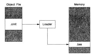
Figure 9-13. RAM Model of Autoinitialization
