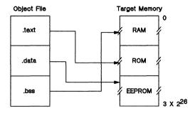
Figure 3-1. Partitioning Memory into Logical Blocks
