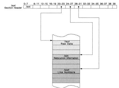
Figure A-3 illustrates how the pointers in a section header would point to the various elements in an object file that are associated with the .text section.
