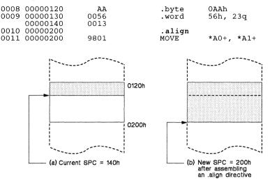
Figure 5-6. An Example of the .align Directive
