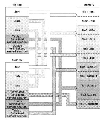
Figure 3-5. Combining Input Sections from Two Files (Default Allocation)
