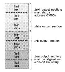
Figure 9-7. Section Allocation Defined by Figure 9-6
