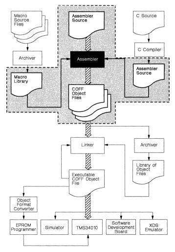
Figure 4-1. Assembler Development Flow
