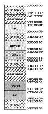
Figure 3-8. Placing the Code from Figure 3-4 into the Memory Map Defined by Figure 3-6
