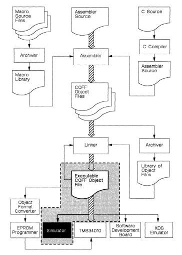
Figure 11-1. Simulator Development Flow
