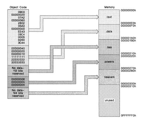
Figure 3-4. Default Allocation of the Object Code from Figure 3-2
