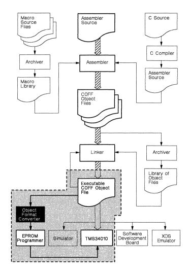
Figure 10-1. Object Format Converter Development Flow
