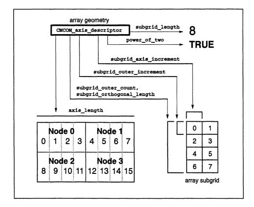
Figure 23. The CMCOM\_axis\_descriptor data structure.
