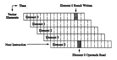
For example, assuming a four-element vector length, the pipeline pattern is:
