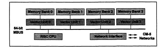
Figure 4. A typical CM-5 processing node, showing the location of the 4 VUs.
