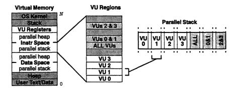
The VU control and data registers for each VU combination are mapped together into a single region:
