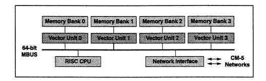
Figure 2. A typical CM-5 processing node.
