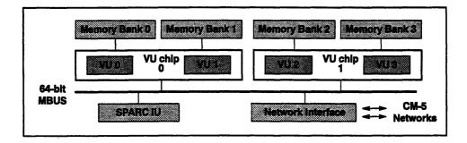
Figure 5. Internal arrangement of VU chips in CM-5 processing node.
