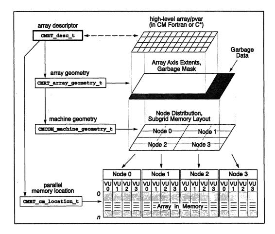
Figure 18. Internal Structure of a CM Array.
