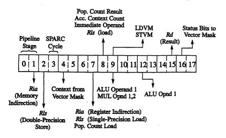
A new vector element is started at each VU pipeline stage. Thus, the result of the operation for element 0 is not generally available until four operations later.
