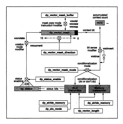
Figure 10. Effects of VU control registers on ALU and memory instructions.
