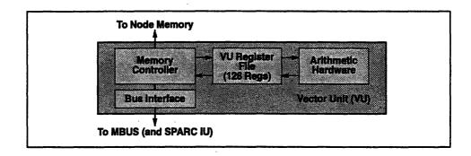
Figure 8. VU internal components.
