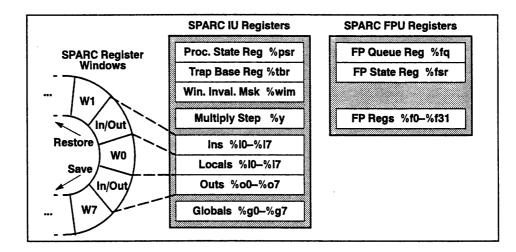
Figure 12. SPARC CPU registers accessible from DPEAC.
