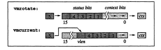
Figure 11. Bit-shifting modes of vector mask register.
