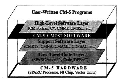
Figure 3. Structure of software layers on the CM-5.
