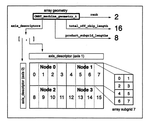
Figure 22. The CMCOM\_machine\_geometry data structure.
