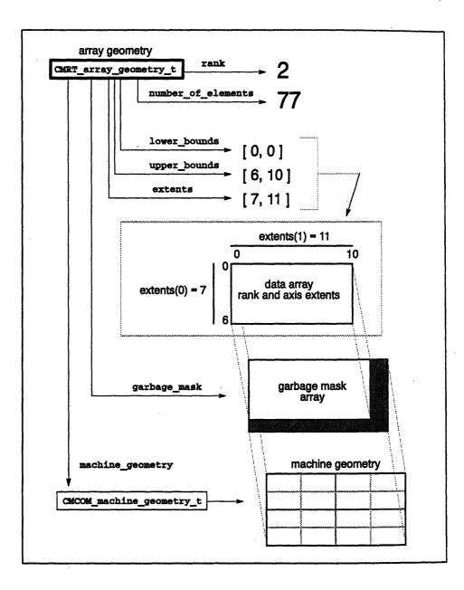
Figure 21. The CMRT\_array\_geometry data structure.
