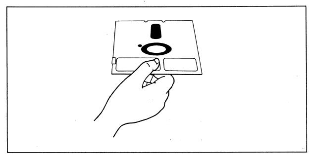
Figure 5-4 Holding Diskette Before Insertion
