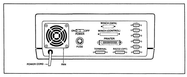
Figure 2-3 Rear Panel of the TS 806/20
