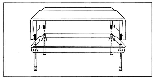
Figure 2-4 Location of Screws in the TS 806/20 Case
