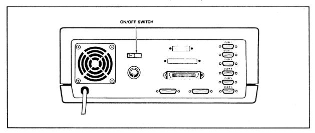
Figure 3-1 On/Off Switch on Rear Panel
