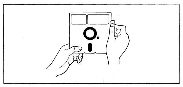
Figure 5-3 Write-Protecting Diskette
