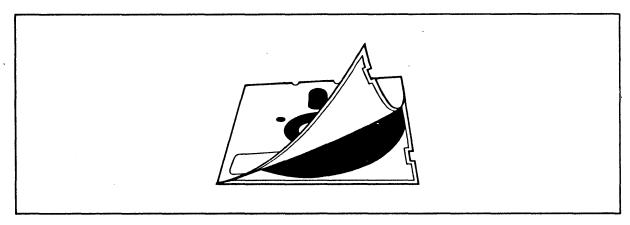
Figure 5-7 Diskette and Protective Lining Inside the Protective Black Plastic Enclosure
