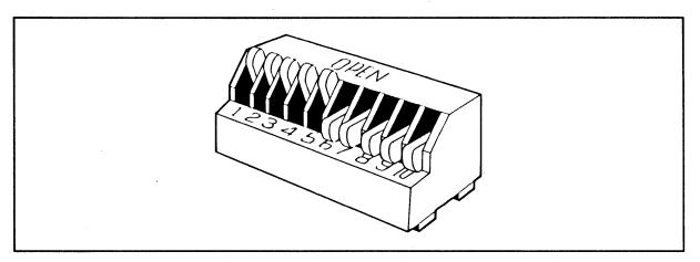
Figure 2-6 Dipswitches 1 through 5 Open; 6 through 10 Closed
