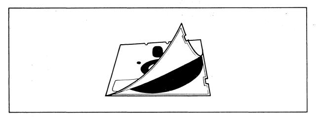
Figure 1-4 Diskette Inside Permanent Plastic Enclosure
