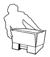
4. Holding the box firmly, gently turn it upside down. Lift the box off the TS 806/20.
