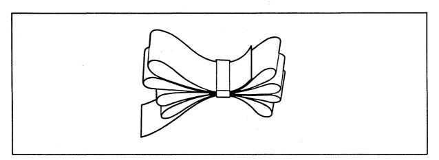
Figure 2-2 Correctly-Folded Excess Ribbon Cable
