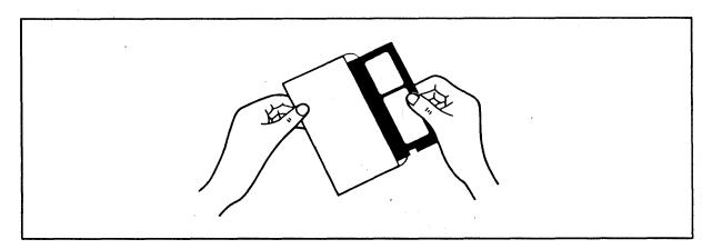
Figure 5-2 Removing Diskette from Jacket
