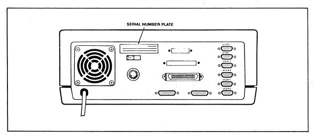
Figure 7-4 Location of Serial Number on Rear Panel
