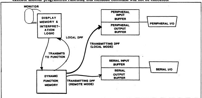
Figure 5-12: Dynamic Programmable Functions
