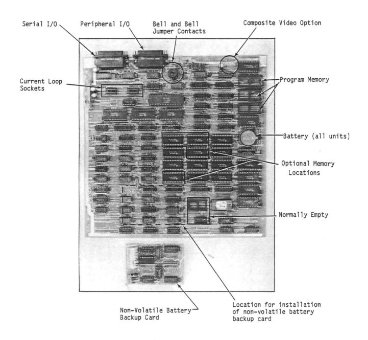
Figure 2-1: Logic Module
