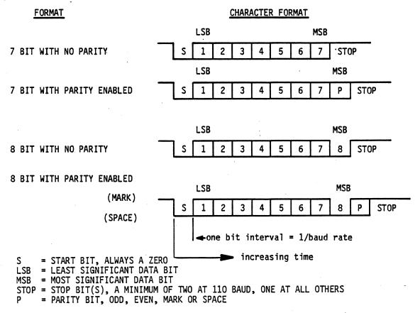
Figure 5-5 - Asynchronous Character Format
