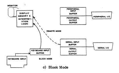
Figure 5-6: Data Flow Controls
