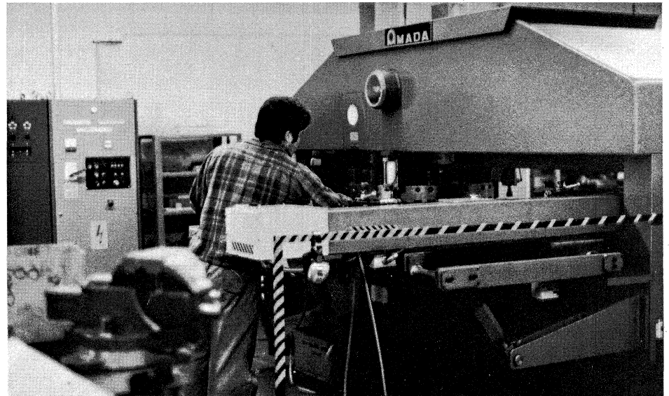
Machine operator mounts the sheet metal "blanks" and clamps them. The rest is automatic. (Photos courtesy of Prime Metals.)
