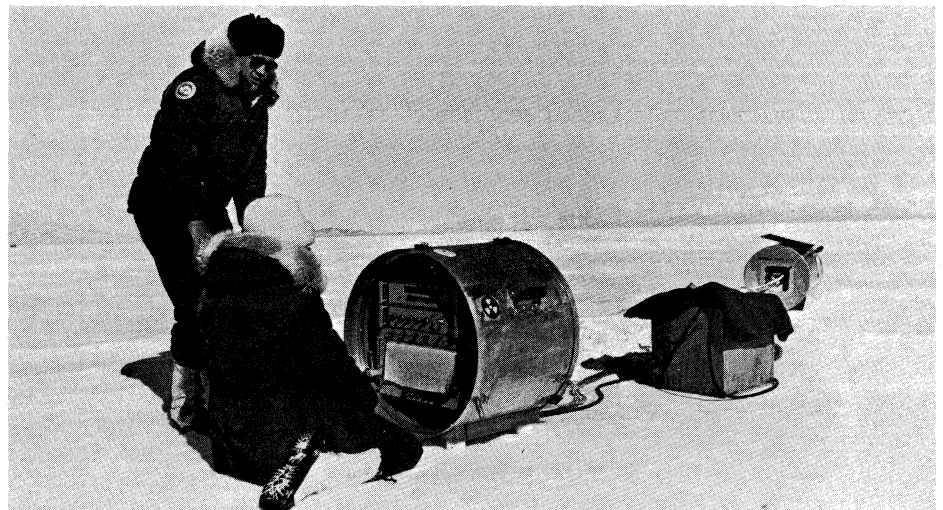
The gamma ray detector and analog recorder shown will be loaded into a helicopter and flown over Antarctic mountain peaks to gather data on potential uranium and thorium resources.
