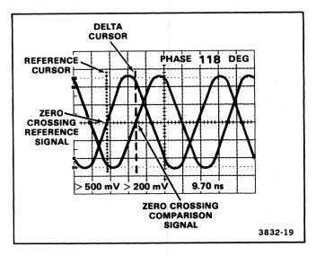
Figure 6-7. Phase difference between two time-related signals.
