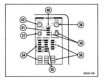
Figure 3-5. Trigger controls and indicators.
