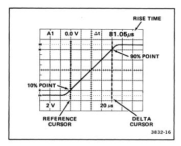
Figure 6-4. Measuring rise times.
