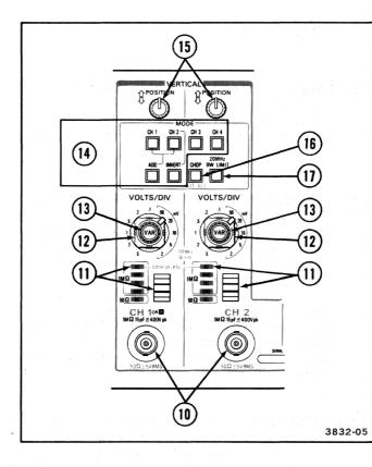
Figure 3-2. Vertical controls and CH 1 OR X and CH 2 connectors.
