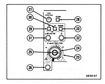
Figure 3-4. Horizontal and delta measurement controls.
