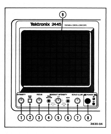
Figure 3-1. Power and display controls.
