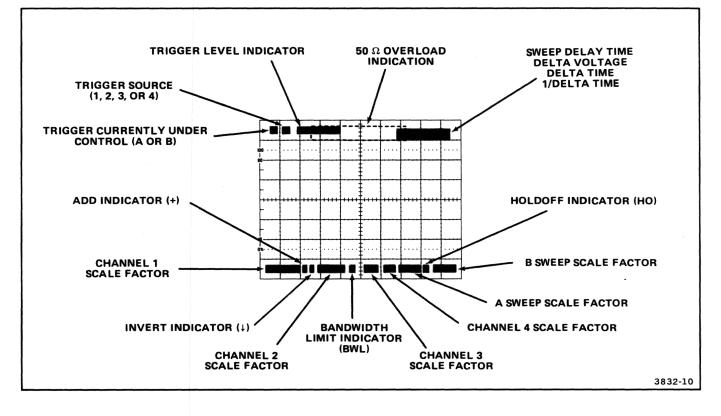
Figure 3-7. Readout display locations.
