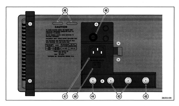
Figure 3-6. Rear-panel controls and connectors.
