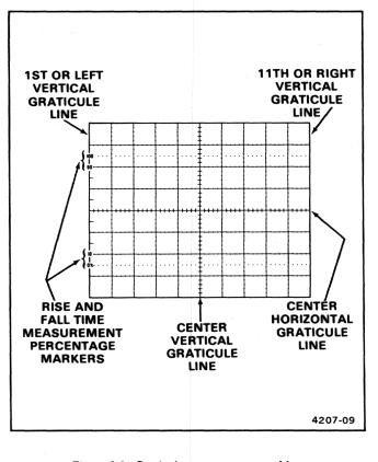
Figure 4-1. Graticule measurement markings.
