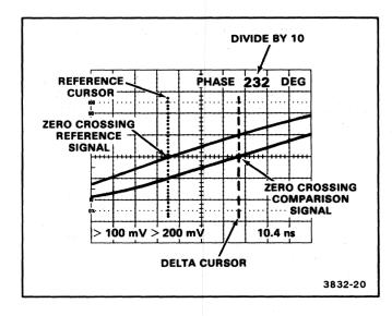
Figure 6-8. Small-angle phase difference.
