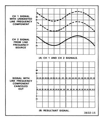
Figure 6-3. Eliminating common-mode signals.
