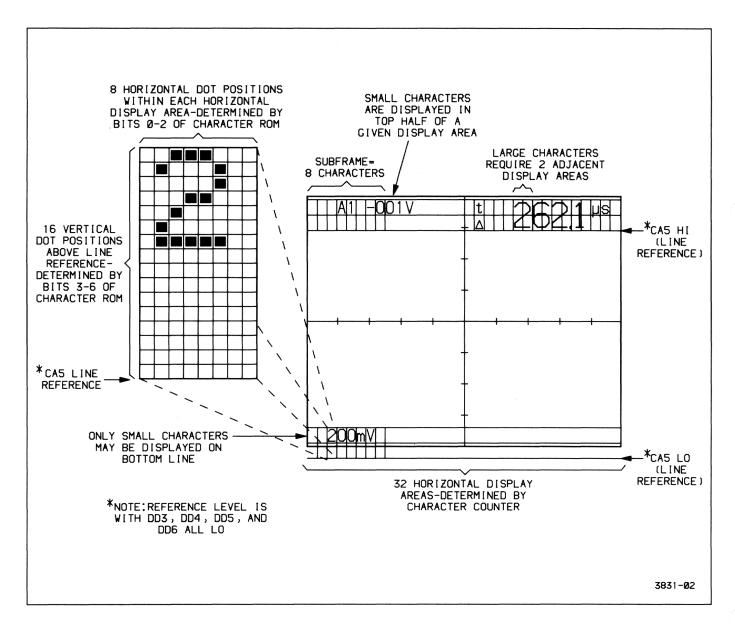
Figure 3-7. Developing the readout display.
