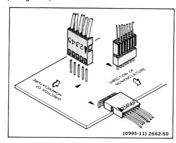
Figure 6-1. Multipin connector orientation.
