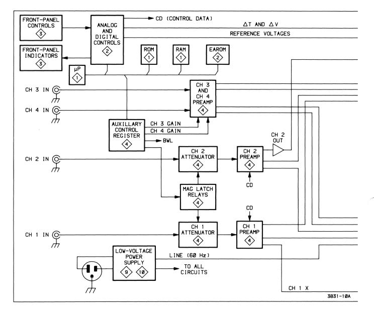
Figure 3-1. Block diagram.
