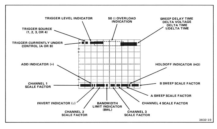
Figure 2-8. Readout display locations
