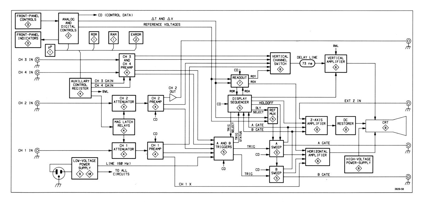
Figure 9-4. 2445 block diagram.
