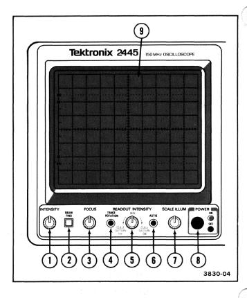
Figure 2-2. Power and display controls.
