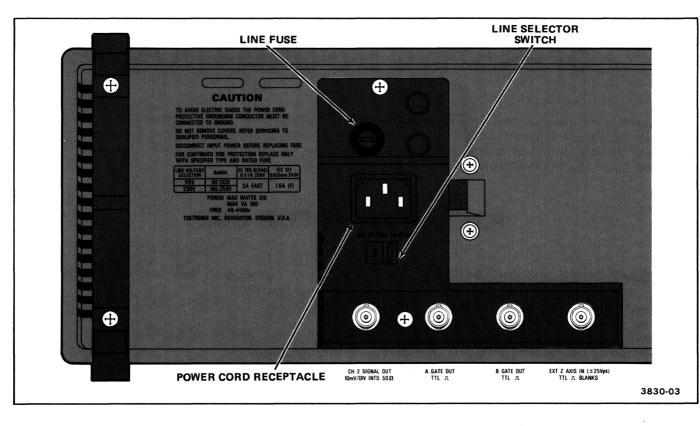
Figure 2-1. Line selector switch, line fuse, and detachable power cord.
