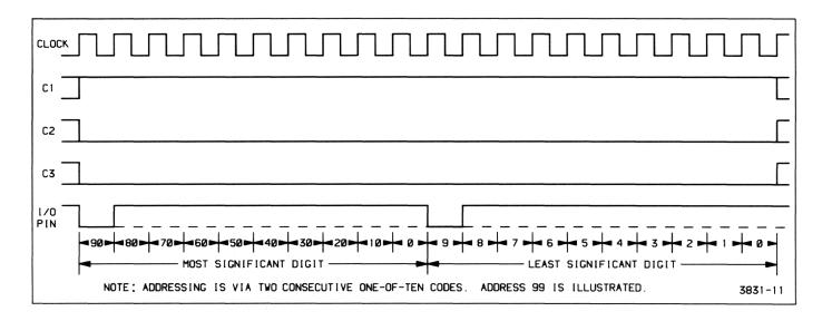
Figure 3-3. Accept address timing.
