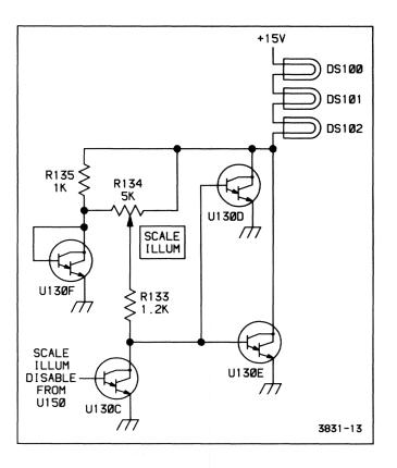
Figure 3-5. Scale Illumination circuit.
