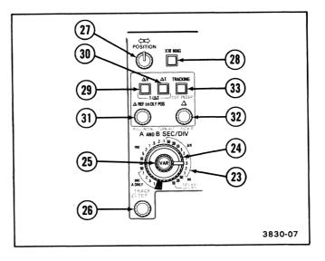
Figure 2-5. Horizontal and delta measurement controls.
