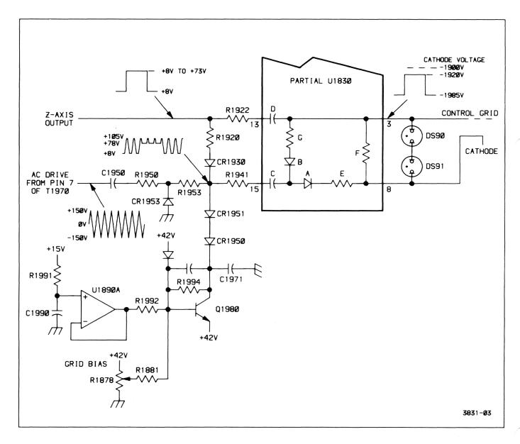
Figure 3-10. Dc Restorer circuit.
