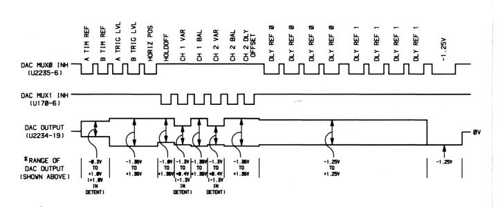
\*NOTE AS ANY GIVEN CONTROL IS EXERCISED, THE CORRESPONDING PORTION OF THE DAC OUTPUT WAVEFORM SHOULD VARY WITHIN THE LIMITS INDICATED.
