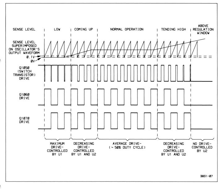
Figure 3-11. Timing relationships of the Inverter Drive signals.
