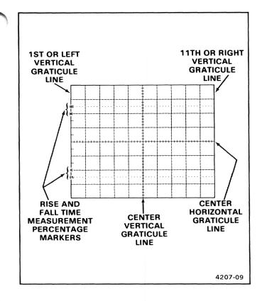
Figure 2-9. Graticule measurement markings.
