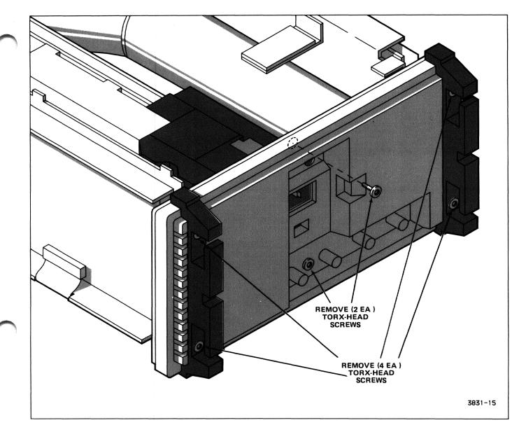
Figure 6-2. Rear panel removal.
