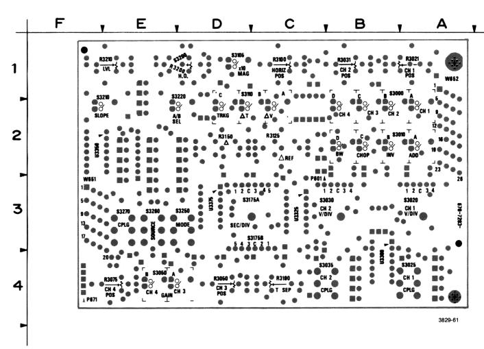
Figure 9-7. Circuit view of A6—Front Panel.
