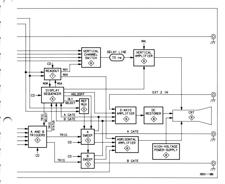
Figure 3-1. Block diagram (cont).
