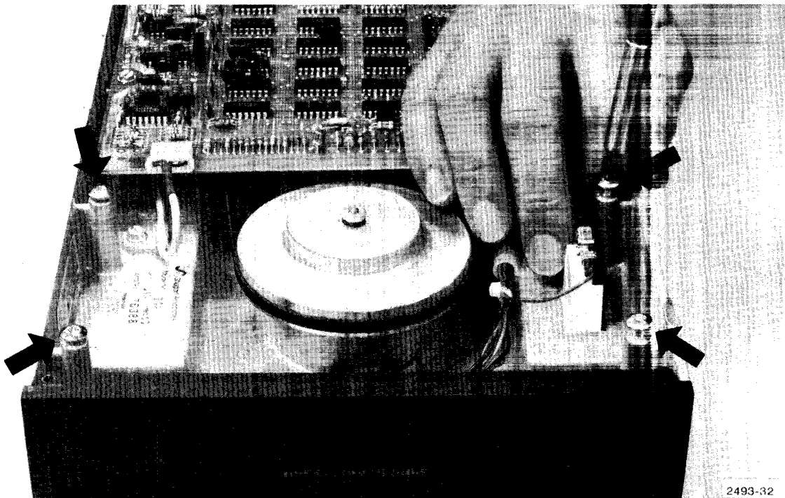
Figure 7-6. Removing screws from kit drive chassis.
