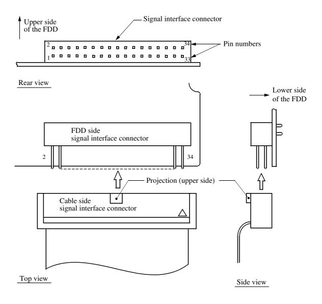
(Fig. 8.1-1) Signal interface connector external view
