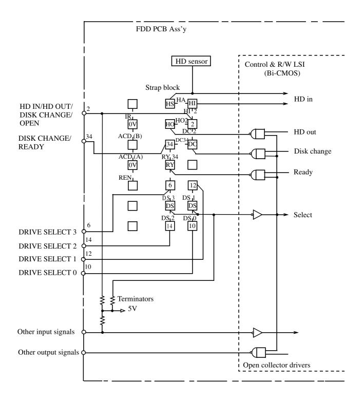
(Fig. 8.2-1) FDD signal interface circuit
