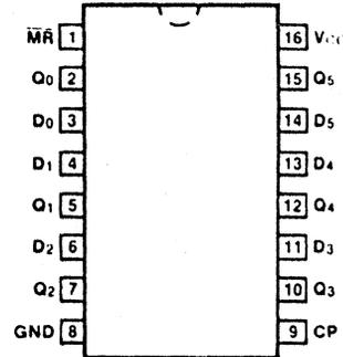
**DESCRIPTION** — The '174 is a high speed hex D flip-flop. The device is used primarily as a 6-bit edge-triggered storage register. The information on the D inputs is transferred to storage during the LOW-to-HIGH clock transition. The device has a Master Reset to simultaneously clear all flip-flops.
