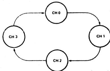
If the ROTATING PRIORITY bit is not set (set to a zero), each DMA channel has a fixed priority. In the fixed priority mode, Channel 0 has the highest priority and Channel 3 has the lowest priority. If the ROTATING PRIORITY bit is set to a one, the priority of each channel changes after each DMA cycle (not each DMA request). Each channel moves up to the next highest priority assignment, while the channel which has just been serviced moves to the lowest priority assignment:
