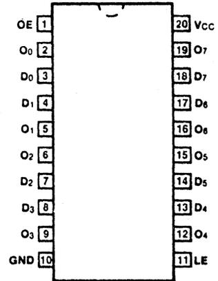
**DESCRIPTION** — The '373 consists of eight latches with 3-state outputs for bus organized system applications. The flip-flops appear transparent to the data when Latch Enable (LE) is HIGH. When LE is LOW, the data that meets the setup times is latched. Data appears on the bus when the Output Enable ( $\overline{OE}$ ) is LOW. When  $\overline{OE}$  is HIGH the bus output is in the high impedance state.
