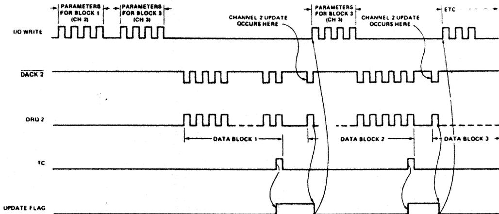
Figure 5. Autoload Timing
