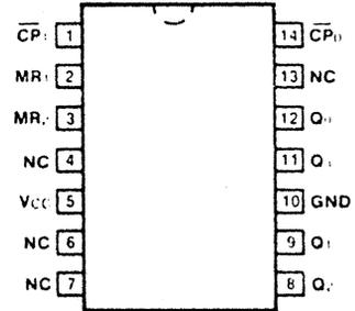
**DESCRIPTION** — The '93 is a 4-stage ripple counter containing a high speed flip-flop acting as a divide-by-two and three flip-flops connected as a divide-by-eight. HIGH signals on the Master Reset (MR) inputs override the clocks and force all outputs to the LOW state.
