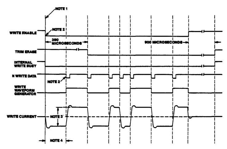
NOTES: 1. t = 0 = 250 MILLISECONDS AFTER DRIVE MOTOR STARTS OR 20 MILLISECONDS AFTER LAST STEP PULSE, WHICHEVER IS THE LATEST TIME.
