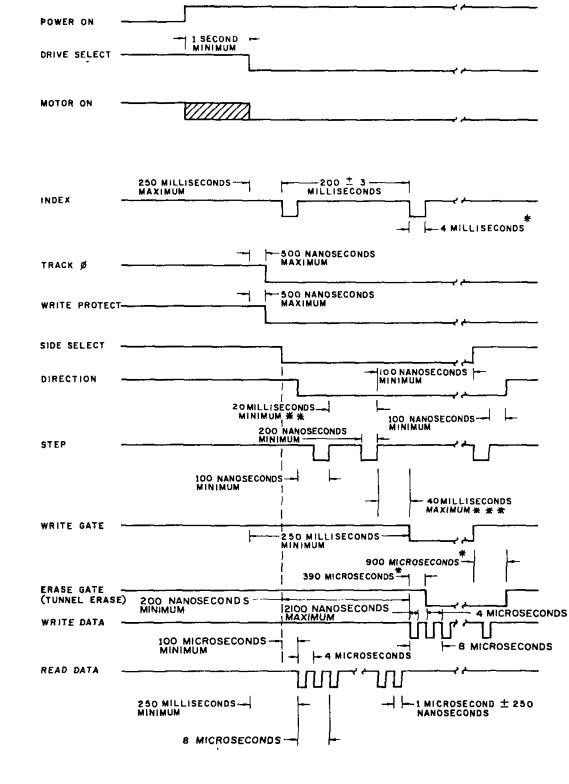
NOTES: \* FOR REFERENCE ONLY \*\* 6 MILLISECONDS FOR FAST STEP MOTOR (OPTIONAL) \*\*\* 21 MILLISECONDS FOR FAST STEP MOTOR (OPTIONAL)
