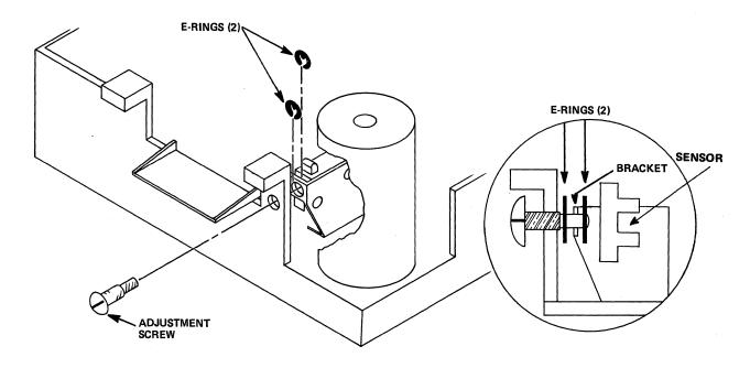
Figure 5-21 Track 00 Sensor Assembly E-Rings and Adjustment Screw
