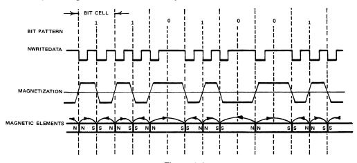
Figure 1-3 FM Recording Magnetization Profiles
