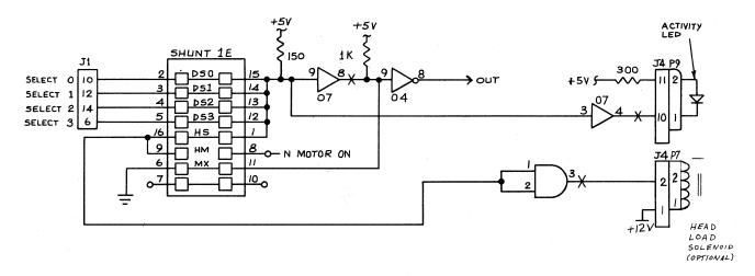
Figure 3-3 Select Lines Schematic Diagram
