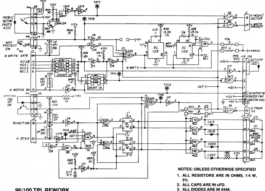
96/100 TPI, REWORK, UNIPOLAR LOGIC SCHEMATIC
