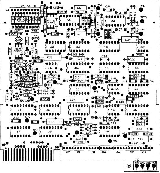
96/100 TPI UNIPOLAR LOGIC PCBA ASSEMBLY DRAWING
