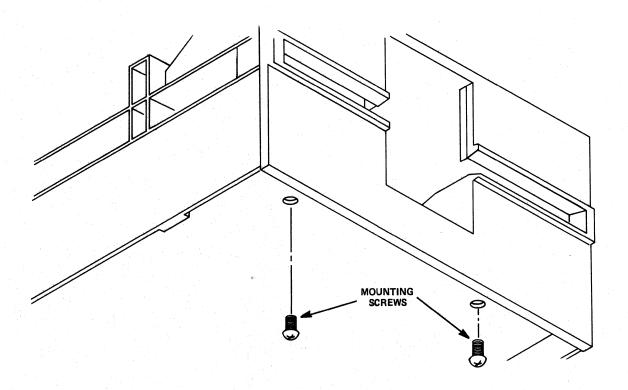
Figure 5-13 Front Panel Mounting Screws
