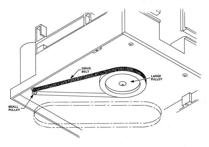
Figure 5-1 Drive Belt and Pulleys
