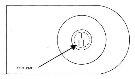
Figure 5-28 Felt Pad on Upper Arm
