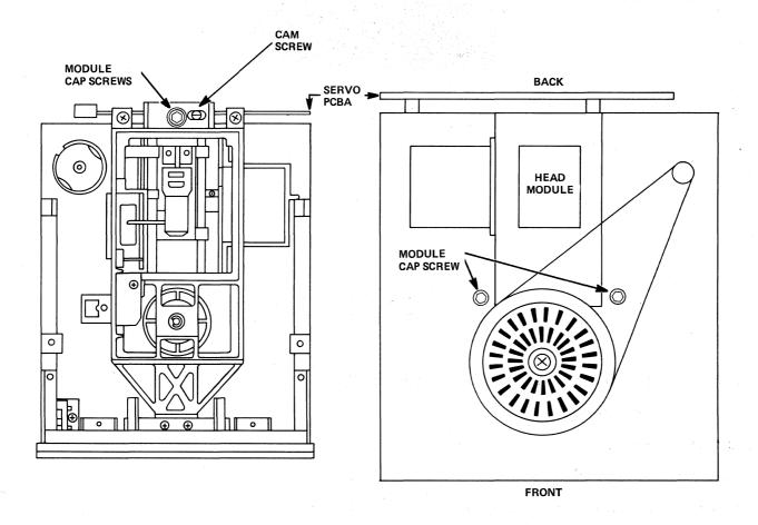
Figure 2-6 Head Module Cap and Cam Screws
