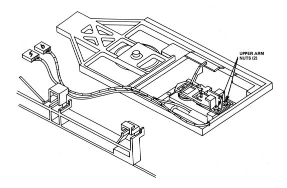
Figure 5-26 Nuts for Upper Arm and Spring Retainer
