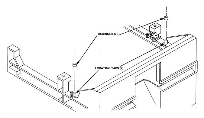
Figure 5-11 Front Panel Bushings
