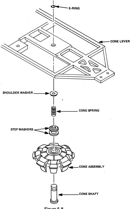
Figure 5-8 Cone's Component Parts
