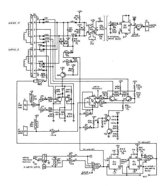
Figure 3-8 Write Data Schematic Diagram, Unipolar
