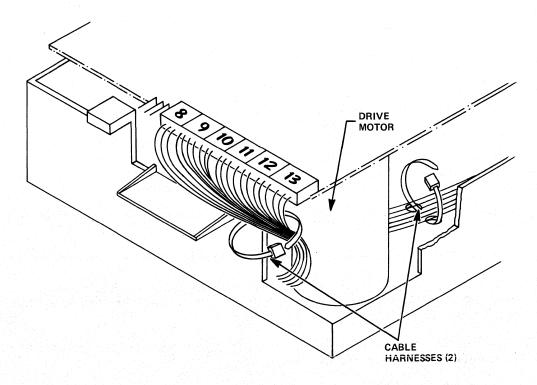
Figure 5-25 Write Protect Switch Assembly Cable Harnessing
