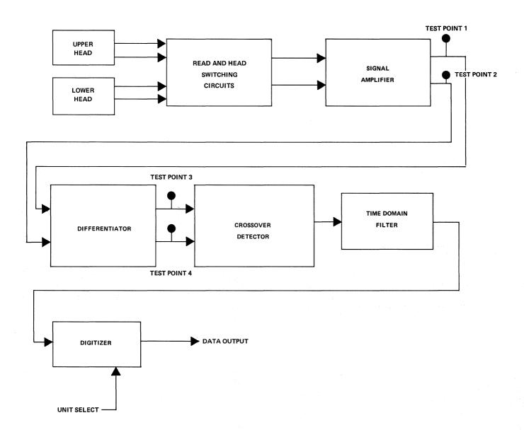
Figure 3-15 Read Circuit Block Diagram
