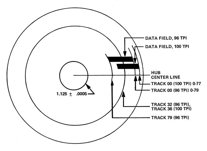
Figure 2-4 Hub Center Line and Track Locations
