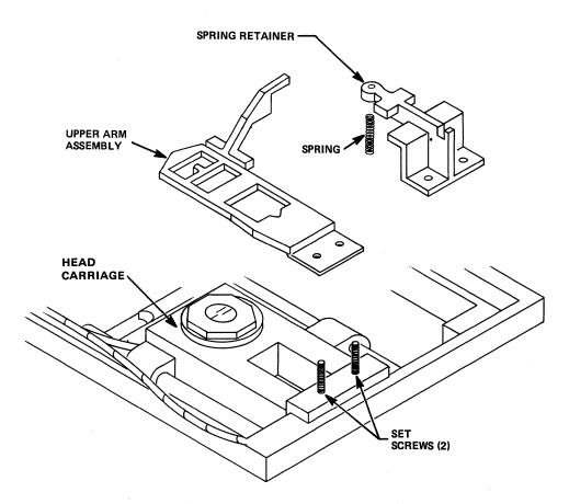
Figure 5-27 Upper Arm Assembly Parts
