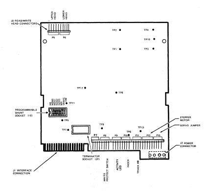
Figure 1-6 Logic Printed Circuit Board Assembly
