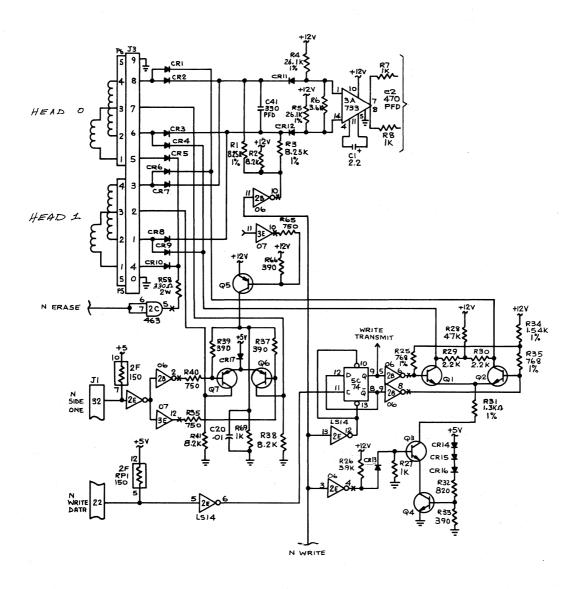
Figure 3-9 Side Select Schematic Diagram
