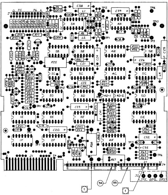
96/100 TPI BIPOLAR LOGIC PCBA ASSEMBLY DRAWING
