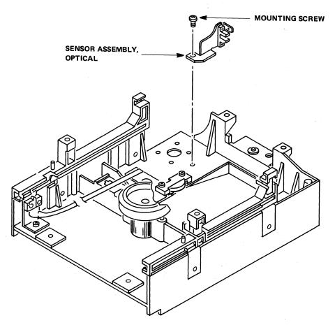
Figure 5-22 Track 00 Sensor Assembly and Mounting Screw
