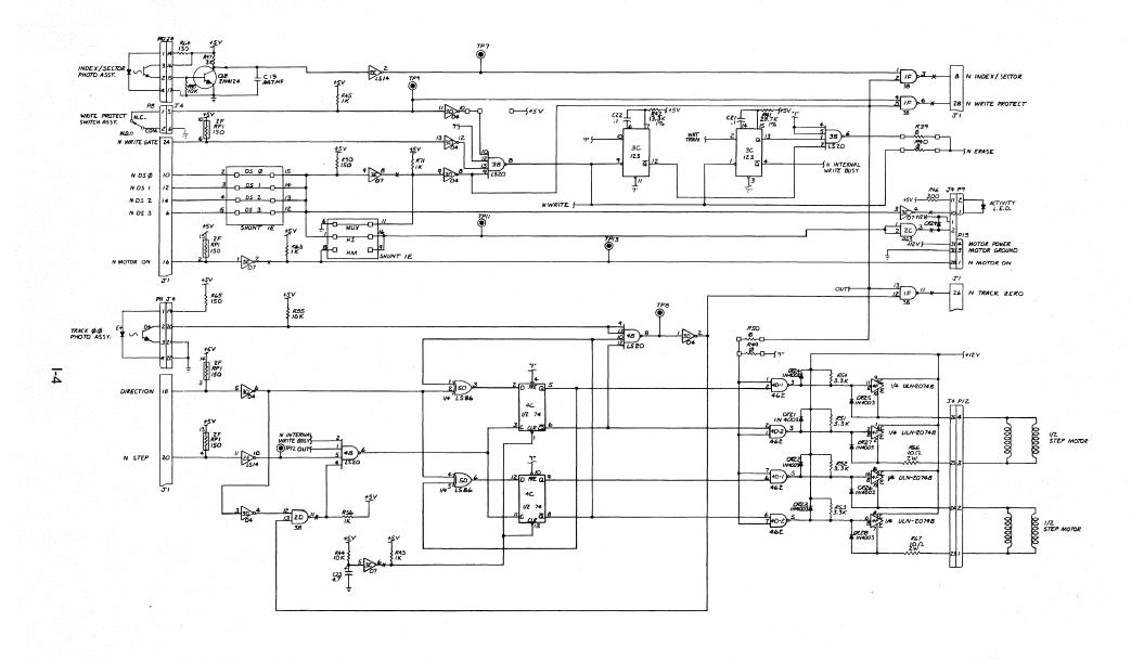
96/100 TPI BIPOLAR LOGIC SCHEMATIC
