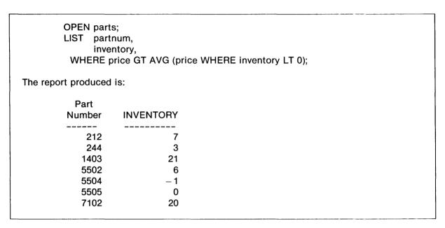
Figure 3-6. Qualification Aggregate With Embedded WHERE Clause
