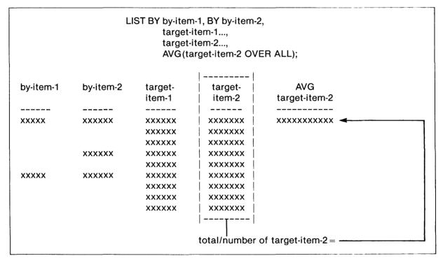
Figure 3-3. Query Outline of Target-Aggregate With OVER ALL Syntax
