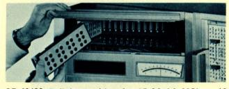
**SD 40/80:** Built-in provision for 15 Model 3351 or 10 Model 3352 high-resolution VDFG cards. Functions are set up with the help of a Model 3341 FG Set-up Unit which brings the VDFG card out into the open for easy screwdriver pot adjustment of breakpoint and slope.
