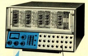
1 Meter Readout Ranges: 1, 3, 10, 30, 100, and 300 volts, and  $\pm$  null. Full scale accuracy: 3%. Null position provides 0.02% F.S. resolution with reference potentiometer having a  $\pm$ 0.05% linearity at 25°C.
