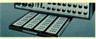
**SD 10/20:** A sliding tray (optional) mounted below the cabinet holds up to four 3351 VDFG cards. Four Model 3352 VDFG cards may be specified in place of the 3351.
