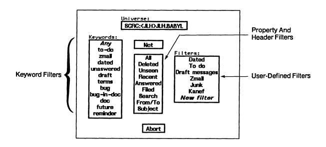
Figure 14. Filter Selection Display.
