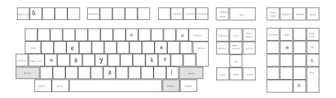
Figure 6. Open Genera Interpretation of the DEC LK401 AA Keyboard Using the Symbol and Shift Keys  $% \left( {{{\rm{S}}_{\rm{S}}}} \right)$
