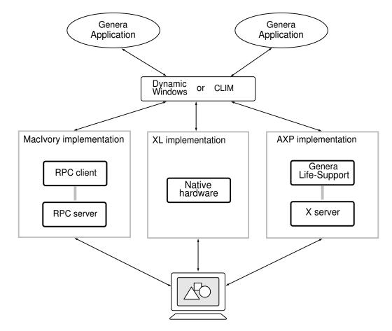
Figure 1. Open Genera User Interface Architecture
