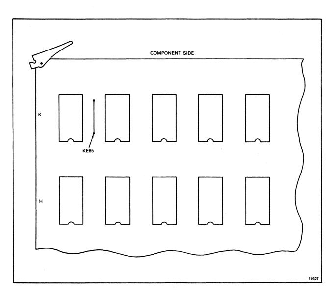
Figure 2-7. KG Card Jumper Location
