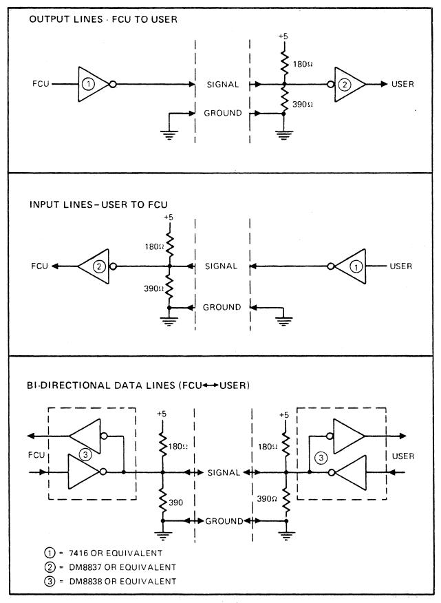
Figure 3-1. FCU-USER Interface Circuits
