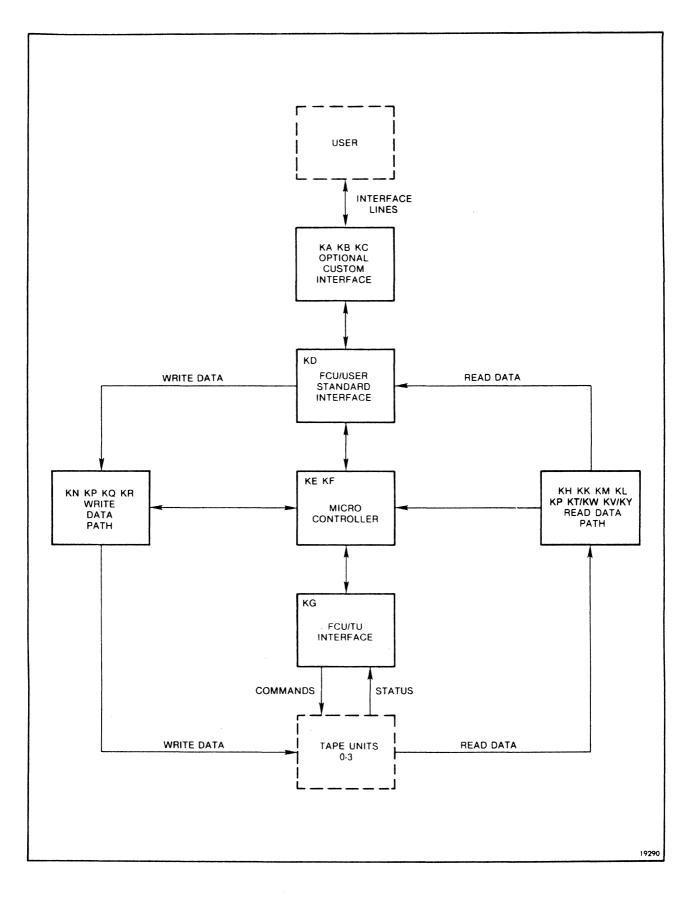
Figure 1-4. FCU General Block Diagram
