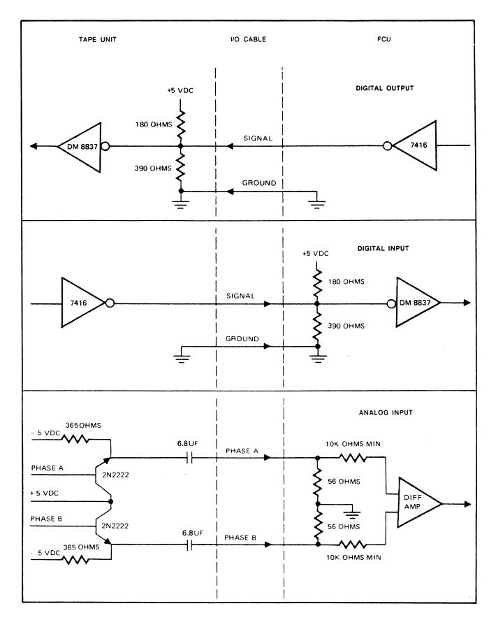
Figure 4-1. FCU/TU Interface Circuits
