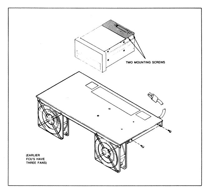
Figure 6-4. Cooling Fan Replacement
