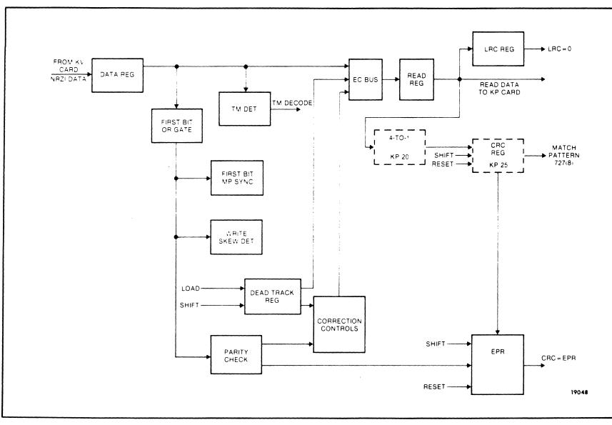
Figure 5-13. NRZI Read Data Path (KL Card)
