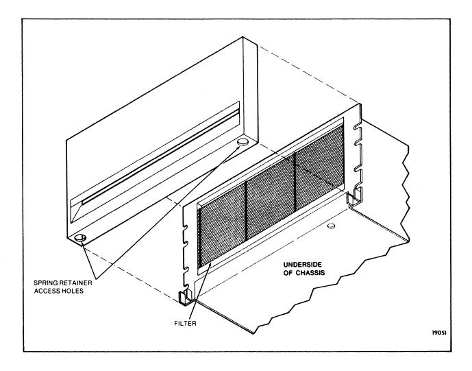
Figure 6-3. Filter Removal
