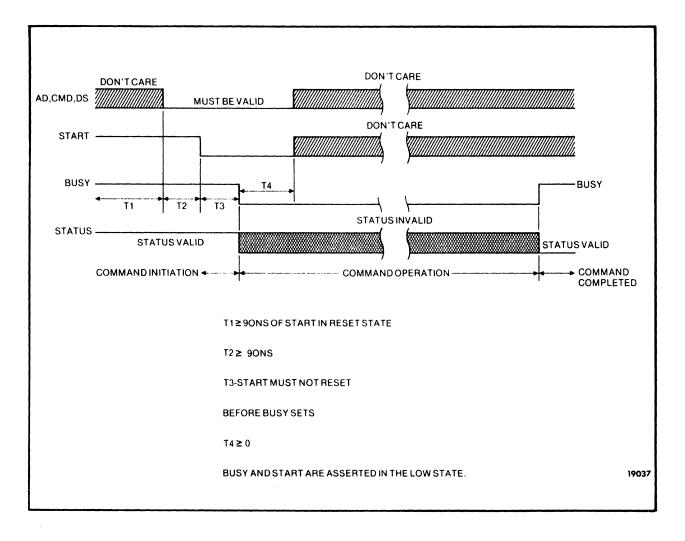
Figure 3-2. Command Initiation, Operation, and Completion
