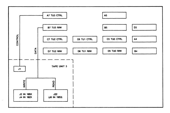
Figure 2-4. FCU/TU Interface Cable Connection
