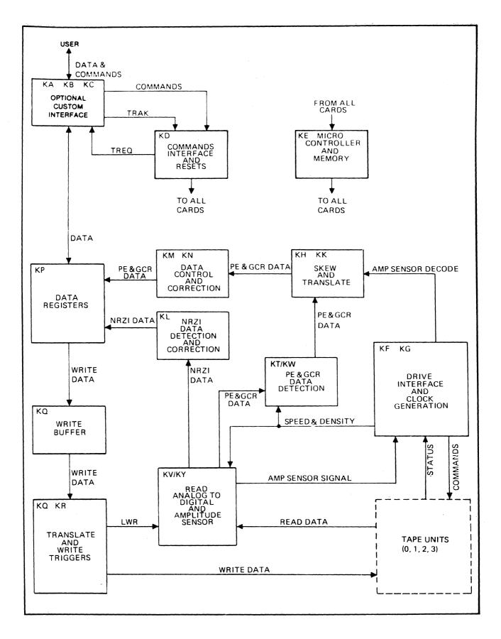
Figure 5-1. FCU Functional Block Diagram
