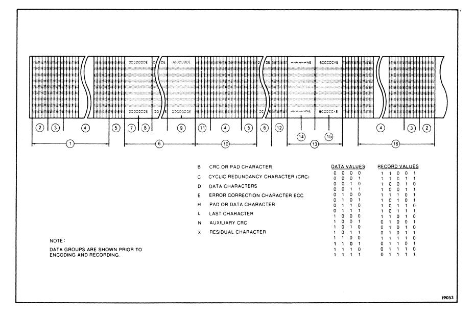
Figure A-4. GCR Data Block Format (Sheet 1 of 3)
