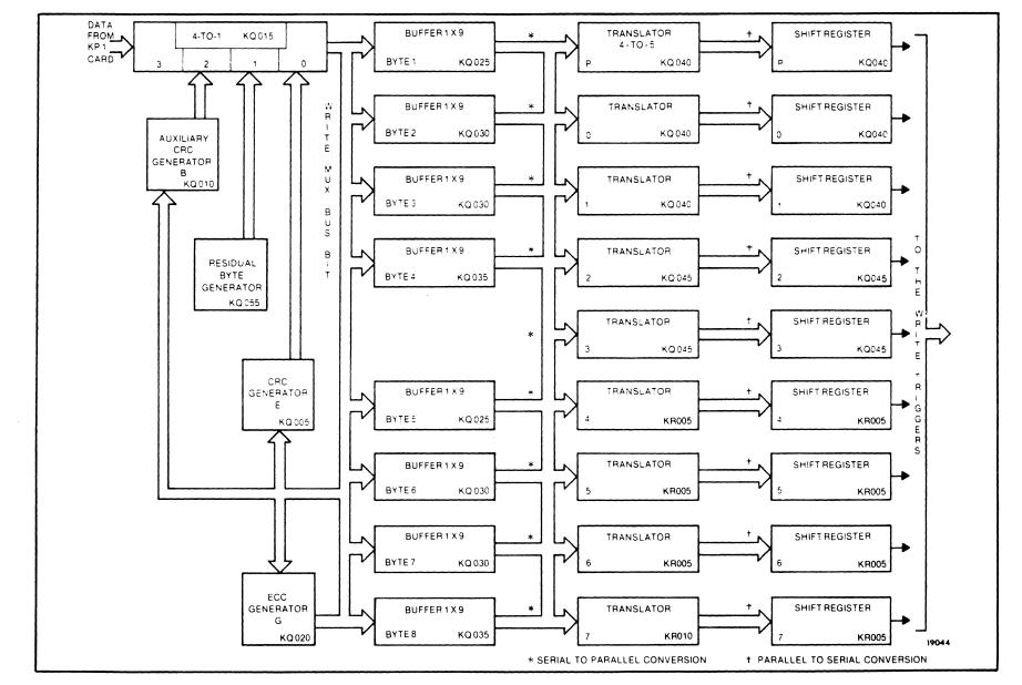
Figure 5-7. Write Data Path (GCR Only)
