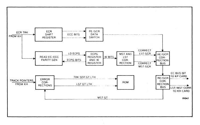
Figure 5-12. PE/GCR Read Data Path (KM Card)
