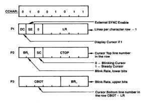
In graphics mode, LR should be set to 0. The blink rate parameter controls both the cursor and attribute blink rates. The cursor blink-on time = blink-off time =  $2 \times BR$  (video frames). The attribute blink rate is always  $\frac{1}{2}$  the cursor rate but with a  $\frac{3}{4}$  on  $\frac{1}{4}$  off duty cycle. All three parameter bytes must be output for interlace displays, regardless of mode. For interlace displays in graphics mode, the parameter eter BR<sub>i</sub> = 3.
