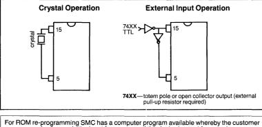
or ROM re-programming SMC has a computer program available whereby the customer need only supply the input frequency and the desired output frequencies. The ROM programming is automatically generated.
