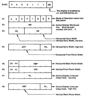
This command also loads parameters into the sync generator. The various parameter fields and bits are identical to those at the RESET command. The HGDC is not reset nor does it enter idle mode.
