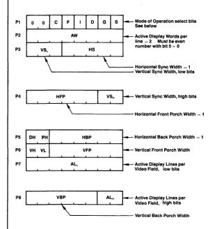
In graphics mode, a word is a group of 16 pixels. In character mode, a word is one character code and its attributes, if any. The number of active words per line must be an even number from 2 to 256. An all-zero parameter value selects a count equal to  $2^n$  where n = number of bits in the parameter field for vertical parameters. All horizontal widths are counted in display words. All vertical intervals are counted in lines.
