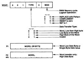
Upon receiving a set of parameters (two bytes for a word transfer, one for a byte transfer), one RMW cycle into Video Memory is done at the address pointed to by the cursor EAD. The EAD pointer is advanced to the next word, according to the previously specified direction. More parameters can then be accepted.
