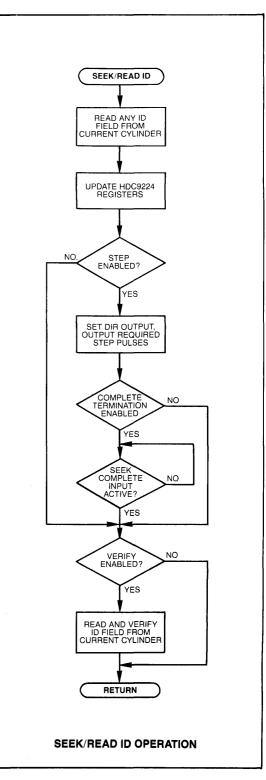
disk. If the UDC is unable to find an ID Field sync mark within 33,792 byte times, the SYNC ERROR bit (in the CHIP STATUS register) is set to "1", and the command is terminated.
