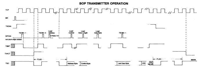
Note 1—Trailing edge of DPENA must occur at least one-half clock pulse prior to TBMT = 1. To avoid underrun.
