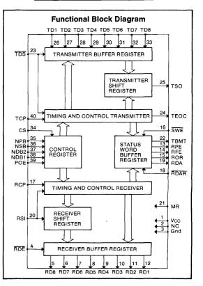
At start-up the power is turned on, a clock whose frequency is 16 times the desired baud rate is applied and master reset is pulsed. Under these conditions TBMT, TEOC, and TSO are all at a high level (the line is marking).
