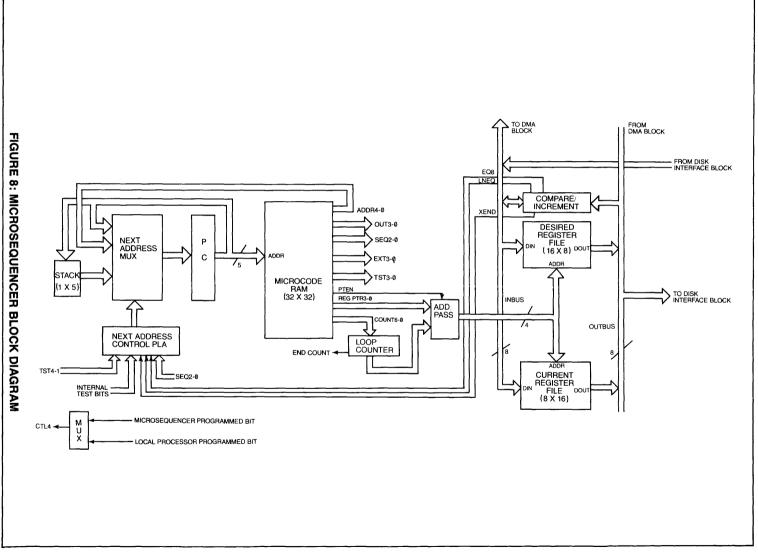
DESIRED REGISTER FILE holds information such as the desired sector to be operated on in a READ or WRITE DISK operation. The desired header information, in this case is written into the DESIRED REGISTER FILE by the Local Processor prior to the execution of the READ OR WRITE command in an order that is consistent with the order in which the MICROSEQUENCER loads and compares the CURRENT REGISTER FILE.
