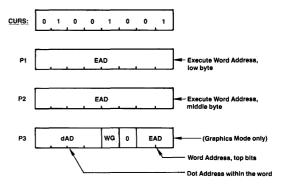
In character mode, the third parameter byte is not needed. The cursor is displayed for the word time in which the display scan address (DAD) equals the cursor address. In graphics mode, the cursor word address specifies the word containing the starting pixel of the drawing; the dot address value specifies the pixel within that word.
