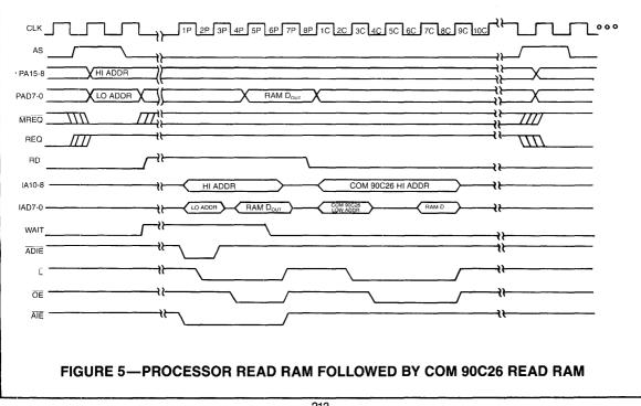
and driven out via the logic function RD ended with <u>REQ</u>. For <u>processor</u> I/O read cycles from the COM 90C26, <u>ADIE</u> and <u>AIE</u> are used to enable the processor address into the COM 90C26. Data out of the COM 90C26 is gated through the transparent latch and appears on the processor's data bus with the same control signals used for RAM read cycles.
