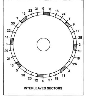
The UDC can format a track with interleaved sectors by staggering the sector numbers. For example, to format a 32 sector track, with a sector interleave factor of 4, the system processor would set up the ID Field table sector numbers as follows:
