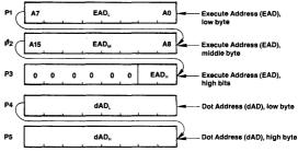
The Execute Address, EAD, points to the display memory word containing the pixel to be addressed.
