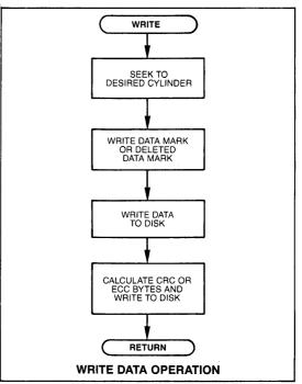
Before writing data to the selected disk drive, the UDC will read the current ID field, step to the desired cylinder (if enabled in command) and verify that has located the correct cylinder and sector. (These steps were described previously under "UDC Command Overview").
