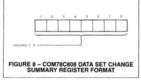
then be obtained from that line's status register. If the state of a line changes twice within one microsecond, the change in state may not be detected. Figure 8 shows the format of the data set change summary register.
