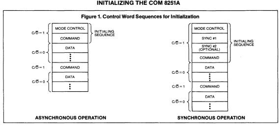
The COM 8251A may be initialized following a system RESET or prior to starting a new seral I/O sequence. The USART must be RESET (external or internal) following power up and subsequently may be reset at any time following completion of one activity and preceding a new set of operations. Following a reset, the COM 8251A enters an idle state in which it can neither transmit nor receive data.
