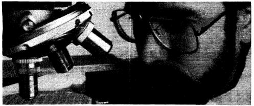
The laser cutter in SMC<sup>®</sup>'s Special Analysis Laboratory helps isolate small sections of complex circuitry for investigation.
