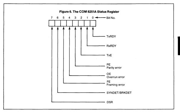
TxE signals the processor that the Transmit Register is empty.
