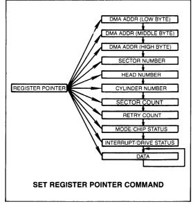
reduces the number of times the user must set the register pointer during read and write operation.
