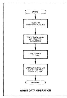
Before writing data to the selected disk drive, the UDC will read the current ID field, step to the desired cylinder and verify that it has located the correct cylinder and sector. (These steps were described previously under "UDC Command Overview").
