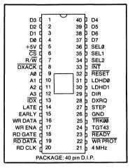
Read/Write on one Drive while Seeking on another for Enhanced System Throughput Three On-Chip Status Registers TTL Compatible Inputs and Outputs +5 Volt Only Operation FLOPPY DISK INTERFACE
