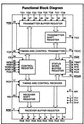
At start-up the power is turned on, a clock whose frequency is 16 times the desired baud rate is applied and master reset is pulsed. Under these conditions TBMT, TEOC, and TSO are all at a high level (the line is marking).
