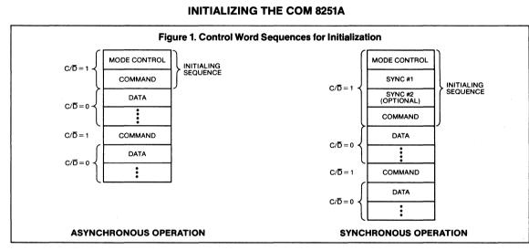
The COM 8251A may be initialized following a system RESET or prior to starting a new seral I/O sequence. The USART must be RESET (external or internal) following power up and subsequently may be reset at any time following completion of one activity and preceding a new set of operations. Following a reset, the COM 8251A enters an idle state in which it can neither transmit nor receive data.
