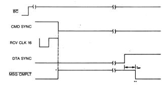
\*WORD COUNTER PRESET TO COUNT IN COMMAND WORD \*\*MSG CMPLT GENERATED BY LAST DATA SYNC OF THE MESSAGE GROUP
