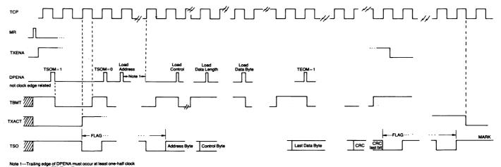
pulse prior to TBMT=1. To avoid underrun.
