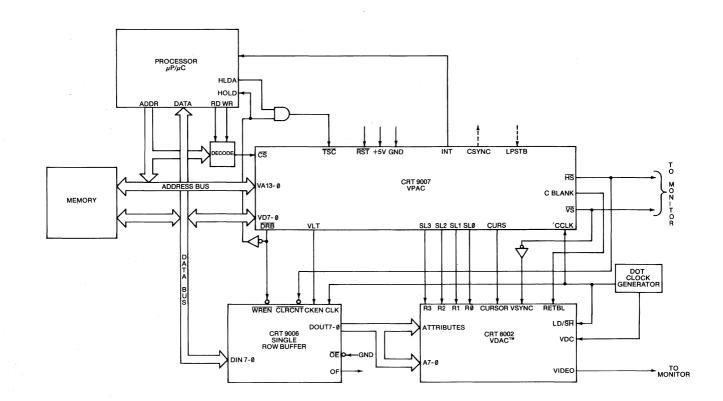
Figure 2. VPAC Configuration With Single Row Buffer
