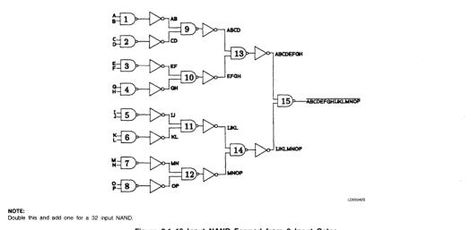
Figure 2.1 16 Input NAND Formed from 2 Input Gates
