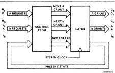
a. A and b service requests  $(R_N,\,r_N)$  plus the present state determine, through the control PROM, the next state and the next grant outputs  $(G_N,\,g_N)$ .
