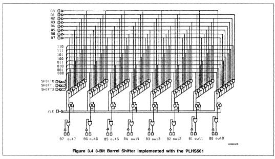
An eight bit barrel shifter exploits most of the PLHS501 as depicted in Figure 3.4. This implementation utilizes all 72 internal foldback NANDs in a relatively brute force configuration as well as 8 output NANDs to generate transparent latched and shifted results. The shift position here is generated by the shift 0, shift 1 and shift 2 inputs which are distinguished and selected from the input cells. Variations on this idea of data manipulation could include direct passing data, mirror
