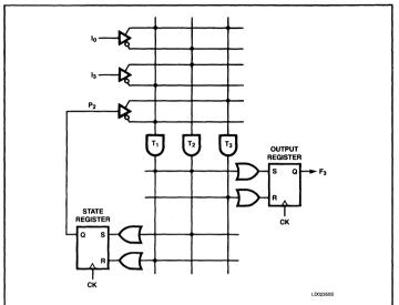
Figure 25. Typical OR Array Gating of Transition Terms T<sub>1,2,3</sub> Controlling Arbitrary State and Output Register Stages.
