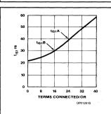
Figure 2. PLS105A t<sub>IS1</sub> vs. Terms/OR Connected
