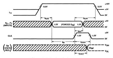
Diagnostic Mode - State Register Input Jam
