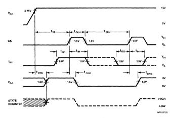
Test Circuit Timing Diagram
