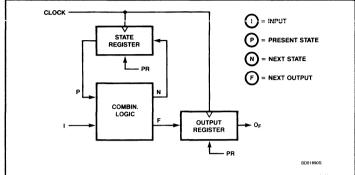
Figure 17. Basic Architecture of PLS105 FPLS. I, P, N, and F are Multi-line Paths Denoting Groups of Binary Variables Programmed by The User.
