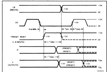
\* The leading edge of preset/reset must occur only when the input clock is "low", and must remain "high" as long as required to override clock. The falling edge of preset/reset can never go "low" when the input clock is "high".
