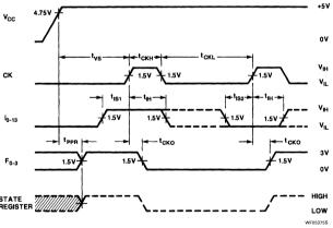
Test Circuit Timing Diagram
