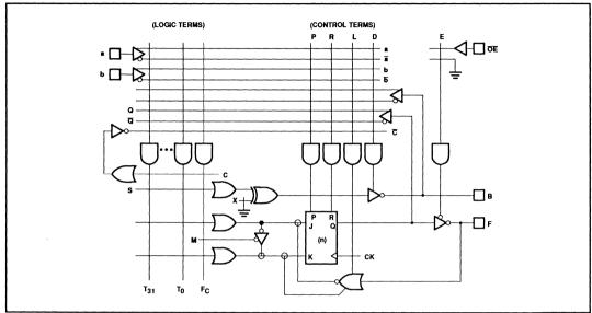
On-chip T/C buffers couple either True (I, B, Q) or Complement (I, B, Q, C) input polarities to all AND gates, whose outputs can be optionally linked to all OR gates. Any of the 32 AND gates can drive bidirectional I/O lines (B), whose output polarity is individually programmable through a set of Ex-OR gates for implementing AND-OR or AND-NOR logic functions. Similarly, any of the 32 AND gates can drive the
