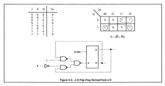
If required, J–K flip–flops can be constructed from D flip–flops by utilizing the structure shown in Figure 4–5, as a substitution. The sum term is taken from the NAND physically connected to the D flip–flop and the K input may be derivable from either an input inverter or a  $\Omega$  from a flip–flop. There will be a penalty for using this structure from a speed point, but it may save gates if used judiciously.
