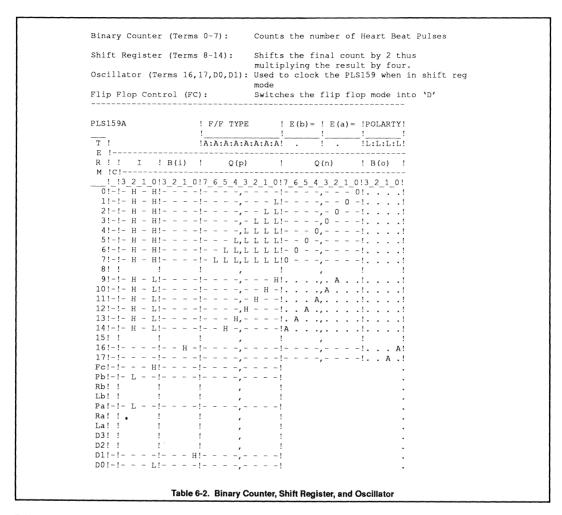
Table 6-2 illustrates the implementation of the binary counter, shift register, and oscillator. '12' is the RESET signal input. '10' is the '15\_SEC' signal input used to enable/disable the counter, shift register, and oscillator. 'B0' is the oscillator output used to clock the PLS159A when it is in the shift register mode.
