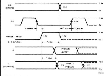
\* The leading edge of preset/reset must occur only when the input clock is "low", and must remain "high" as long as required to override clock. The falling edge of preset/reset can never go "low" when the input clock is "high".
