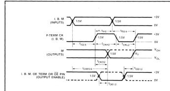
Flip-Flop Outputs with P-term Clock
