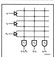
Figure 24. Typical Transition Terms Involving Arbitrary Inputs and State Variables. All Remaining Gate Inputs Are Programmed Don't Care. Note That T<sub>2</sub> Output is State Independent.
