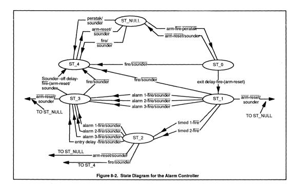
Detect inputs can be divided into timed, untimed, fire and personal attack inputs. Timed circuits allow entry/exit delay circuits for front and rear doors, to delay operation of the alarm for approximately 16 seconds. Untimed circuits cause the alarm to operate immediately when an alarm condition occurs. These would be used to protect unusual means of entry, such as windows. Both the timed and untimed circuits should operate only if the system is armed.
