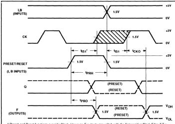
Preset and Reset functions override Clock. However, F outputs may glitch with the first positive Clock Edge if T<sub>IS1</sub> cannot be guaranteed by the user.
