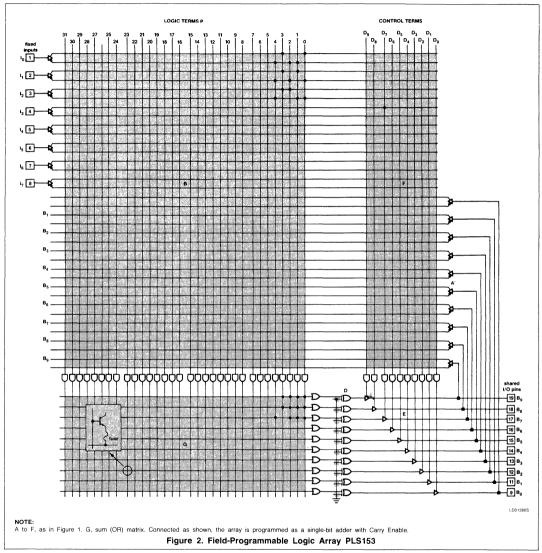
At the same time, and without using any additional inputs, output  $\mathsf{B}_{10}$  (fuse blown) is programmed
