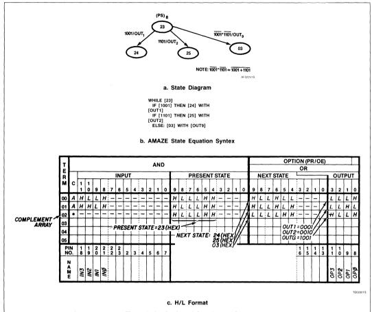
Figure 6. Application of Complement Array
