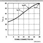
Figure 1. PLS168 t<sub>IS1</sub> vs. Terms/OR Connected
