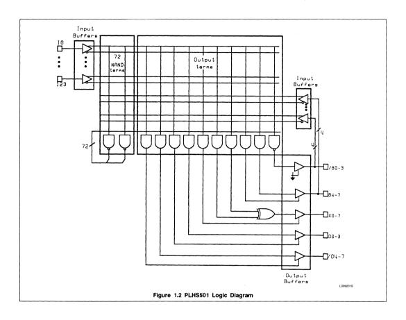
The data sheet first lists some maximum propagation delays from an input, through a NAND output term and out through various output gates. Secondly, it lists maximum propagation delays from an input, through a NAND foldback term, through a NAND output term and out through the different output gates.
