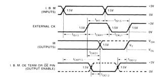
Flip-Flop Outputs with External Clock
