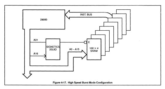
Consider, for example, the configuration depicted in Figure 4-17 with Motorola MCM 6288 SRAMs. As depicted, there are eight modules forming a 16K word space. The 29000 is targeted to drive 80pf according to the data manual at full speed (25MHz clock). How much additional time delay will be attributed to the bus and RAM loading?
