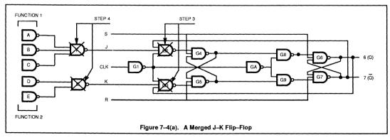
It is hoped that the reader can, in general, avoid the use of the J-K structures built from gates as shown due to their inefficiency of gate usage. There is also a potential timing liability
