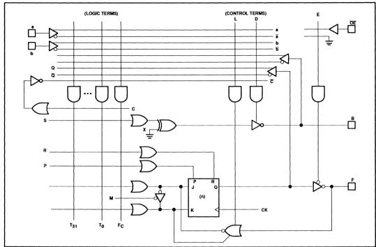
On-chip T/C buffers couple either True (I, B, Q) or Complement (I, B, Q, C) input polarities to all AND gates, whose outputs can be optionally linked to all OR gates. Any of the 32 AND gates can drive bidirectional I/O lines (B), whose output polarity is individually programmable through a set of Ex-OR gates for implementing AND-OR or AND-NOR logic functions. Similarly, any of the AND gates can drive the J-K
