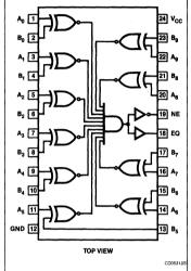
Figure 1. Logical Equivalent Circuit of 10-Bit Comparator
