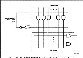
Figure 26. The COMPLEMENT Array is Logically Constructed from a multiple input Programmable NOR Gate. All AND Terms Coupled to the OR Gate are Complemented at the Inverter Output, and Can be Fed Back as Inputs to the AND Array.
