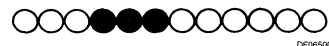
NOTE: The strands of one turn are indicated by black dots. Figure 25. A Multiple-Wire Winding of 4 Turns, Each of 3 Strands
