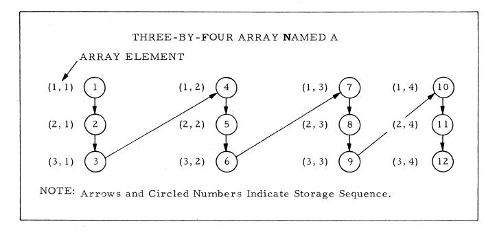
Figure 2-1. Two-Dimensional Array, Storage Sequence of Elements
