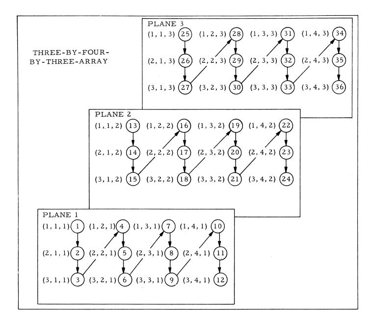
Figure 2-2. Three-Dimensional Array, Storage Sequence of Elements
