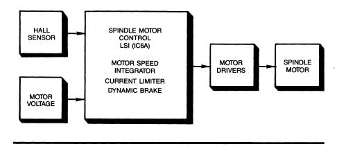
FIGURE 27: Motor Speed Control: PC Board 20292-XXX
