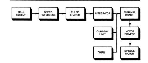
FIGURE 28: Motor Speed Control PC Board 20249-XXX
