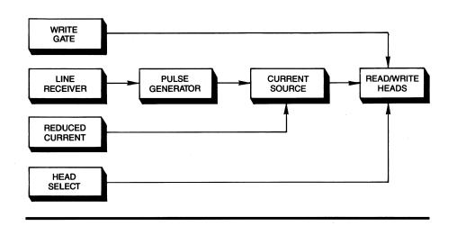
FIGURE 21: Write Operation PC Board 20243-XXX
