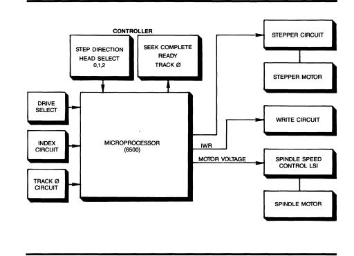
FIGURE 25: MPU: PC Board 20292-XXX
