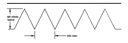
FIGURE 30: Differential Read Filter
