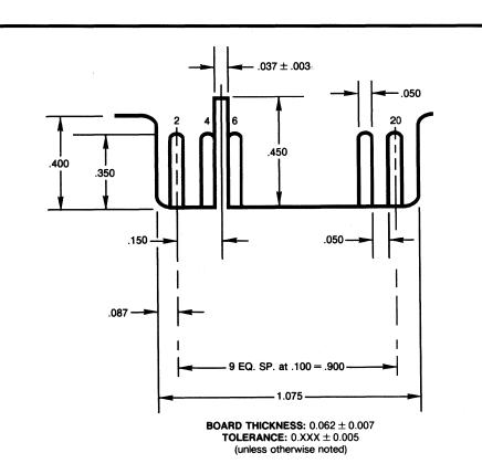
FIGURE 5: J2 Connector Dimensions TABLE 2: J2 Host/Drive Pin Assignments
