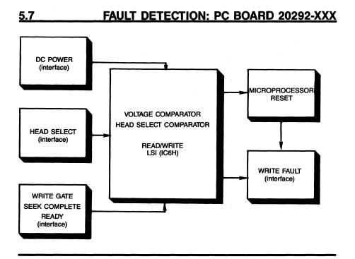
FIGURE 17: Fault Detection PC Board 20292-XXX
