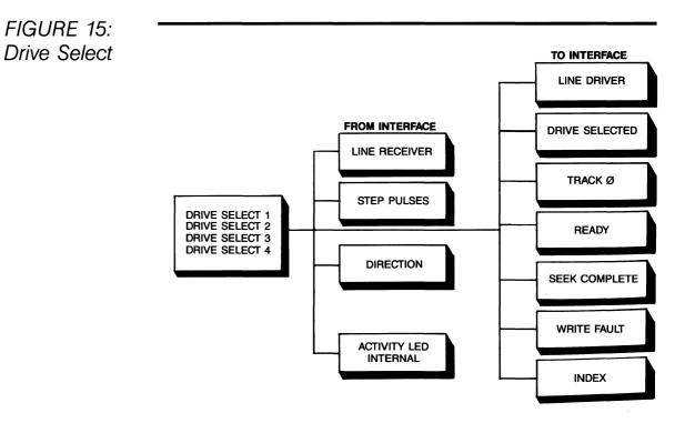
The control output signals are gated to the interface when selected. They are: DRIVE SELECTED, INDEX, TRACK Ø, READY, SEEK COMPLETE and WRITE FAULT.
