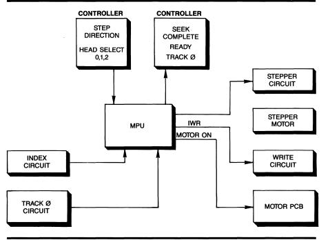
The microprocessor monitors and controls the internal drive functions and the host interface lines. The MPU has only three active modes: Initializing, Seeking, Waiting.
