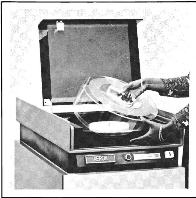
Figure 23. Removing Top Canister Cover from Installed Disk Pack
