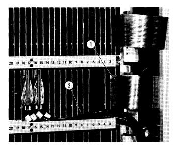
The ZT52 wire used to interconnect backpanel wire wrap pins has two special mechanical features. The insulation is especially tough, to resist cold flow; and, the copper conductor has the proper tensile strength to provide a firm wrap without loosening the pin. Electrically, the wire behaves as a 150-ohm transmission line, when pushed close to the ground plane that is built into all SDS mounting cases. The ground plane protects the signal.
