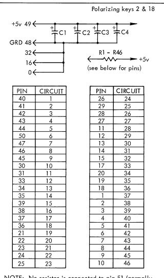
NOTE: No resistor is connected to pin 51 (normally the +8v connection) or to pins 0, 16, 32, 48 (ground). The Test Lamp Assembly plugs on the front edge of any J Series module that has test points on the front edge. The XJ11 contains ten independent test lamp circuits on a module with a special connector mounted at the back. Each lamp circuit input connects to one test point on the module under test.
