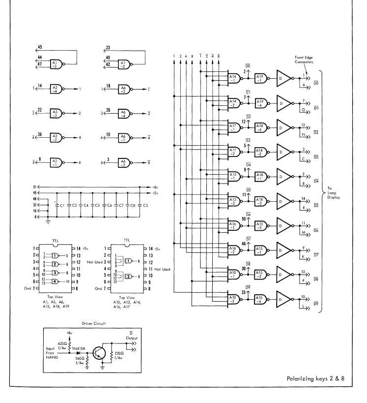
The BJ61 contains a binary input to 16-line output decoder.
