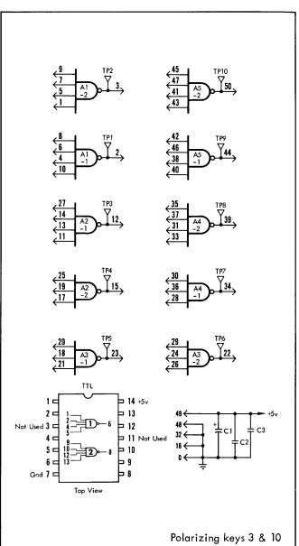
The IJ62 module contains fourteen inverters and six 2-input NAND gates. The 2-input NANDs perform the function  $Q = \overline{AB}$ . An unwired input functions as if it were wired True.
