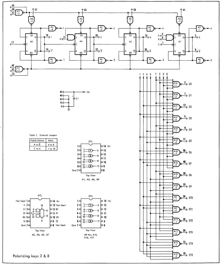
This module contains three identical decades of clocked BCD counting on one module. It functions as either upcounter or down-counter, depending on whether the control signals at pins 9, 25, and 41 are high (up) or low (down).
