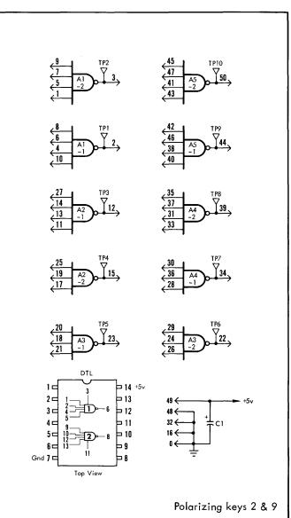
The IJ12 module contains fourteen inverters and six 2-input NAND gates. The 2-input NANDs perform the function  $Q = \overline{AB}$ . An unwired input functions as if it were wired True.
