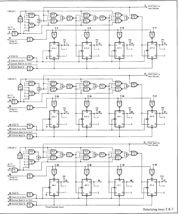
The FJ19, FJ20, and FJ21 are high-density buffered-latch storage register modules. Each module contains two registers. The two FJ19 registers have 8 bits each; FJ20 registers have 10 bits each; and FJ21 registers have 12 bits each.
