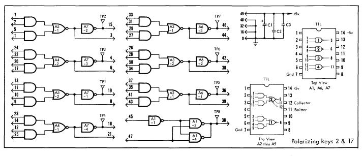
The LJ66 module contains a 4-bit parallel binary full-adder with ripple carry between stages. The module also contains four 2-input NANDs which permit the adder to be used with single-ended (True input only) data signals. The NANDs can be used for other logic functions if not needed at adder input. Refer to logic diagrams 1 and 2, and schematic diagram.
