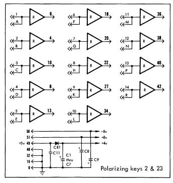
and provide a convenient method of interfacing J Series with T Series. However, there is a logical inversion in going through an AJ driver-receiver chain, but no inversion in going through the AT chain.
