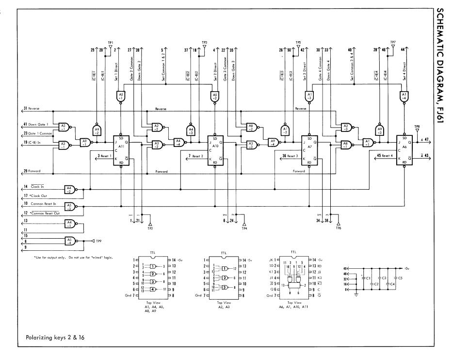
The FJ62 module contains five independent, gated, clocked JK flip-flops. Each J and K input is preceded by a 2-input AND gate. Logic levels appearing at these gates enter the flip-flop only in conjunction with a clock signal.
