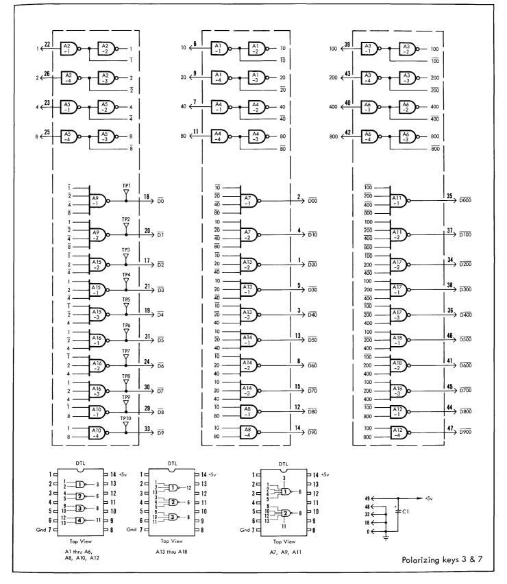
The BJ60 contains both a BCD to 10-line decoder and a group of ten indicator lamp (or relay) drivers. In addition, two independent 2-input NANDs are supplied on the module.
