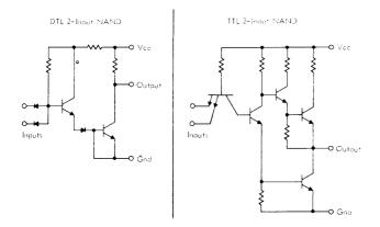
The differing circuit structures lead to performance differences in four main areas: speed (clock rate), noise level, power consumption, and logic flexibility. J Series modules exhibit differences in only three of these areas: speed, power, and logic flexibility, because special precautions have been taken to reduce noise.
