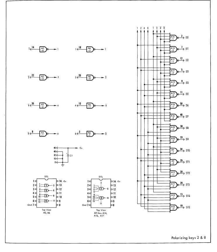
The BJ12 contains three independent decades of decoding, each with BCD input and 10-line output.
