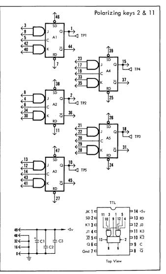
The FJ63 module contains four 4-bit buffer storage registers. It is constructed entirely of 2-input NANDs, arranged as buffered latches with strobed gates at inputs and outputs. Each 4-bit section is independent of the others, and has its own common reset line, set strobe (load strobe), and readout strobe. Only the complement of the input data is available at the outputs.
