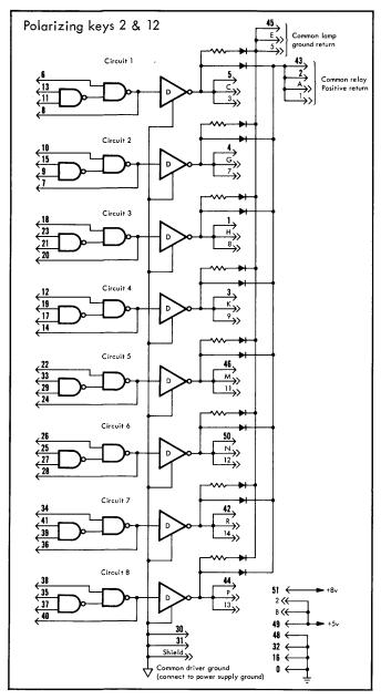
for an ET11 connector to permit routing of outputs to remote lamps or relays. (The single connector symbols indicate back panel contacts).
