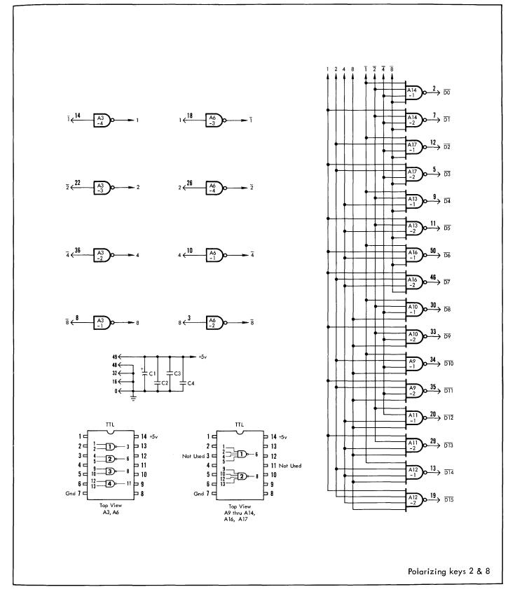
The BJ62 contains three independent decades of decoding, each with BCD input and 10-line output.
