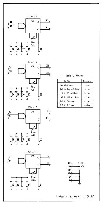
The OJ18 contains four one-shot circuits (sometimes called single-shots) which produce both Q and Q output, of pulse-width that is continuously adjustable from 100 nsec to 20  $\mu$ sec (see Table 1).
