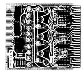
The AT22 module contains two Schmitt Trigger circuits. Three input ranges are provided. Each Q output rises to +5v when input exceeds the adjustable trigger level, and returns to 0v when input drops below the adjustable hysteresis level, which is always more negative than the trigger level. Thus the trigger adjustment (R4) adjusts timing of the output leading edge while the hysteresis adjustment (R13) adjusts timing of the output trailing edge.
