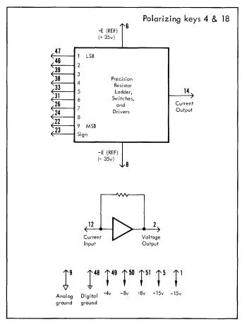
The output voltage is related to digital input as shown in Table 1.
