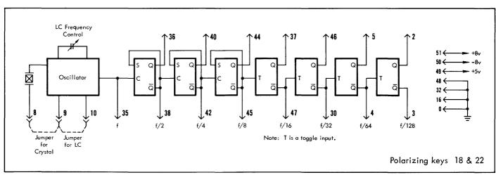
The CT10 contains a 1 MHz to 10 MHz oscillator, a pulse shaper, and a gated clock amplifier (driver). The oscillator is controlled by an adjustable LC circuit or optionally by a plug-in crystal. External jumpers select range (see table 1). When crystal control is desired frequency must be specified by the user. When using crystal, first adjust to approximate frequency using LC control with jumper 45-20 in place. Then remove jumper 45-20 and insert crystal.
