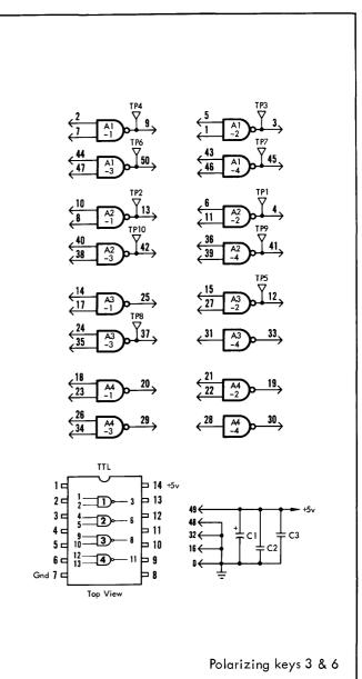
The IJ61 module contains six 4-input NAND gates and four 3-input NAND gates, which perform the function  $Q = \overrightarrow{ABCD}$  and  $Q = \overrightarrow{ABC}$  respectively. An unwired input functions as if it were wired True.
