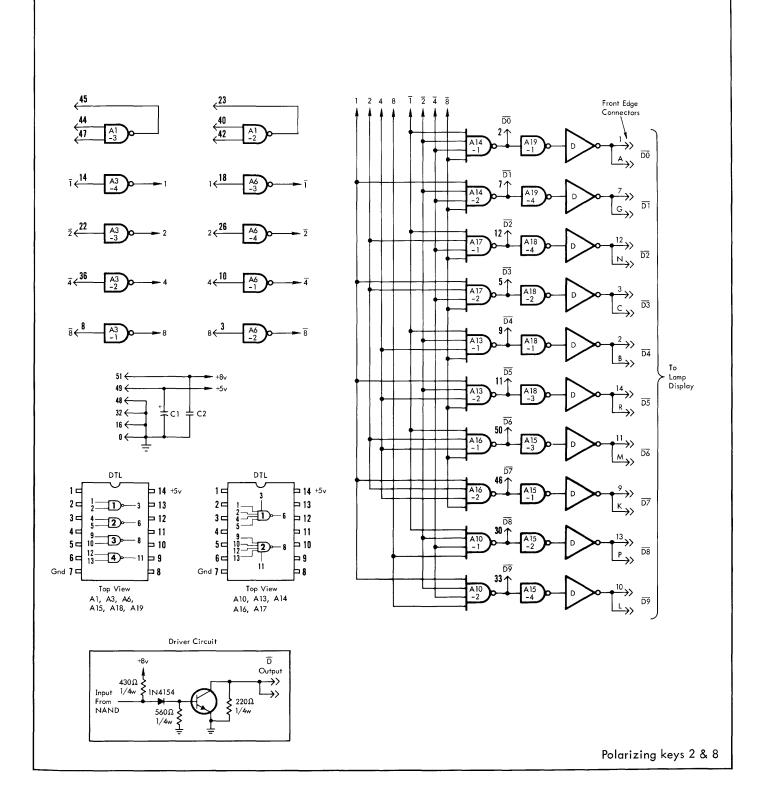
The BJ11 contains a binary input to 16-line output decoder.
