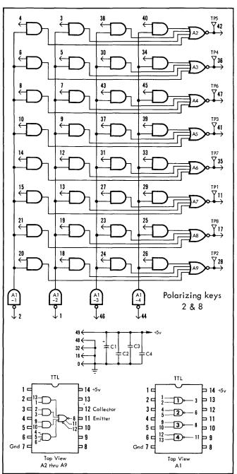
The LJ62 contains seven AND-NOR gates with complementary outputs, and one logic driver/inverter. Each gate performs both functions Q = AB + CD and  $\overline{Q} = \overline{AB} + \overline{CD}$ . If used for the Exclusive-Or function, apply complementary inputs of the same two signals as shown in the example.
