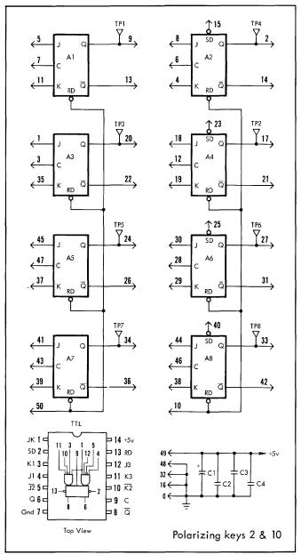
The FJ61 contains four JK flip-flops and gating to permit operation as a 4-bit synchronous binary up-counter, a 4-bit synchronous binary down-counter, a 4-bit right-shift register, or a 4-bit left-shift register.
