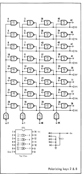
The LJ12 contains seven AND/NOR gates with complementary outputs, and one logic driver/inverter. Each gate performs both functions Q = AB + CD and  $\overline{Q} = \overline{AB} + CD$ . If used for the Exclusive-OR function, apply complementary inputs of the same two signals as shown in the example.
