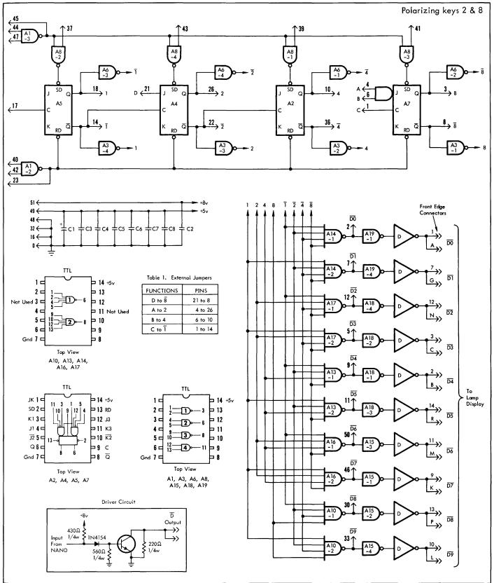
The FJ67 contains a 4-bit binary ripple-through up-counter and a binary to 16-line decoder. The counter has strobed individual direct-set inputs for presetting, as well as a gated common reset line.
