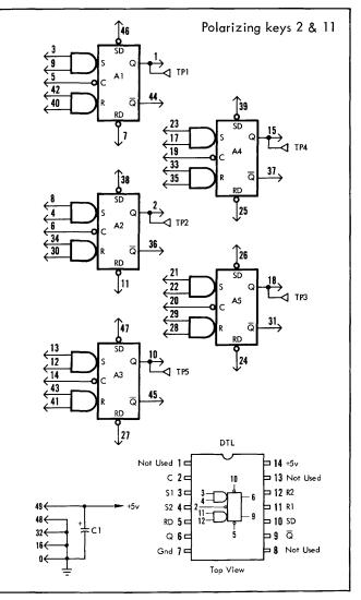
The FJ13 module contains four 4-bit buffer storage registers. It is constructed entirely of 2-input NANDs, arranged as buffered latches with strobed gates at inputs and outputs. Each 4-bit section is independent of the others, and has its own common reset line, set strobe (load strobe), and readout strobe. Only the complement of the input data is available at the outputs.
