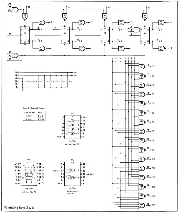
This module contains three identical decades of clocked BCD counting on one module. It functions as either upcounter or down-counter, depending on whether the control signals at pins 9, 25, and 41 are high (up) or low (down).
