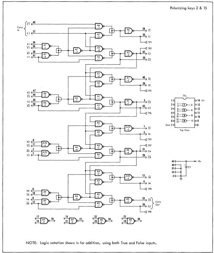
LJ17 contains five 8-input NANDs, each composed of two 4-input NANDs on a single type 930 chip, connected via etch as shown below. Because both inputs and outputs of the two inverters are paralleled, input loading and fan-out are doubled.
