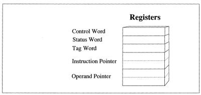
Figure 18-2 Coprocessor Control Registers
