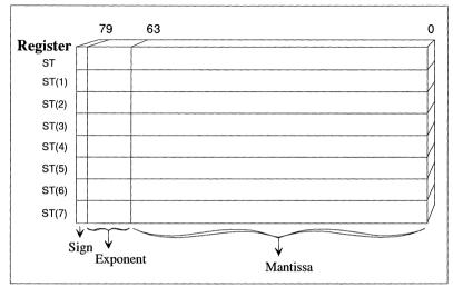
Figure 18-1 Coprocessor Data Registers
