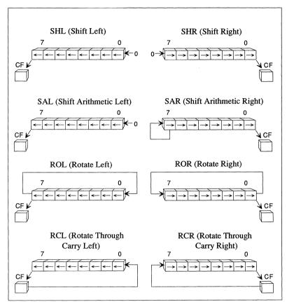
Figure 15-1 Shifts and Rotates
