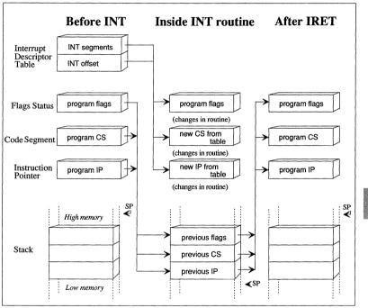
Figure 16-3 Operation of Interrupts
