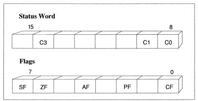
Figure 18-3 Coprocessor and Processor Control Flags
