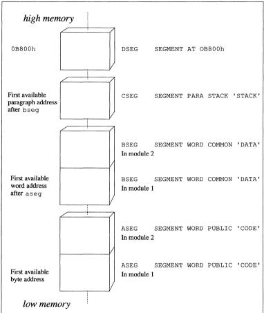
Figure 4-1 Segment Structure with Combine and Align Types
