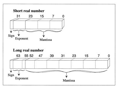
Figure 5-1 Encoding for Real Numbers in IEEE Format
