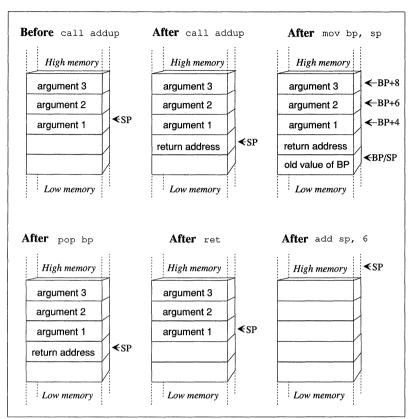
Figure 16-1 Procedure Arguments on the Stack
