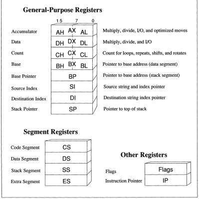
Figure 12-1 Register for 8088-80286 Processors
