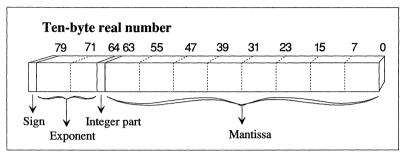
Figure 5-3 Encoding for Real Numbers in Temporary-Real Format
