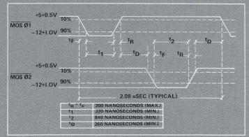
Figure 9 - Clock Pulse Requirements
