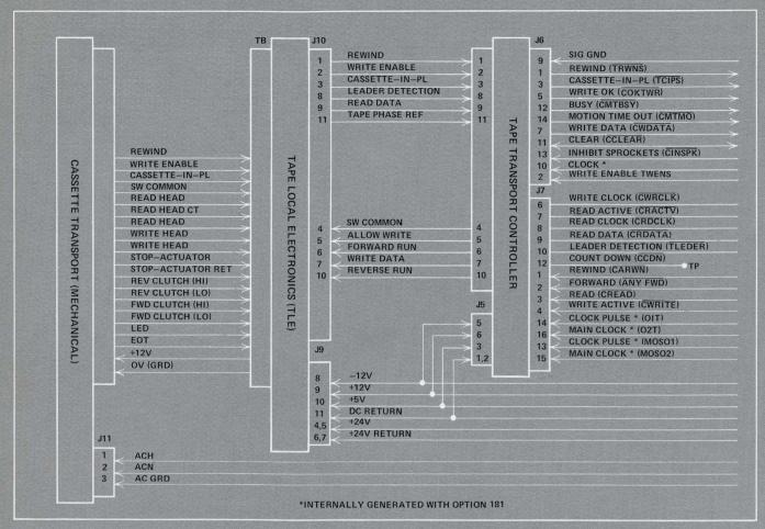
Figure 8 – Interface Connections
