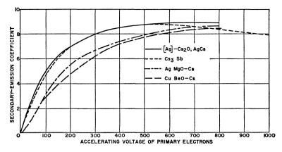
Fig. 30. Secondary emission coefficient for a number of dynode materials.
