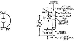
SIDE-ON type having S-1 response. Wavelength of maximum spectral response is  $8000 \pm 1000$  angstroms. This type makes use of a semicylindrical photocathode, and has a direct interelectrode capacitance of 3 picofarads. It weighs approximately 1.1 ounces. For curves of typical anode characteristics, refer to type 1P41. For outline and terminal-connection diagram, refer to type 1P29.
