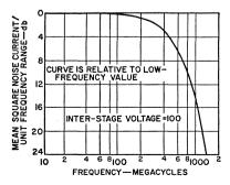
Fig. 56. Power spectrum of the noise from the RCA 981 multiplier phototube operated at 100 volts per stage, as calculated by R. D. Sard.
