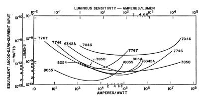
Fig. 45. "Equivalent anode dark current input" as a function of the luminous sensitivity for various multiplier phototubes. The Equivalent Anode Dark Current Input represents the light flux which would result in an output current change just equal to the dark current. Optimum operating range is usually where this function is near a minimum.
