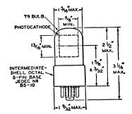
HEAD-ON type having S-1 response. Wavelength of maximum spectral response is  $8000 \pm 1000$  angstroms. This type makes use of a flat circular photocathode, and has a direct interelectrode capacitance of 1.8 picofarads. It weighs approximately 0.3 ounces.
