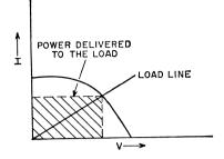
Fig. 84. Current-voltage characteristic of a photojunction device connected in the photovoltaic mode.
