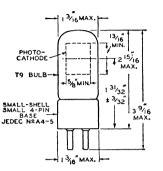
SIDE-ON, short-bulb type having S-1 response. Wavelength of maximum spectral response is  $8000 \pm 1000$ angstroms. This type makes use of a semicylindrical photocathode, and has a direct interelectrode capacitance of 1.6 picofarads. It weighs approximately 0.8 ounce.
