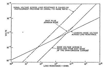
Fig. 23. Variation of signal voltage, Johnson-noise voltage, and shot-noise voltage developed across the load resistor by the dark emission—all as a function of the load resistor. Data are for a vacuum phototube having S-1 response, dark emission of 10 picoamperes, and temperature of 300° K, and for a bandwidth of 1 cycle.
