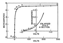
Fig. 20. Current-voltage characteristic for a typical vacuum phototube showing the various regions of interest.
