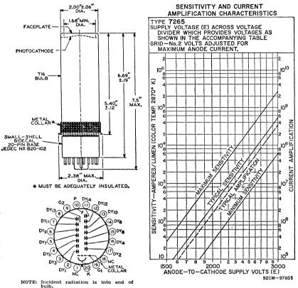
TEN-STAGE, head-on, flat-faceplate type having S-20 response. Wavelength of maximum response is 4200  $\pm$  500 angstroms. This type makes use of silver-magnesium dynodes and a curved-circular, potassium-bismuth-sodium-cesium, semitransparent photocathode. (This type may also be ordered with copper-beryllium dynodes.) Window material is Corning No. 0080 lime glass or equivalent. Tube weighs approximately 6 ounces and has a non-hygroscopic base.
