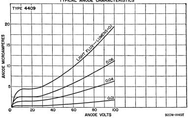
TEN-STAGE, ruggedized, flat-faceplate type having S-11 response. Wavelength of maximum response is  $4400 \pm 500$  angstroms. This type makes use of cesium-antimony dynodes and a flat-circular, cesiumantimony, semitransparent photocathode. Window material is Corning No. 0080 lime glass or equivalent. Tube weighs approximately 2 ounces.
