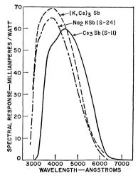
Fig. 40. Comparison of the absolute spectral sensitivities of three antimony alkali photocathodes: Cs\_Sb, Na\_KSb, and (K,CS)\_3Sb. The S-11 curve shown is representative of the cathode on type 8053: the S-24 and (K, Cs)\_3Sb curves are tentative.
