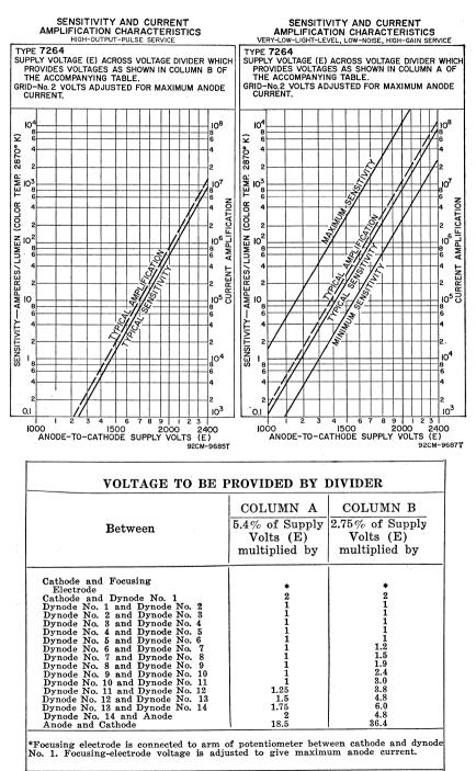
FOURTEEN-STAGE, head-on, flat-faceplate type having S-20 response. Wavelength of maximum spectral response is  $4200 \pm 500$  angstroms. This type makes use of copper-beryllium dynodes, and a curved-circular, semitransparent, antimony-potassium-sodium-cesium photocathode. Window material is Corning No. 0080 lime glass or equivalent. Tube weighs approximately 8 ounces and has a non-hygroscopic base.
