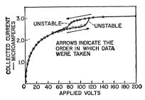
Fig. 16. Erratic current-voltage characteristic in a vacuum phototube caused by bulb charges which result when the anode is too small to collect all emitted photoelectrons.
