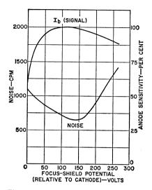
Fig. 48. Typical variation of noise output of a 6342A multiplier phototube as **a** function of focus-shield potential. Also indicated is the output signal current showing how only a minimum loss in signal sensitivity results from a choice of shield potential which minimizes noise.
