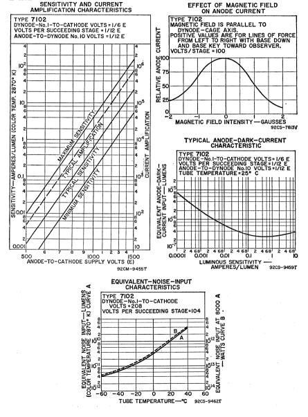
NINE-STAGE, side-on type having S-4 response. Wavelength of maximum response is  $4000 \pm 500$  angstroms. This type makes use of cesium-antimony dynodes and a cesium-antimony, opaque photocathode. Window material is Corning No. 0080 lime glass or equivalent. Tube weighs approximately 1.6 ounces. For outline and terminal-connection diagram, refer to type 6328.
