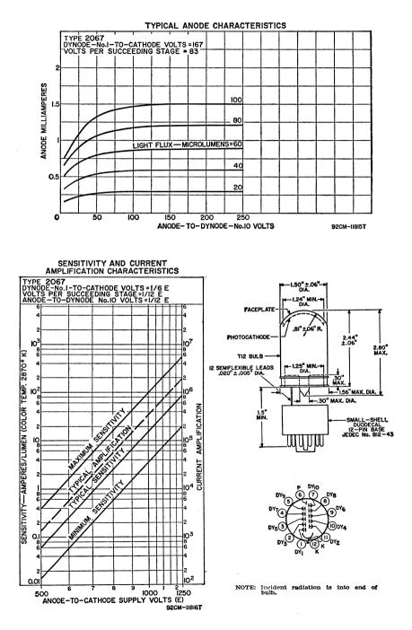
SIDE-ON type having unobstructed photocathode area and S-4 response. Wavelength of maximum spectral response is  $4000 \pm 500$  angstroms. This type makes use of a semicylindrical photocathode, and has a direct interelectrode capacitance of 2.4 picofarads. It weighs approximately 0.9 ounce. For outline and terminal-connection diagram, refer to type 1P40.
