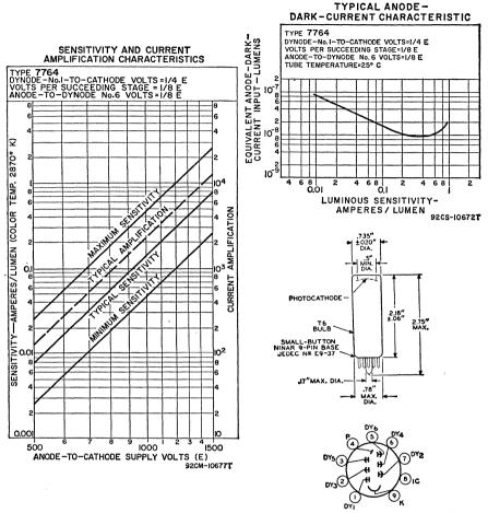
NOTE: Incident radiation is into end of bulb.
