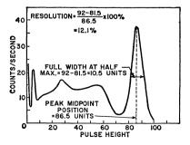
Fig. 52. Distribution of pulse heights observed in a scintillation counting experiment using gamma rays from Cs<sub>137</sub> to excite a NaI (T1) crystal.
