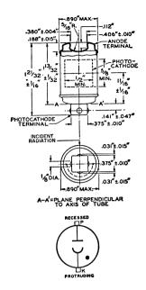
SIDE-ON type having S-4 response. Wavelength of maximum spectral response is  $4000 \pm 500$  angstroms. This type makes use of a semicylindrical photocathode, and has a direct interelectrode capacitance of 2 picofarads. It weighs approximately 0.3 ounce. For curves of typical anode characteristics, refer to type 5581. For outline and terminal-connection diagram, refer to type 927.
