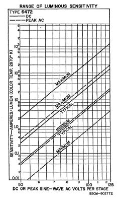
SIDE-ON type having S-1 response. Wavelength of maximum spectral response is  $8000 \pm 1000$  angstroms. This type makes use of a semicylindrical photocathode, and has a direct interelectrode capacitance of 3 picofarads. It weighs approximately 1.3 ounces and has a non-hygroscopic base.
