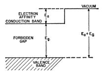
Fig. 5. Energy model of a semiconductor photoemitter.
