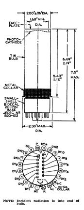
TEN-STAGE, head-on, flat-faceplate type having S-13 response. Wavelength of maximum response is 4400  $\pm$  500 angstroms. This type makes use of cesiumantimony dynodes and flat-circular, cesium-antimony, semitransparent photocathode. Window material is fused silica. Tube weighs approximately 5.8 ounces and has a non-hygroscopic base.
