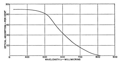
Fig. 38. Optical absorption of Cs<sub>3</sub>Sb layer having a typical S-11 spectral response.
