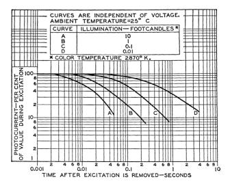
Fig. 75. Typical decay characteristics of a cadmium-sulfide cell.
