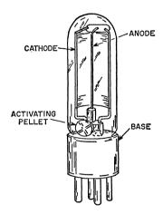
Fig. 17. Typical construction of a vacuum phototube.
