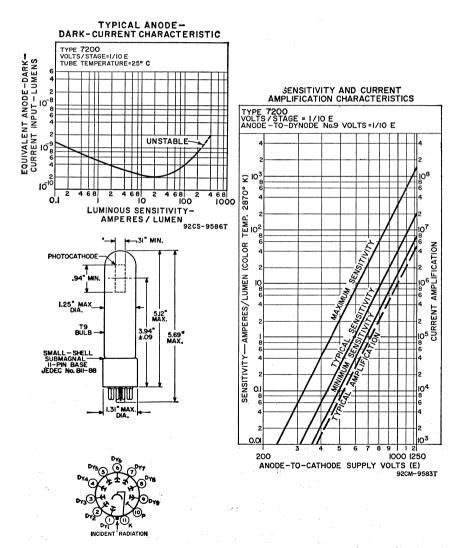
FOURTEEN-STAGE, head-on, spherical-faceplate type having S-11 response. Wavelength of maximum spectral response is  $4400 \pm 500$  angstroms. This type makes use of silver-magnesium dynodes and a spherical-circular, cesium-antimony, semitransparent photocathode. (This type may also be ordered with copper-beryllium dynodes.) Window material is Corning No. 0080 lime glass or equivalent. Tube weighs approximately 8 ounces and has a non-hygroscopic base.
