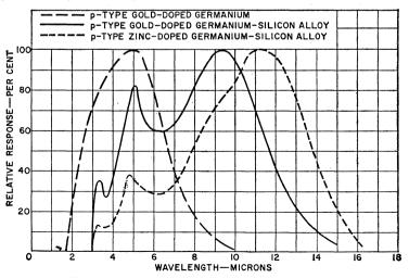
Fig. 87. Spectral response of infrared-sensitive detectors.
