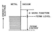
Fig. 1. Energy model for a metal showing the relationship of the work function and the Fermi level.
