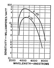
Fig. 39. Spectral response characteristics for S-10 (Bi-Ag-O-Cs photocathode) and S-20 [(Cs) Na<sub>2</sub> KSb photocathode].
