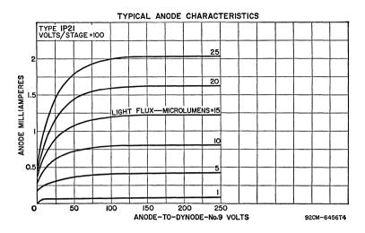
NINE-STAGE, side-on type having S-8 response. Wavelength of maximum response is  $3650 \pm 500$  angstroms. This type makes use of cesium-antimony dynodes and a cesium-bismuth, opaque photocathode. Window material is Corning No. 0080 lime glass or equivalent. Tube weighs approximately 1.6 ounces and has a non-hygroscopic base. For outline and terminal-connection diagram, refer to type 1P21.
