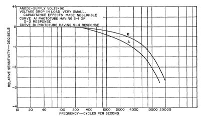
Fig. 28. Frequency response of gas-filled phototubes:
