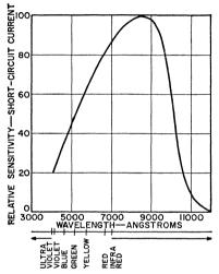
Fig. 86. Spectral response characteristic for a silicon solar cell.
