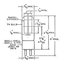
CARTRIDGE type having S-1 response. Wavelength of maximum spectral response is  $8000 \pm 1000$  angstroms. This type makes use of a semicylindrical photocathode, and has a direct interelectrode capacitance of 1 picofarad. It weighs approximately 0.4 ounce. For curves of typical anode characteristics, refer to type 930.
