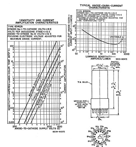
NOTE: Incident radiation is into end of bulb.
