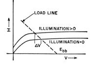
Fig. 82. Analysis of a photojunction device in the photoconductive mode of operation.
