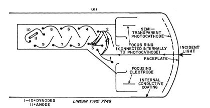
Fig. 32. Various dynode configurations in general use: (A) circular-cage type. (B) and (C) linear types.
