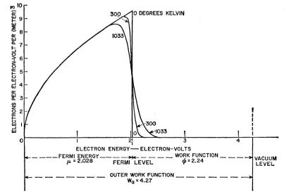
Fig. 2. Energy distribution of conduction electrons in potassium at temperatures of 0, 300, and 1033 degrees Kelvin based on elementary Sommerfeld theory. (ref. 17)
