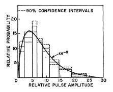
Fig. 51. Measured amplitude distribution of anode pulses due to single photo-electron inputs for a 2-inch diameter, 14-stage multiplier phototube having C<sub>83</sub>Sb dynodes. Gain per stage is approximately 3.
