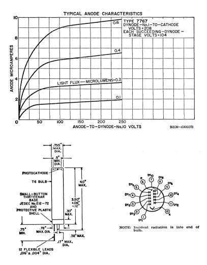
7850 MULTIPLIER PHOTOTUBE TWELVE-STAGE, head-on, spherical-faceplate type having S-11 response. Wavelength of maximum response is  $4400 \pm 500$  angstroms. This type makes use of copper-beryllium dynodes and a sphericalcircular, cesium-antimony, semitransparent photocathode. Window material is Corning No. 0080 lime glass or equivalent. Tube weighs approximately 7 ounces and has a non-hygroscopic base.
