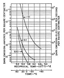
Fig. 46. Temperature variation of dark current for multiplier phototubes in the manner of a Richardson plot.
