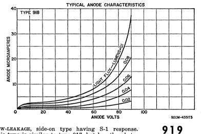
LOW-LEAKAGE, side-on type having S-1 response. This type is similar to type 917, but has the photocathode rather than the anode connected to the top cap.
