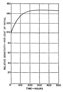
Fig. 67. Typical sensitivity variation on life for a 6342A multiplier phototube (silver magnesium dynodes) operating with 1250-volt anode supply voltage for a period of 500 hours. Initial anode current is 2 milliamperes and is readjusted to this operating value at 48, 168 and 360 hours.
