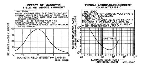
TEN-STAGE, ruggedized, head-on type having S-11 response. Wavelength of maximum response is 4400  $\pm$  500 angstroms. This type makes use of cesiumantimony dynodes and a cesium-antimony, semitransparent photocathode having a circular hemispherical shape. Window material is Corning No. 0080 lime glass or equivalent. Tube weighs approximately 1.8 ounces without base.
