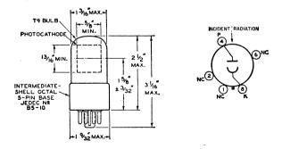
1 P 4 0 GAS PHOTODIODE SIDE-ON type having S-1 response. This type is similar to type 930, but has a maximum anode dark current at  $25^{\circ}$ C of 0.005 microampere at 90 volts, and makes use of a non-hygroscopic base for increased resistance between anode and photocathode pins under adverse conditions of high humidity. INCIDENT ' RADIATION
