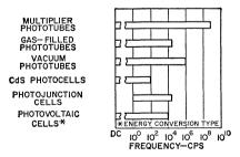
Fig. 91. Range of frequency response of various photodetectors. Recommendation of operation for dc (unmodulated light) sources is indicated by the symbol dc at the left end of the frequency range.
