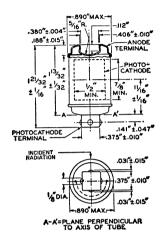
SIDE-ON type having S-1 response. Wavelength of maximum spectral response is  $8000 \pm 1000$  angstroms. This type makes use of a semicylindrical photocathode, and has a direct interelectrode capacitance of 2 picofarads. It weighs approximately 0.3 ounce.
