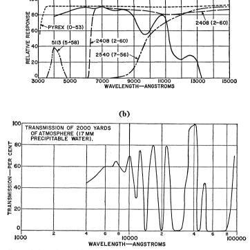
Fig. 90. Transmission characteristics of various useful color filters, glasses, and the atmosphere. ( (A) 2540, 5113, 2408, Pyrex (B) 2000 yds of air.)
