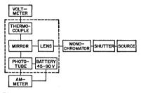
Fig. 93. Typical system for determining spectral-sensitivity characteristics of phototubes.
