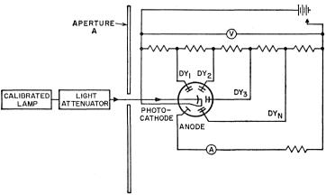
Fig. 95. Typical circuit for measuring sensitivity of multiplier phototubes.
