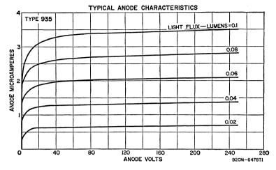
TEN-STAGE, head-on, flat-faceplate type having S-11 response. Wavelength of maximum response is 4400  $\pm$  500 angstroms. This type makes use of copper-beryllium dynodes and a cesium-antimony, semitransparent photocathode having a high-conductivity grating. Window material is Corning No. 0080 lime glass or equivalent. Tube weighs approximately 5.2 ounces and has a non-hygroscopic base.
