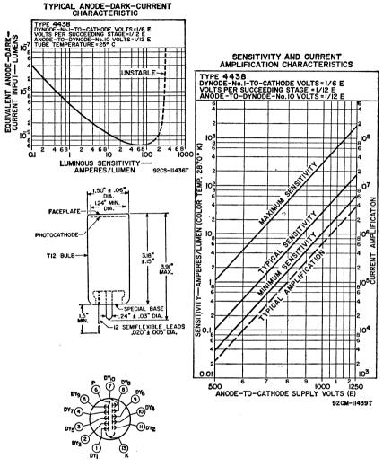
NOTE: Incident radiation is into end of bulb.
