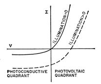
Fig. 81. Current-voltage characteristic for a photojunction device.
