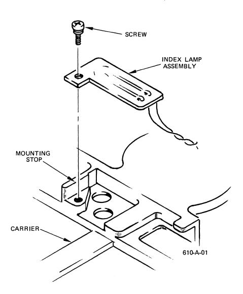
Figure 26. Index Lamp Assembly Removal and Installation
