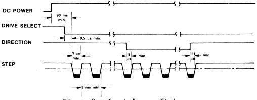
Figure 9. Track Access Timing
