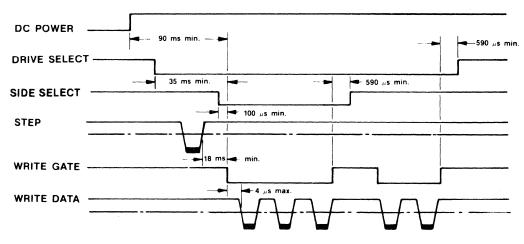
Figure 11. Write Timing
