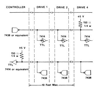
Figure 1. Recommended Controller Interface Circuit
