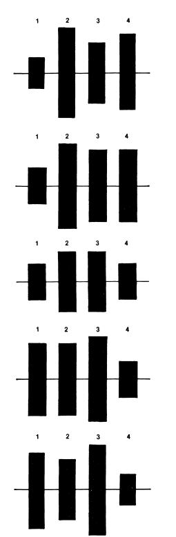
MAXIMUM ALLOWABLE AZIMUTH ERROR OF + 18 MINUTES. BURST #4 IS 25% LARGER IN AMPLITUDE THAN BURST #3.
