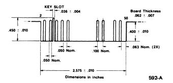
Figure 13. Connector J1 Dimensions (component side)
