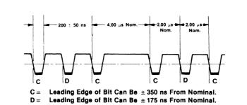
Figure 8. Read Data Timing for Modified Frequency Modulation (MFM)
