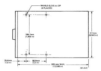
Figure 14. QumeTrak 242 (Top View)
