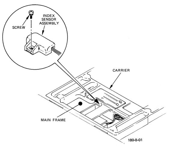
Figure 27. Index Sensor Assembly Removal and Installation
