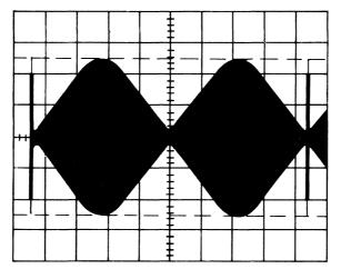
EQUAL AMPLITUDE (EXACTLY ON TRACK 40)
