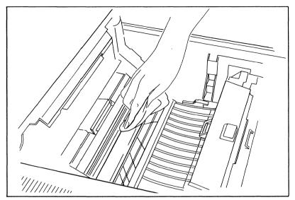
Fig. 8.9. Cleaning the transfer guide and paper lock.
