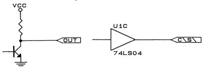
Figure 6-10 Connecting Signals to Module Ports
