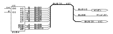
Figure 6-13. Connecting Labels to Module Ports
