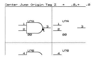
Figure 7-5. The Completed NAND Gate Body
