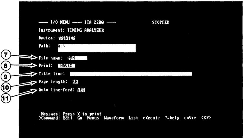
■ Figure 5-25. The I/O Menu with PRINTER as the selected device.
