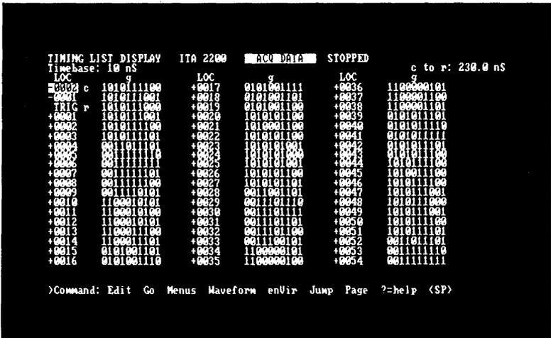
■ Figure 5-23. Example of the compressed display format.
