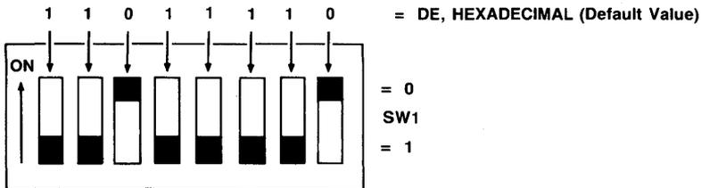
**Figure 2-6. Address switches on the PC interface board.**
