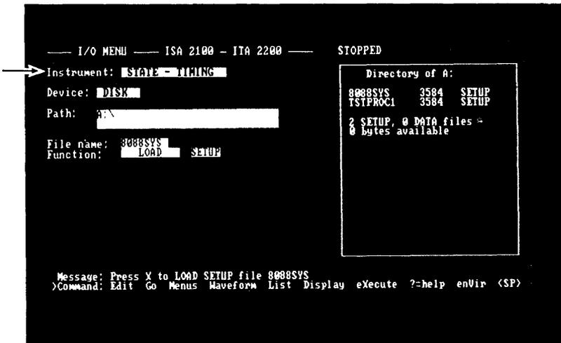
■ Figure 6-4. The I/O Menu when the state and timing non-aligned mode is selected.
