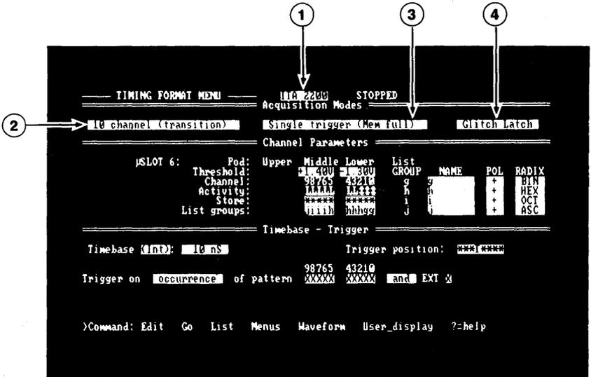
■ **Figure 5-5. The Format Menu and its fields for controlling the analyzer's acquisition modes.**
