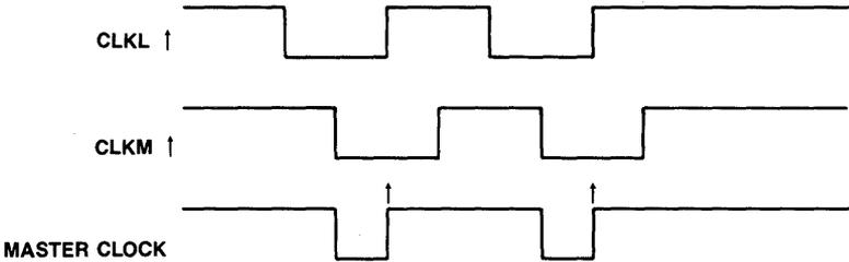
■ **Figure 4-1. Using the lower and middle probe clocks in an ORed condition.**
