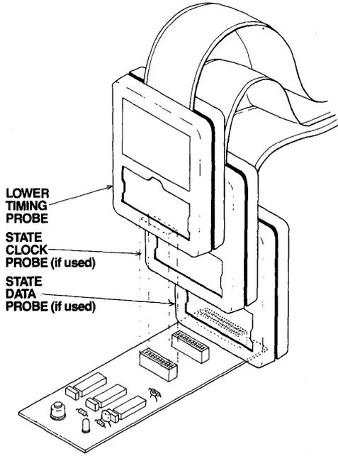
■ Figure 7-2. Connecting the probes.
