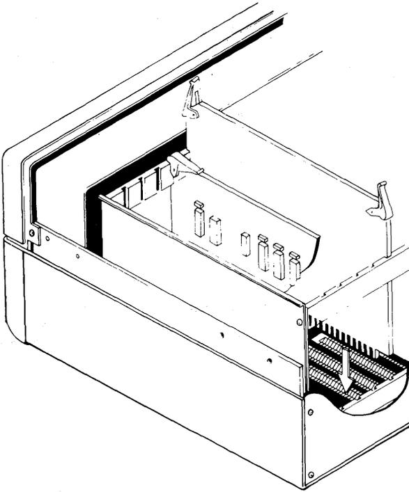
■ **Figure 2-12. Installing a circuit board into the  $\mu$ Analyst mainframe.**
