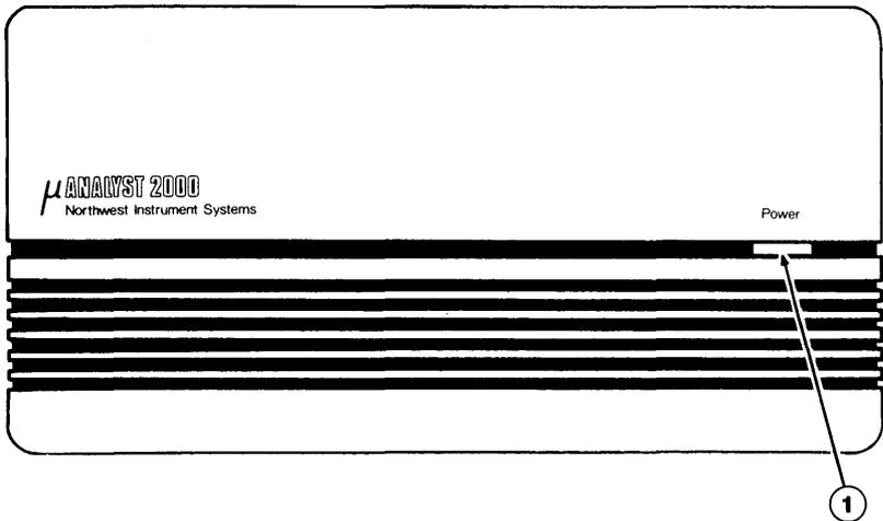
**Figure 2-1. The front panel of the  $\mu$ Analyst mainframe.**
