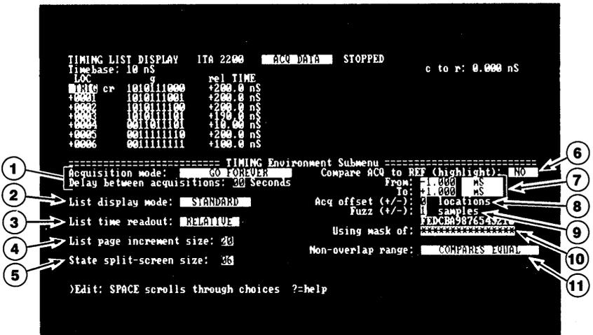
**Figure 5-22. The Environment Submenu and its fields.**
