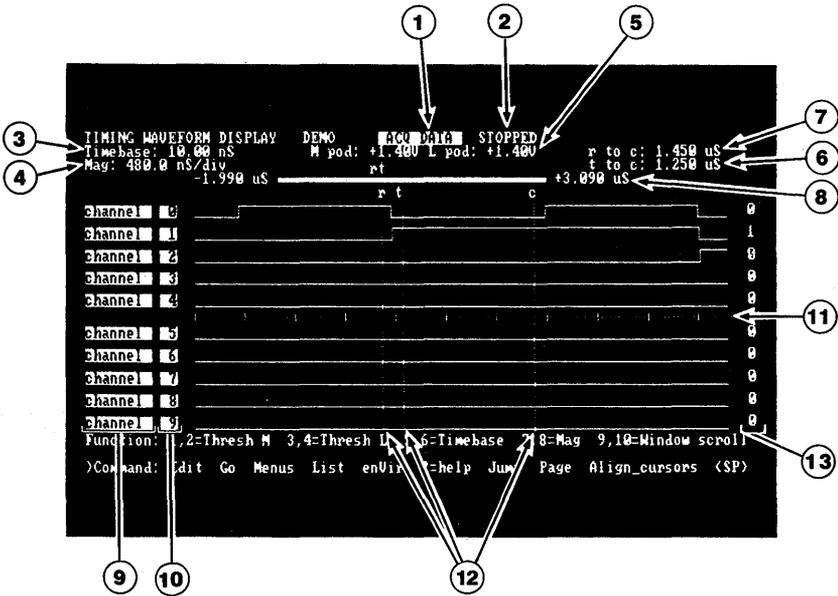
■ Figure 5-13. The Waveform Display Menu and its fields.
