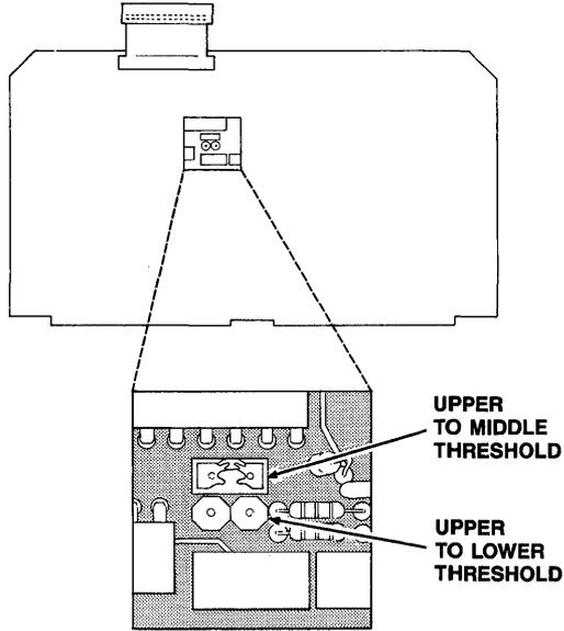
■ **Figure 2-10. Setting the upper probe's threshold jumper.**
