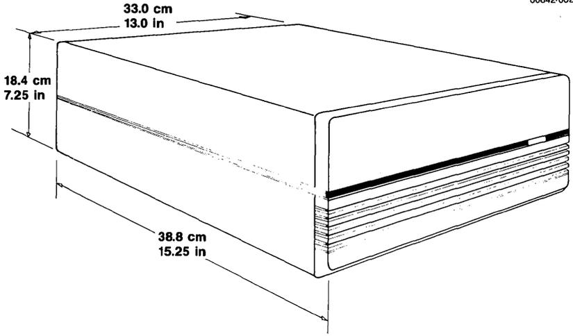
■ Figure 1-2. Dimensions of the  $\mu$ Analyst 2000 Mainframe.
