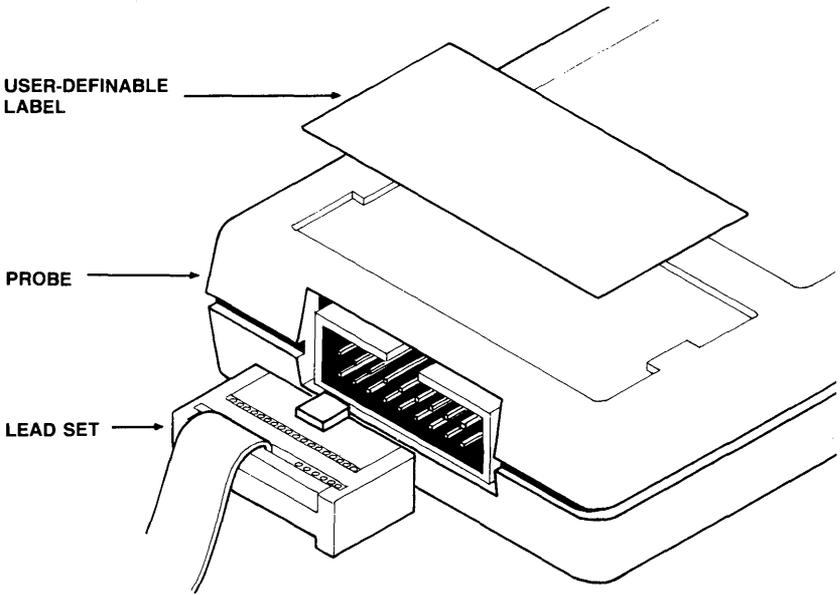
■ Figure 2-14. Installing a lead set on a probe.
