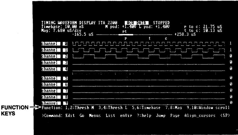
■ Figure 5-14. Function keys in the Waveform Display Menu.
