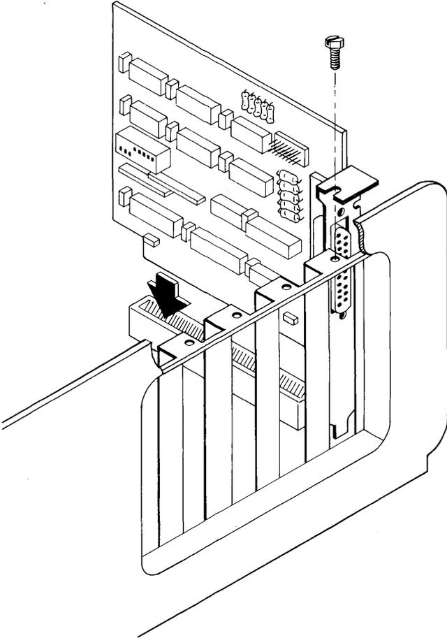
■ Figure 2-7. Installing the PC interface board.
