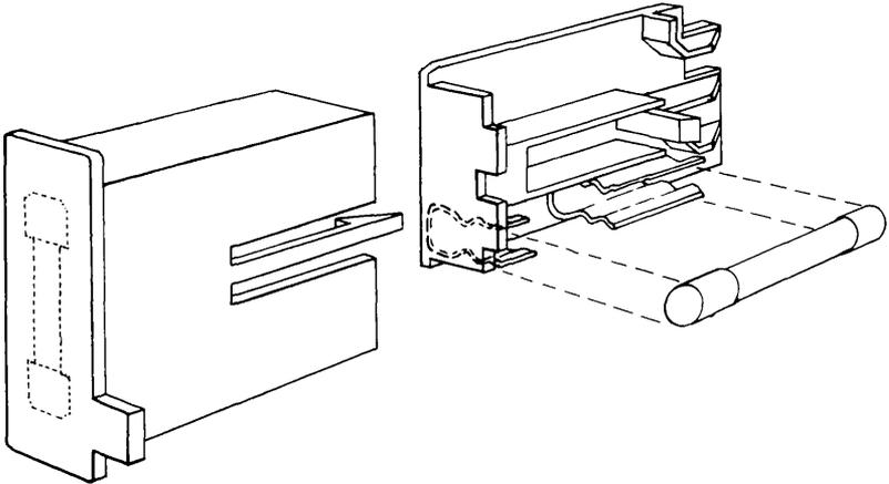
■ Figure 2-4. Detaching the fuse-holder circuit board.
