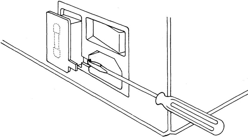
■ Figure 2-3. Removing the fuse holder.
