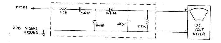
Figure 1C: A.C. SIGNAL DETECTOR
