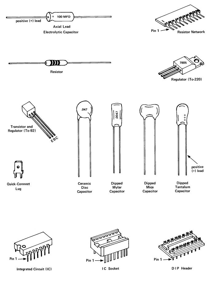
Figure 1A. Identification and orientation of components.
