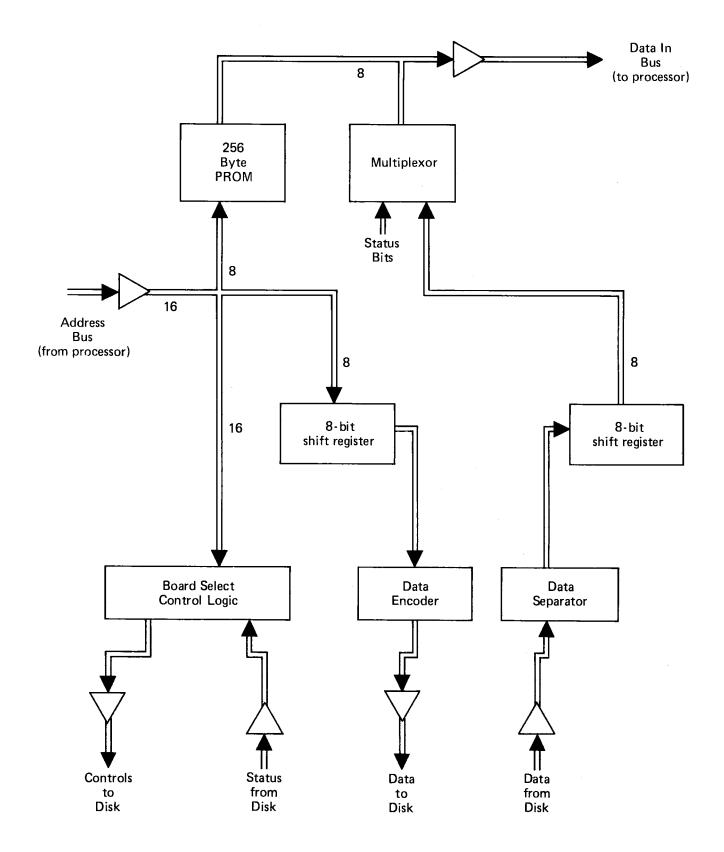
Figure 1T. Disk Controller Block Diagram
