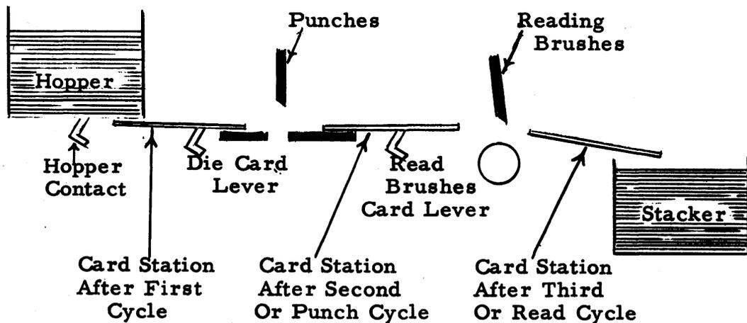
As can be seen from the diagram, one card must be fed into the computer to the First Card Station before punching can begin, and two cards must be fed before reading starts. As a new card is fed, the cards already in the Summary Punch advance to the next station. The Summary Punches used with the CRC 102-A will do only one operation, either read or punch. Two machines must be used to have both operations.
