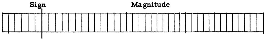
The first four binary digits in the sign are always zero. The fifth digit of the sign indicates the algebraic sign of the magnitude. When it is zero, the number is positive or absolute; when it is one, the number is negative. The sixth binary digit of the sign is an overflow marker. When it is zero, it indicates no overflow; when it is one, it indicates overflow. It may be filled initially, with the magnitude, as a special marker
