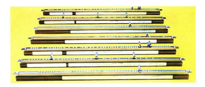
**REMOVABLE PROGRAM BARS.** Each readily altered to meet changing requirements. Easily exchanged while sitting in normal posting position. Provides flexibility in design of forms. Permits a wide variety of applications being placed on the same machine and full utilization of machine time.
