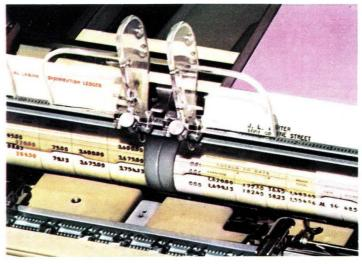
VISIBLE PROGRAM INDEX. An integral part of each program bar. Permits instant verification of proper program selection and the positioning of forms to receive entries. Safeguards against improper entries being made to accounting records. Indicates the type of entry and where each entry should be made. Simplifies operator training . . . Encourages accuracy and greater speed of posting.
