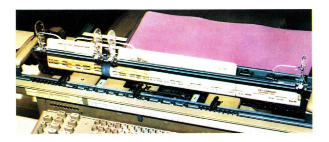
**COMPLETE VISIBILITY.** Visibility of previous and present postings—plus front feed form insertion—encourages accuracy. The ability to sight-audit all entries and balances picked-up prevents high postings, insures correct form alignment and simplifies posting procedure.
