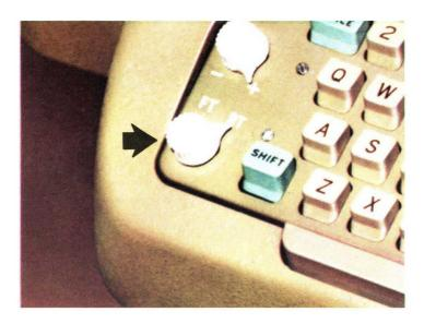
split and NORMAL PLATEN. Platens are available which operate in either "split" or "normal" position—either independently or as one unit. When "split"... by merely pulling outward on the platen control knob... independent controls over vertical spacing and carriage opening are provided automatically for each side. When "normal," both sides of the platen operate together as a single unit.
