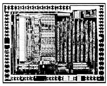
Standard Cell Microcomputer with Core Microprocessor, Sound Generator, I/O and Random Cell Logic.
