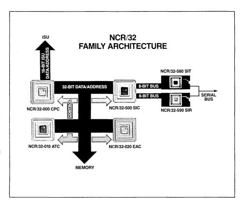
The NCR/32 VLSI Processor family consists of the Central Processor Chip (CPC), the Address Translation Chip (ATC), and the System Interface Controller (SIC). Additional members of the family include the Extended Arithmetic Chip (EAC), the System Interface Transmitter (SIT) and Receiver (SIR) chips, and the Bus Assist Chip (BAC).
