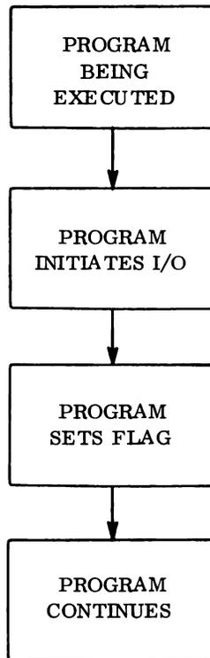
Figure 6-2. Interrupt Input/Output Initiation
