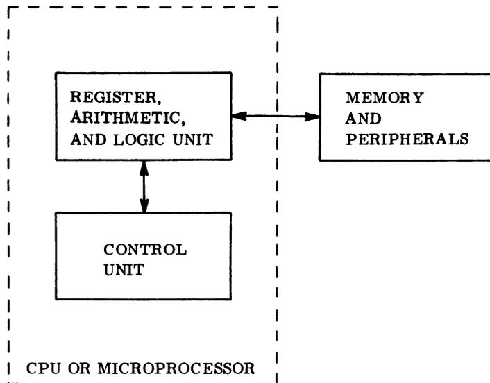
Figure 2-1. Major Components of a Microcomputer
