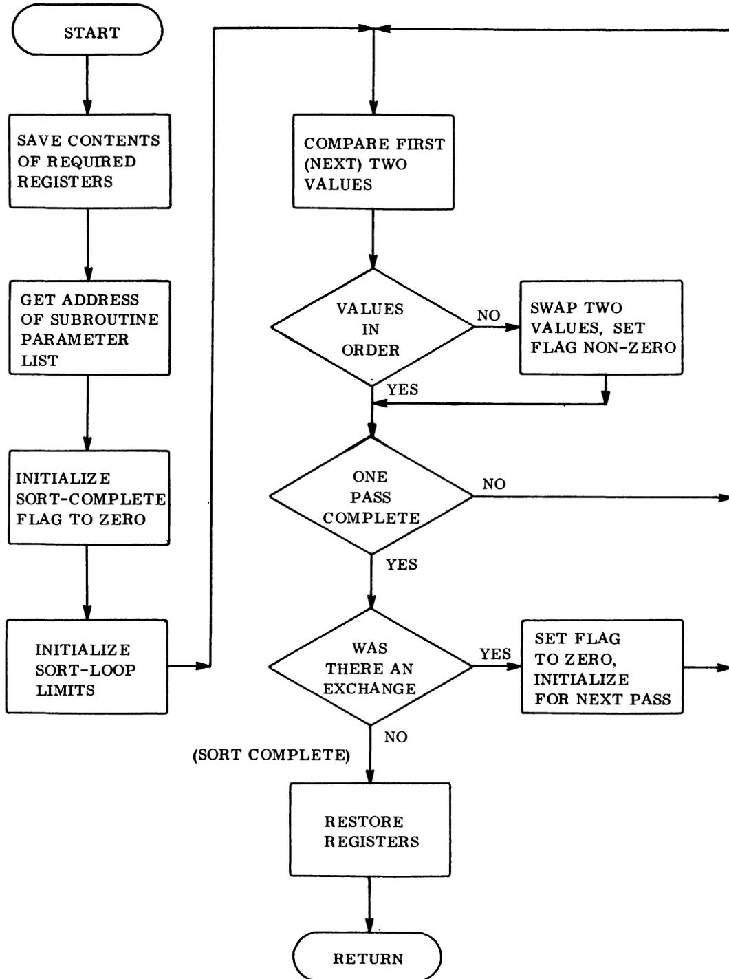
Figure 2-2. Flowchart for Simple Sort Routine
