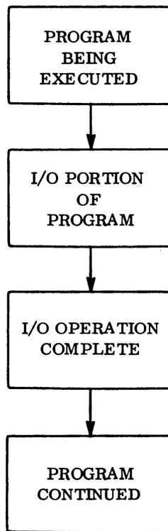
Figure 6-1. Programmed Input/Output
