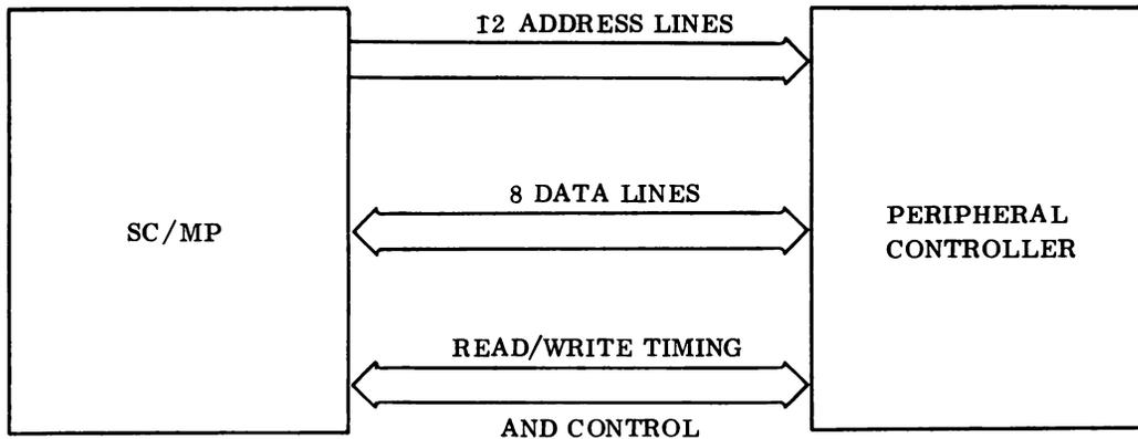
Figure 3-3. Interface to Peripheral Device Controller
