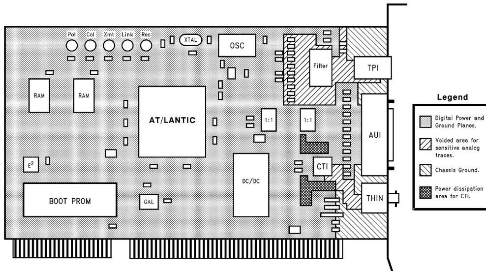
FIGURE 2. DP83905EB-AT Board Layout and Component Placement
