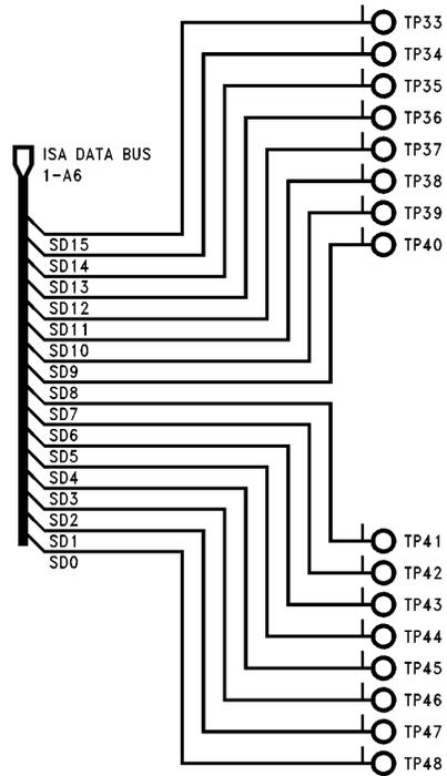
NOTE: These Test Points are for In-Circuit bed-of-nails testing. They will be VIAs on the PCB.
