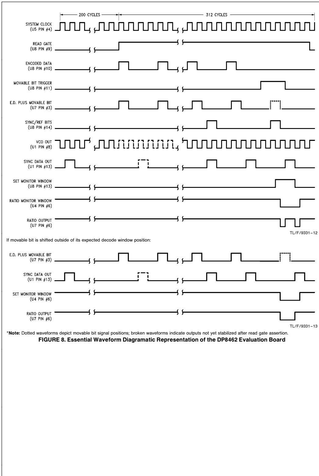
**FIGURE 8. Essential Waveform Diagrammatic Representation of the DP8462 Evaluation Board**
