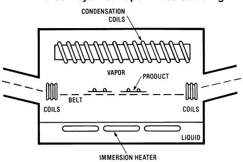
The question of thermal shock is asked frequently because of the relatively sharp increase in component temperature from room temperature to 215°C. SO packages mounted on representative boards have been tested and have shown little effect on the integrity of the packages. Various packages, such as cerdips, metal cans and TO-5 cans with glass seals, have also been tested.
