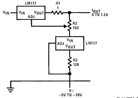
FIGURE 7. Adjustable Current Regulator
