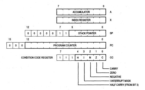
Figure 2-2. M68HC05 CPU Registers
