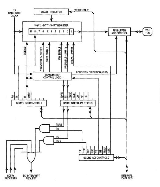
Figure 3-15. SCI Transmitter Block Diagram
