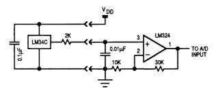
Figure 4-2. Precision Temperature Sensing Circuit
