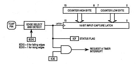
Figure 3-39. Input-Capture Operation
