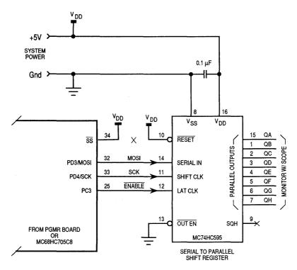
Figure 3-34. SPI Application Example Diagram
