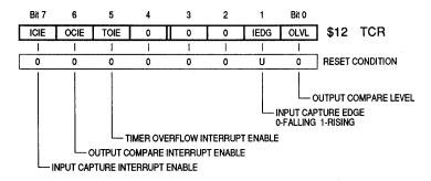
Figure 3-41. Timer Control Register
