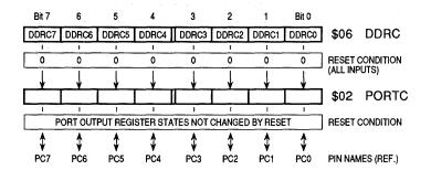
Figure 3-12. Port C and Data Direction C Registers
