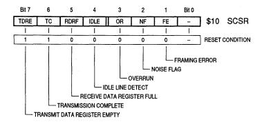
Figure 3-21. Serial Comunications Status Register
