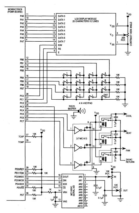
Figure 4-1. Thermostat Project Schematic Diagram
