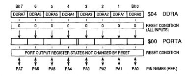
Figure 3-10. Port A and Data Direction A Registers
