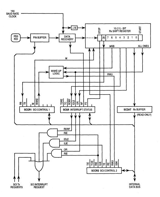
Figure 3-16. SCI Receiver Block Diagram
