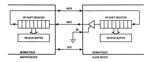
Figure 3-29. Shift Register Operation
