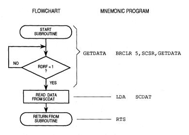
Figure 3-26. SCI Normal Receive Operation Flowchart
