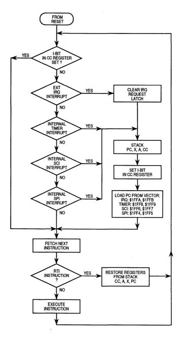
Figure 3-8. Hardware Interrupt Flowchart
