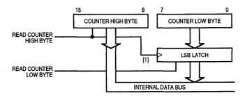
LSB latch is normally transparent, becomes latched when high byte of counter is read, and becomes transparent again when low byte of counter is read.
