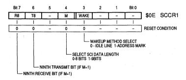
Figure 3-19. Serial Communications Control Register One
