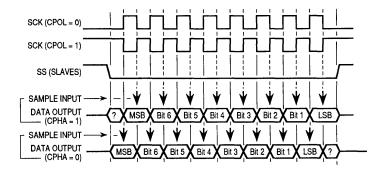
Figure 3-30. Data/Clock Timing Diagram
