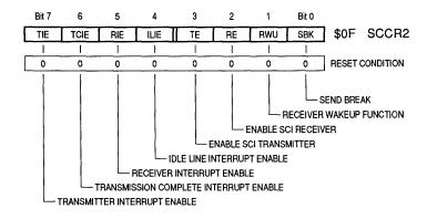
Figure 3-20. Serial Communications Control Register Two
