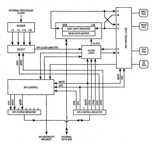
Figure 3-28. SPI Block Diagram
