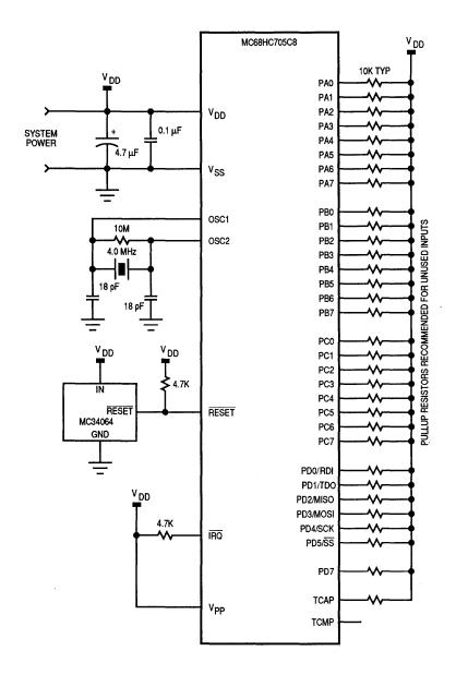
Figure 3-4. Typical Basic Connections
