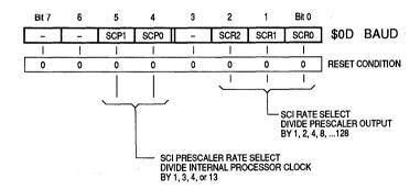
Figure 3-17. Baud Rate Register
