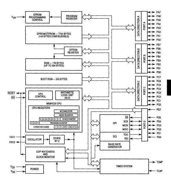
Figure 3-1. MC68HC705C8 Microcontroller Block Diagram
