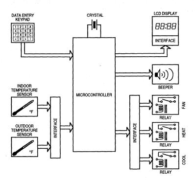
Figure 1-3. Thermostat Project Block Diagram
