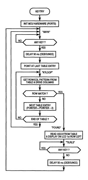
Figure 4-9. Keypad Checkout Flowchart
