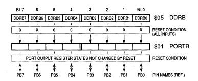
Figure 3-11. Port B and Data Direction B Registers
