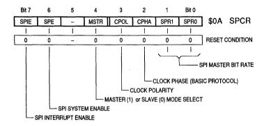
Figure 3-31. Serial Peripheral Control Register
