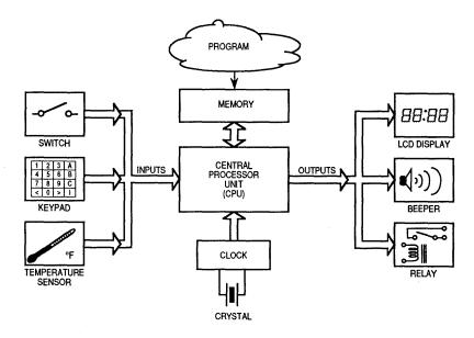
Figure 1-1. A Typical Computer System
