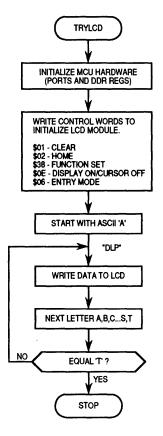
Figure 4-7. Display Checkout Flowchart
