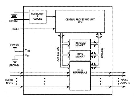
Figure 2-1. MCU Expanded Block Diagram
