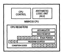
Figure 3-6. M68HC05 CPU Block Diagram
