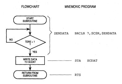
Figure 3-25. SCI Normal Transmit Operation Flowchart
