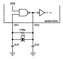
(a) Crystal/Ceramic Resonator Oscillator Connections
