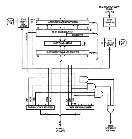
Figure 3-37. Programmable Timer Block Diagram
