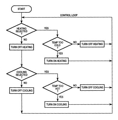
Figure 1-2. A Temperature Control Flowchart
