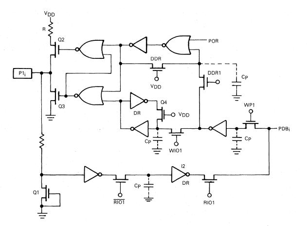
Figure 3-10. Logic Diagram for Port 1
