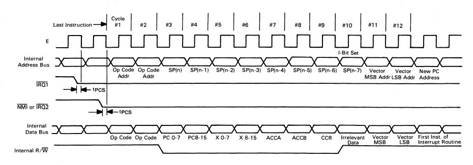
Figure 5-12. MC6801 Interrupt Sequence
