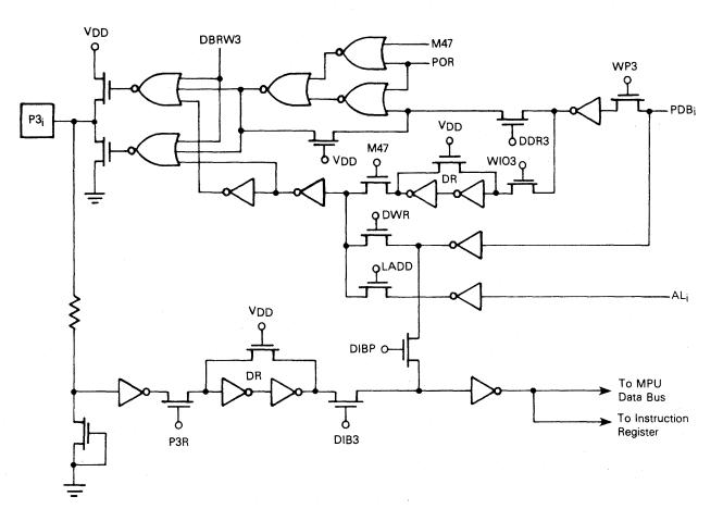
Figure 3-21. Logic Diagram for Port 3 (Repeated)
