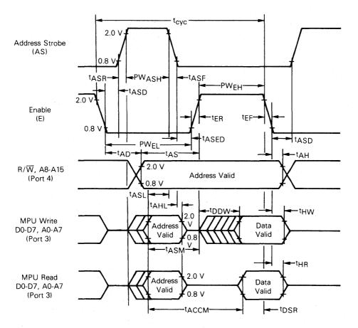
Figure 8-1. Expanded Multiplexed Bus Timing (Repeated)
