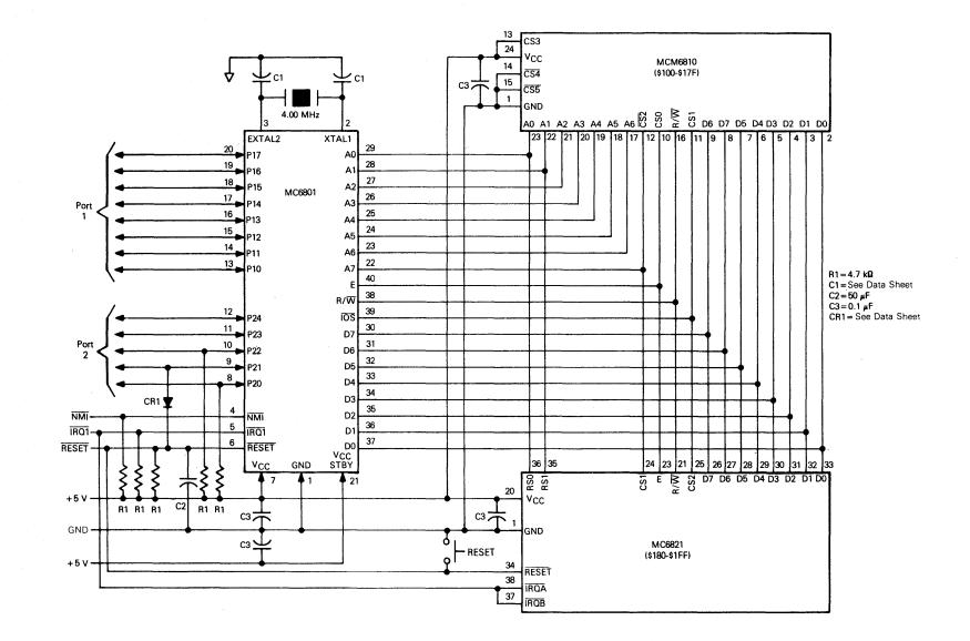
Figure 3-24. Typical Expanded Non-Multiplexed System
