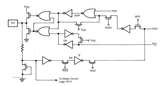
Figure 3-13. Logic Diagram for Port 2 Bit 1
