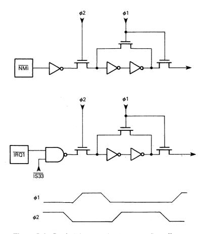
Figure 5-6. Logic Diagrams for Interrupt Sampling
