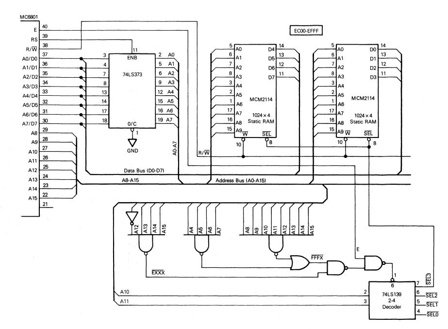
Figure 8-3. Expanded Multiplexed Bus Interface With MCM2114
