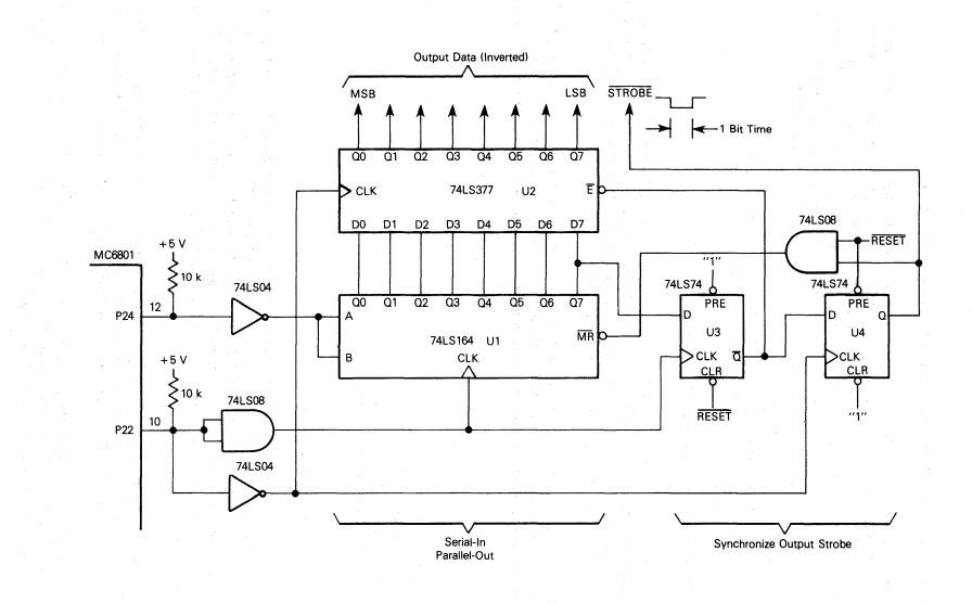
Figure 8-22. SCI Serial-to-Parallel Interface
