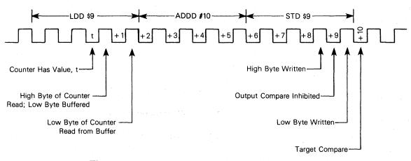
Figure 7-11. Immediate Output Compare Timing
