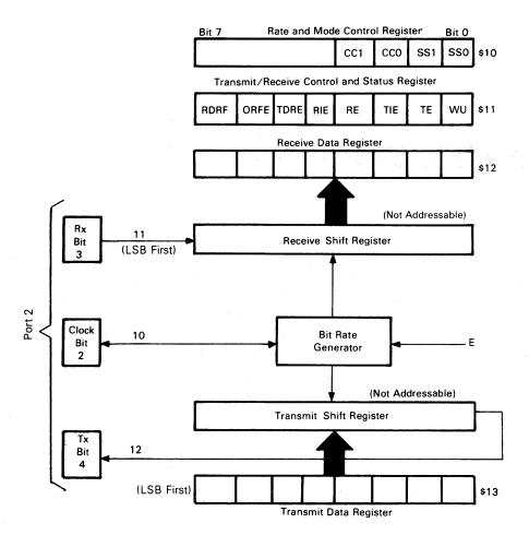
Figure 6-1. Serial Communications Interface Registers
