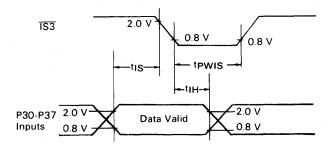
Figure 3-17. Port 3 Latch Setup and Hold Times
