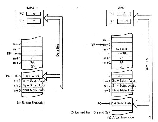
Figure 4-14. Operation of JSR (Extended) Instruction
