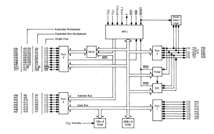
Figure 3-2. MC6801 Block Diagram
