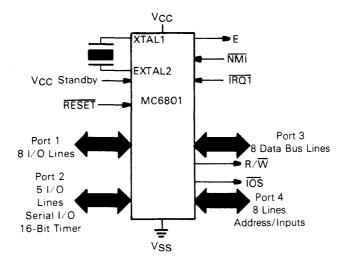
Figure 1-4. Expanded Non-Multiplexed Mode
