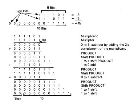
Figure 4-29. Multiplication Using Booth's Algorithm
