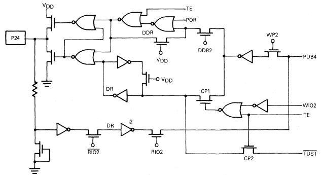
Figure 3-16. Logic Diagram for Port 2 Bit 4
