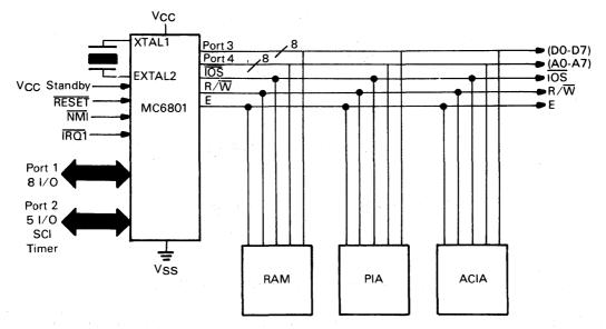
Figure 2-4. System Configuration — Expanded Non-Multiplexed Mode
