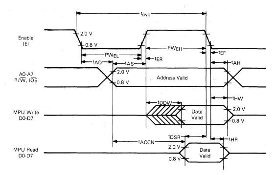
Figure 8-13. Expanded Non-Multiplexed Bus Timing (Repeated)
