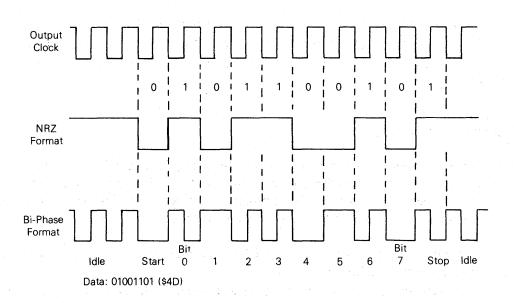
Figure 6-7. SCI Serial Data Formats
