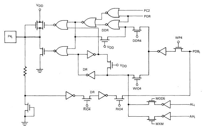
Figure 3-27. Logic Diagram for Port 4 (Repeated)
