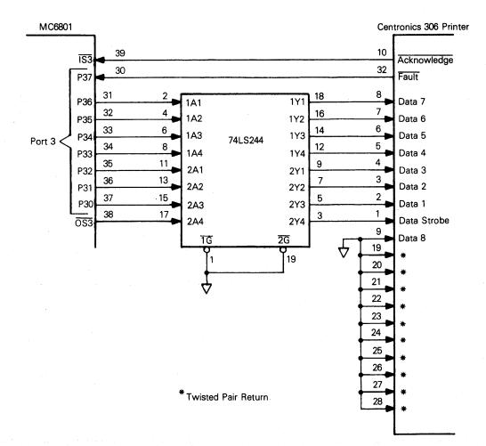
Figure 8-4. Line Printer Interface Connection Diagram
