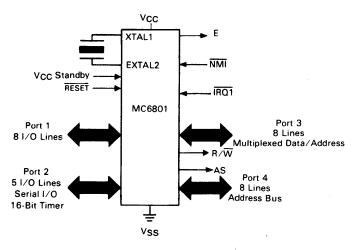
Figure 2-5. Expanded Multiplexed Mode
