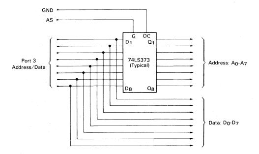
Figure 3-29. Typical Bus De-Multiplexing Latch Arrangement
