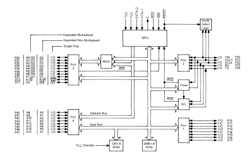
Figure 1-1. MC6801 Single Chip Microcomputer
