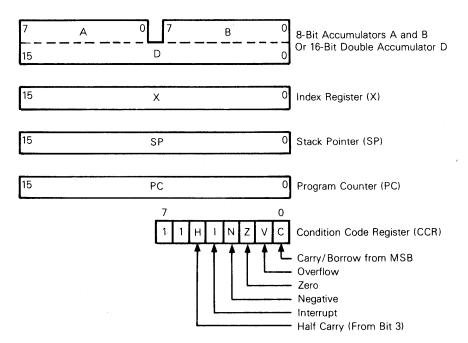
Figure 1-2. MC6801 Programming Model
