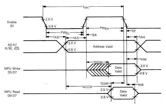
Figure 3-23. Expanded Non-Multiplexed Bus Timing
