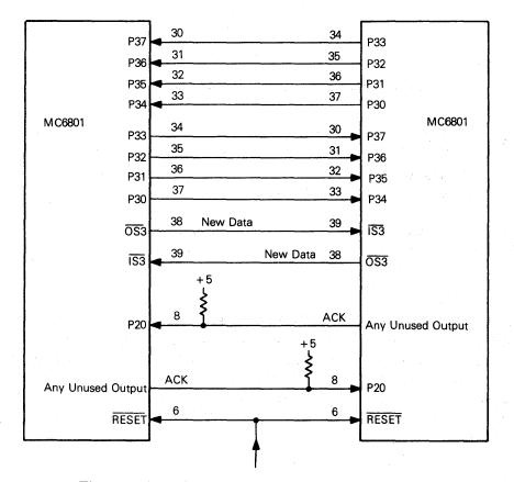
Figure 8-27. Interface Using Input Capture Function
