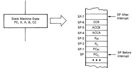
Figure 5-11. Stacking the Machine State
