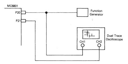
Figure 7-12. Equipment Arrangement for Program ECHO
