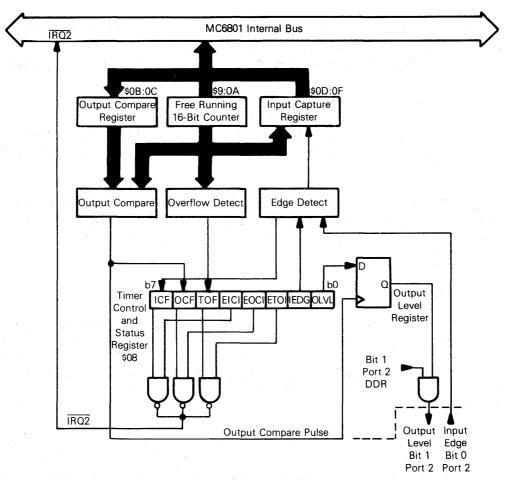
Figure 7-2. Block Diagram of Programmable Timer
