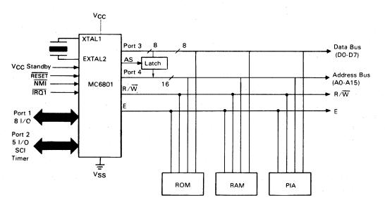
Figure 2-6. System Configuration for Expanded Multiplexed Modes
