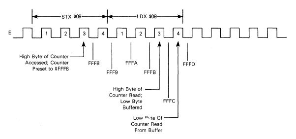
Figure 7-6. Counter Register Write and Read Diagram
