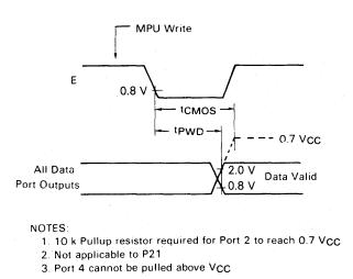
Figure 3-9. Data Port Timing for MPU Write
