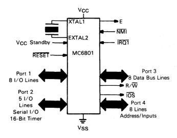
Figure 2-3. Expanded Non-Multiplexed Mode
