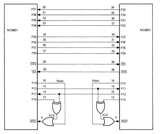
Figure 8-29. Interface Using Exclusive-OR Function
