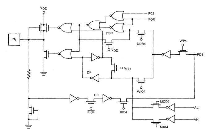
Figure 3-20. Logic Diagram for Port 4
