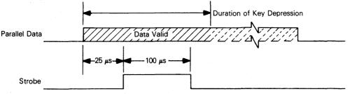
Figure 8-7. Keyboard Interface Signals
