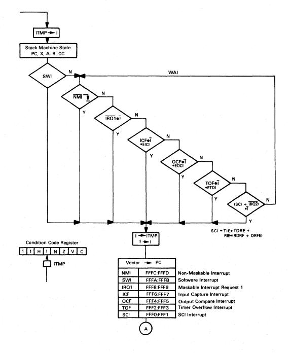
Figure 5-10. MC6801 Interrupt Flowchart
