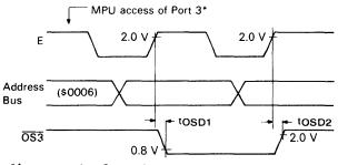
\*Access matches Output Strobe Select (OSS = 0, a read; OSS = 1, a write)
