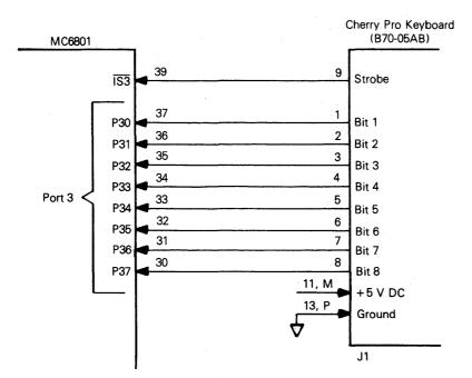
Figure 8-8. Keyboard Interface Connection Diagram
