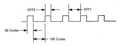
Figure 7-7. WAVGEN Default Output Signal
