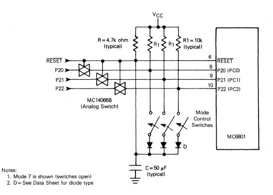
Figure 3-7. Programming the Mode with Analog Switches and Diodes
