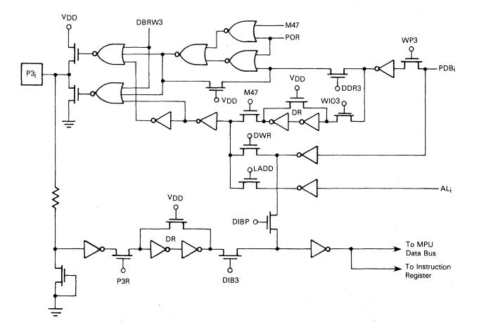
Figure 3-26. Logic Diagram for Port 3 (Repeated)
