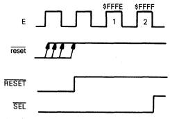
Figure J-1. Schematic for Mode 0 Reset Vector Chip Select Circuit
