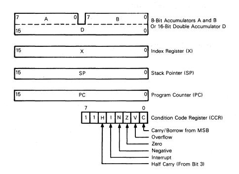
Figure 4-1. MC6801 MPU Programming Model
