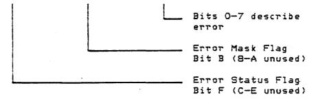
Normally, after the completion of each command, all bits of the Error Status and the Error Type are cleared (= 0). The Error Mask is not affected by MDOS commands. If an error occurred during the command, the Error Status Flag (bit F) will be set by the command. In addition, an Error Type will be set into the lower half of the status word (bits O-7). The Error Type is used to indicate which error was detected by the command.
