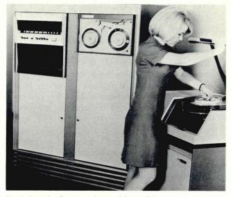
Fig. 4 Central collection and control key-to-disk-to-tape system. (Logic Corp. LC-720.)
