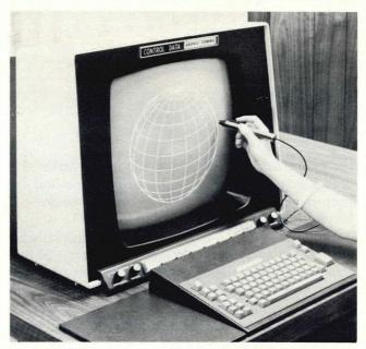
Fig. 1 Light pen in use with Control Data GRID Display
