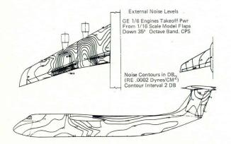
Fig. 9 Jet Aircraft Noise Contour (Courtesy of Electronics Associates Inc.)
