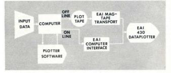
Fig. 1 System Configuration of Electronics Associates Inc. Model 430 Data Plotter
