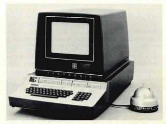
Fig. 2 Tektronic Trackball with T-4002 Terminal
