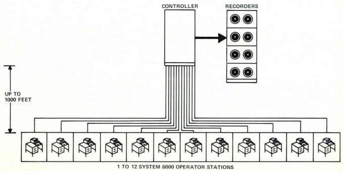
Fig. 5 Central collection and control multiple recorder system. (Sanders System 6000.)
