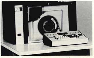
Fig. 2 Free-standing keyboard-to-computer-compatible magnetic tape keystation. (Mohawk Data Systems Model 6401.)
