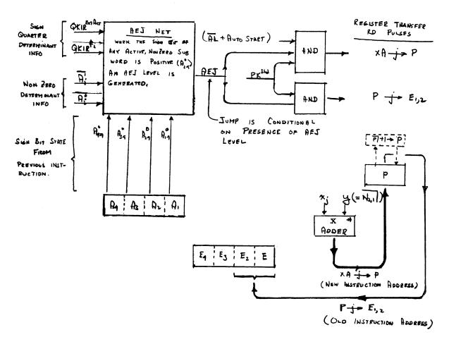
THE OUTPUT OF THE X ADDER (XA) EQUALS THE ARITHMETIC SUM OF X AND Y )
